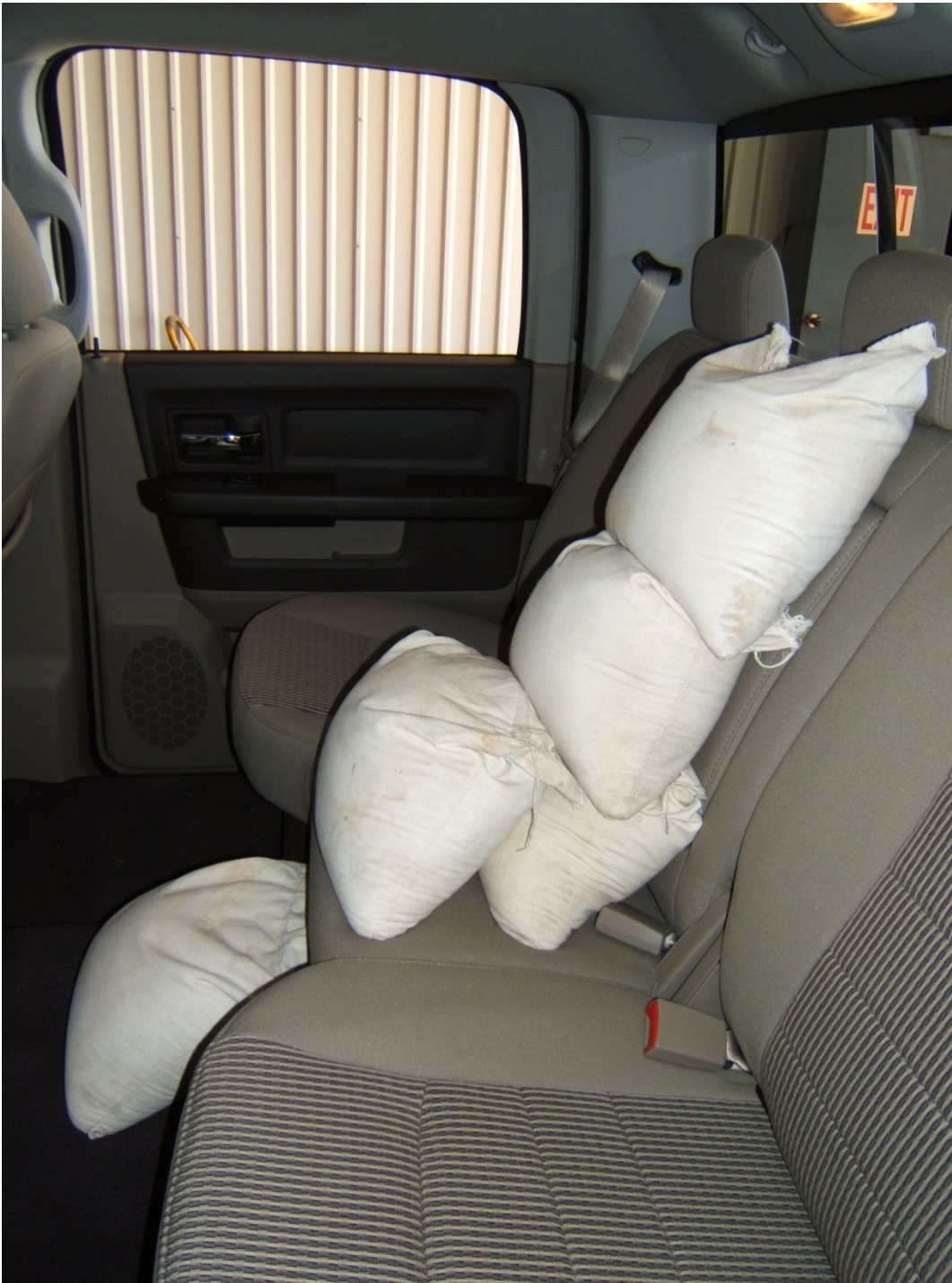
FIGURE 5.14 VEHICLE REAR SEAT BALLASTED FOR NORMAL LOAD
