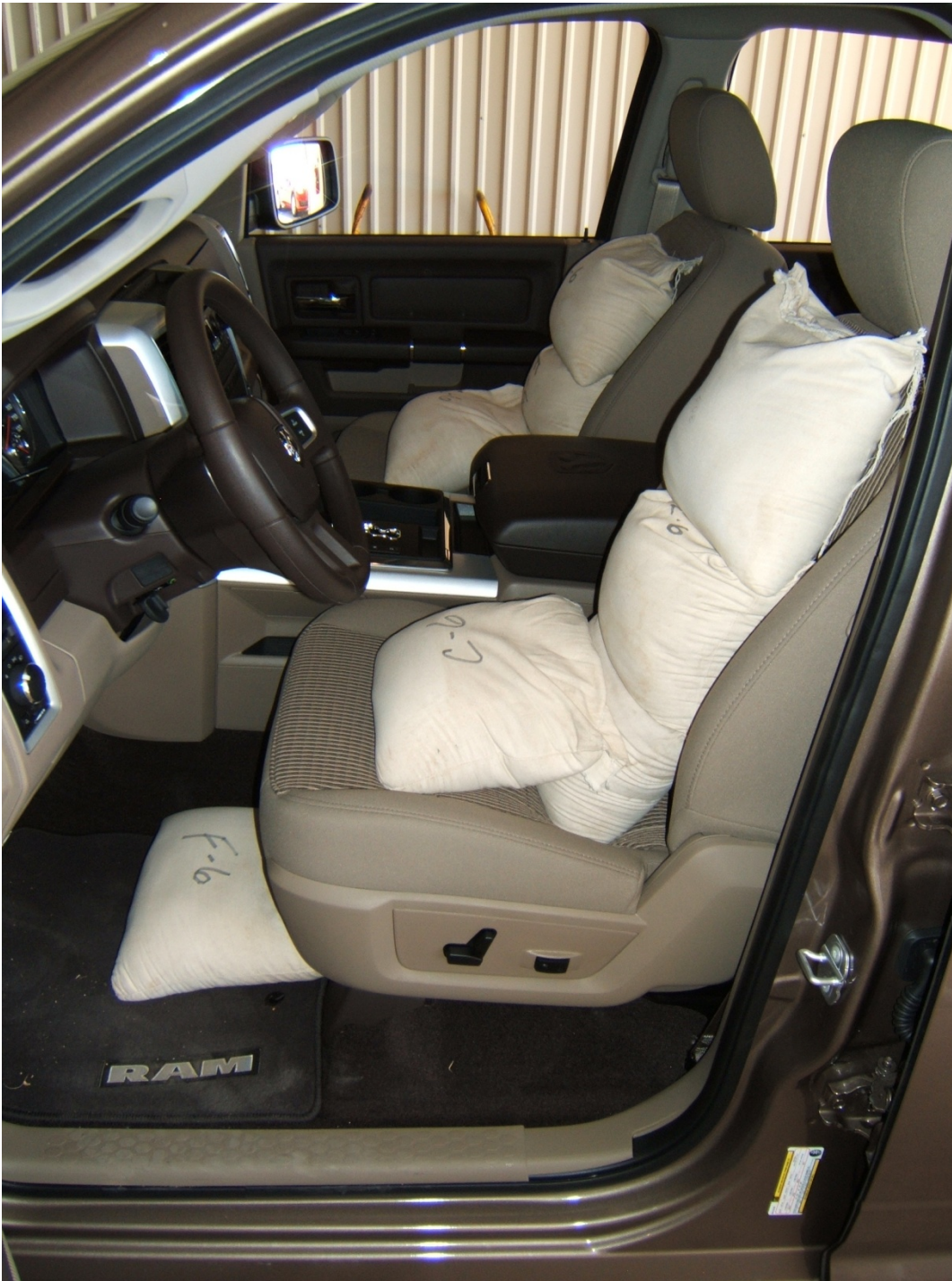
FIGURE 5.13 VEHICLE FRONT SEAT BALLASTED FOR NORMAL, FULL, AND MAXIMUM LOADS
