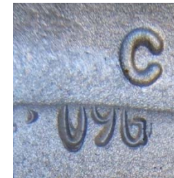
FIGURE 5.11 RIM MARKINGS INCLUDING DOT SYMBOL, LETTER DESIGNATION FOR SOURCE OF PUBLISHED DIMENSIONS, MANUFACTURER, RIM SIZE, AND MANUFACTURE DATE
