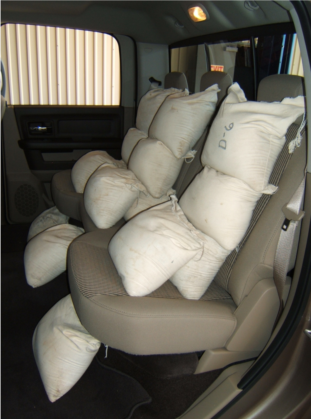
FIGURE 5.15 VEHICLE REAR SEAT BALLASTED FOR FULL AND MAXIMUM LOADS
