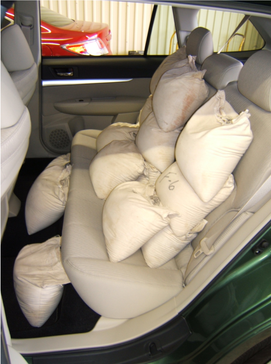
FIGURE 5.14 VEHICLE REAR SEAT BALLASTED FOR FULL AND MAXIMUM LOADS
