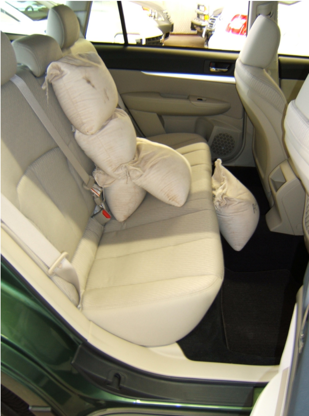
FIGURE 5.13 VEHICLE REAR SEAT BALLASTED FOR NORMAL LOAD
