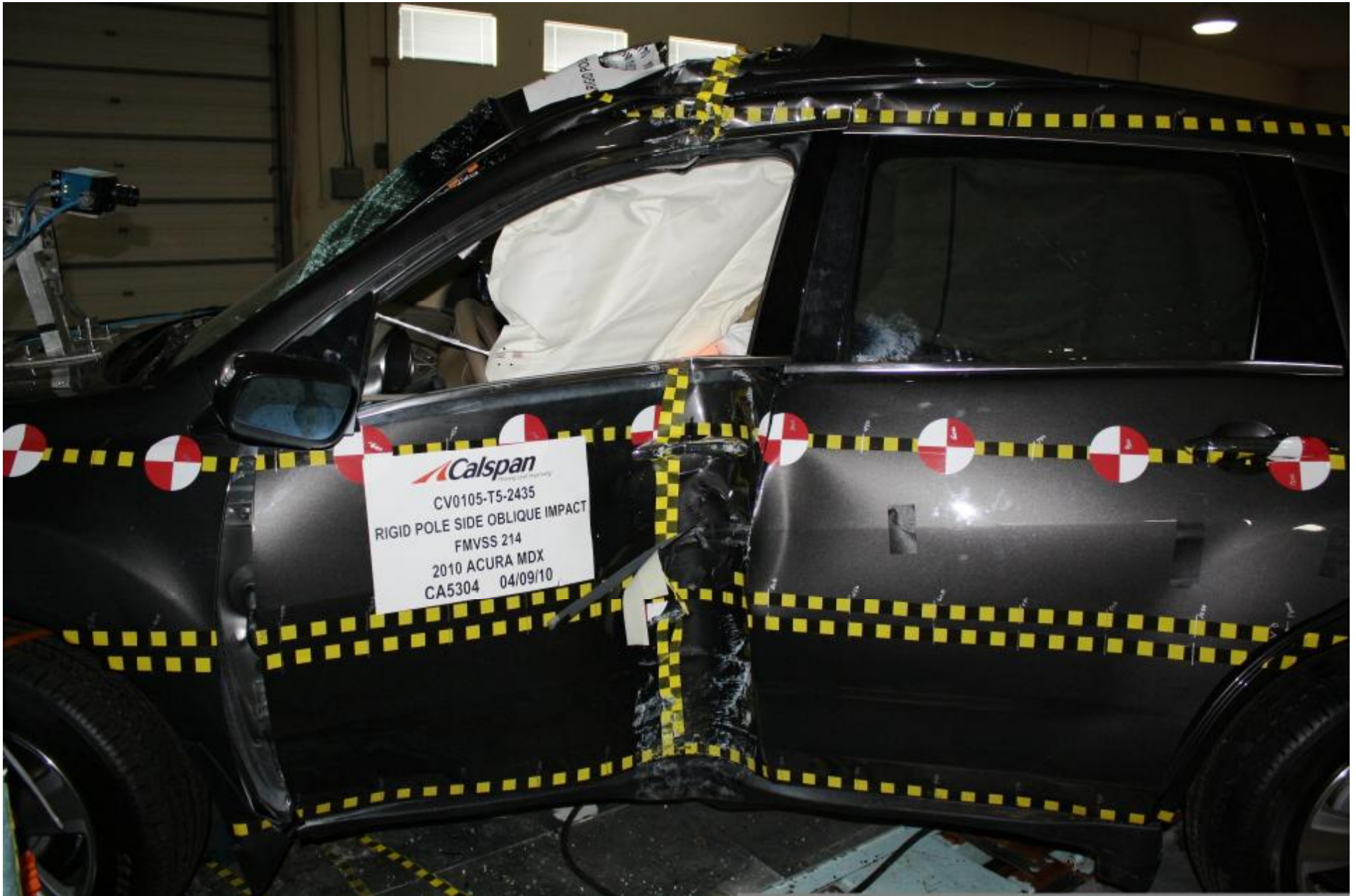
FIGURE A-21 : Post-Test Impact Zone Close-up View
