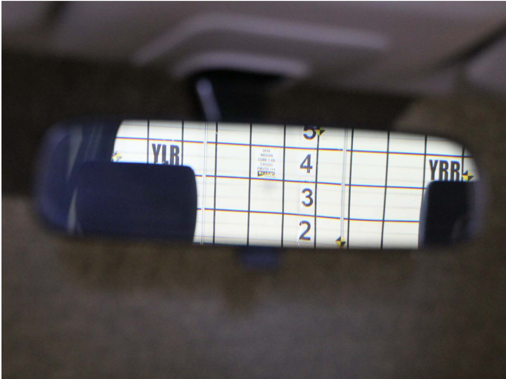
FIGURE 18:RIGHT EYE FIELD OF VIEW TEST (INSIDE MIRROR)
