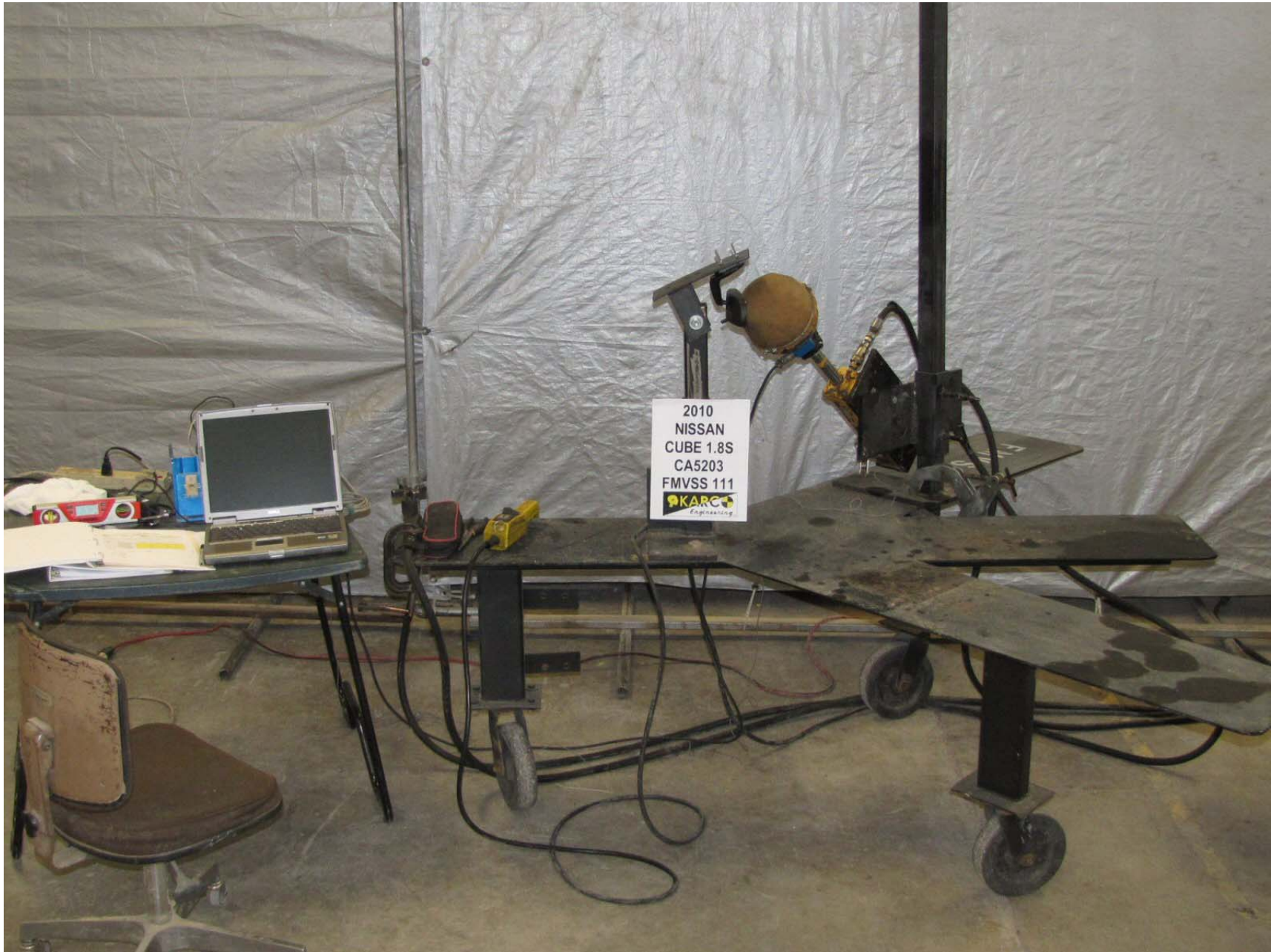
2010 NISSAN CUBE 1.8S NHTSA NO. CA5203 FMVSS NO. 111 FIGURE 12: OVERALL SET-UP AND INSTRUMENTATION FOR MIRROR BREAK- AWAY TEST
