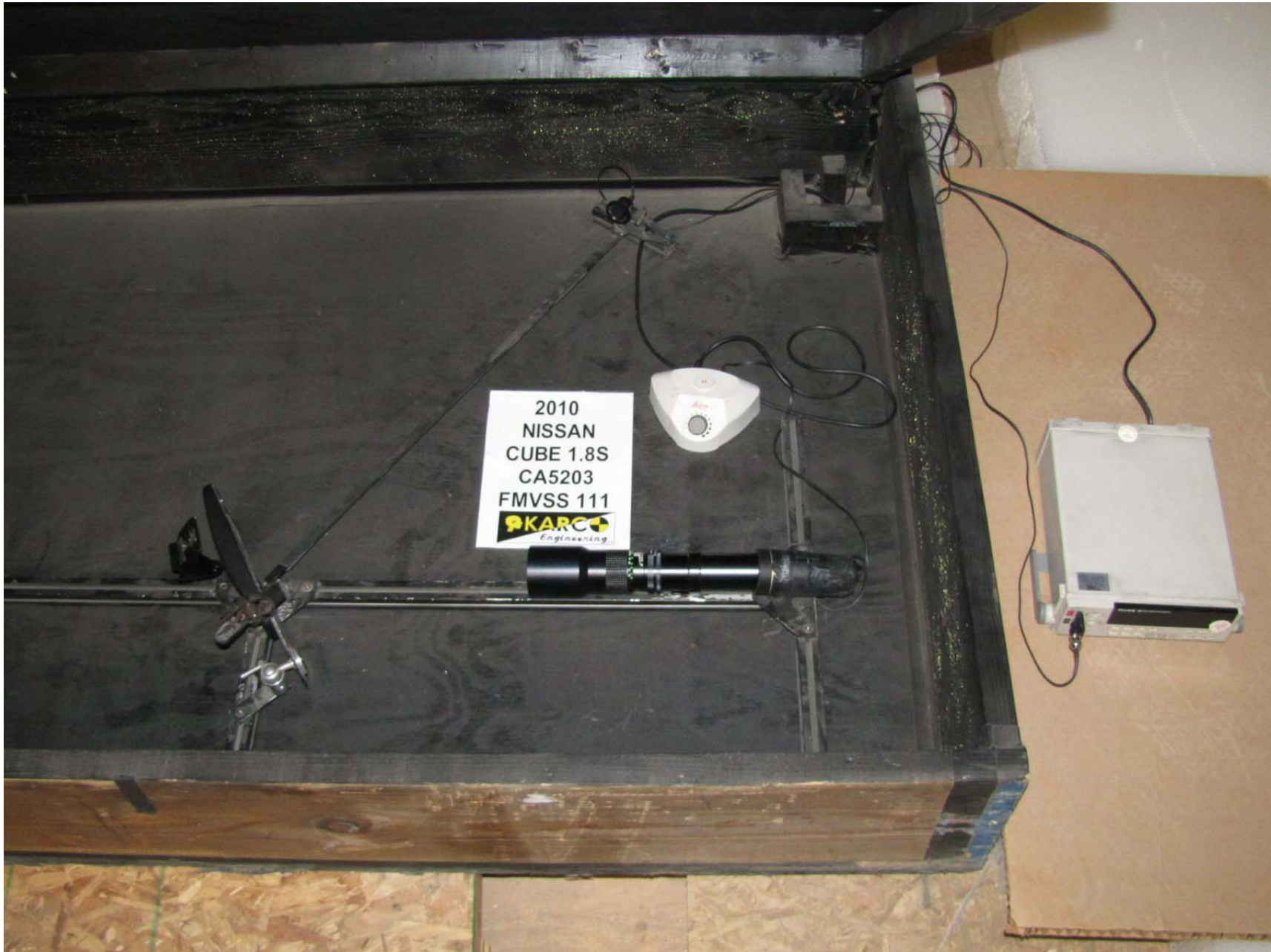
FIGURE 14: REFLECTION TEST SET-UP
