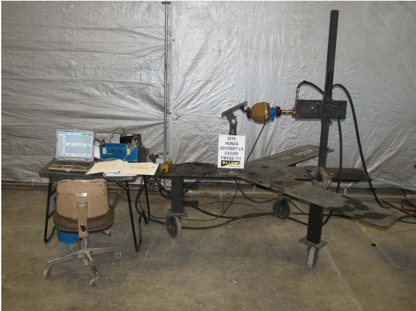
2010 HONDA ODYSSEY LX FIGURE 12: OVERALL SET-UP AND INSTRUMENTATION FOR MIRROR BREAK- AWAY TEST NHTSA NO. CA5305 FMVSS NO. 111
