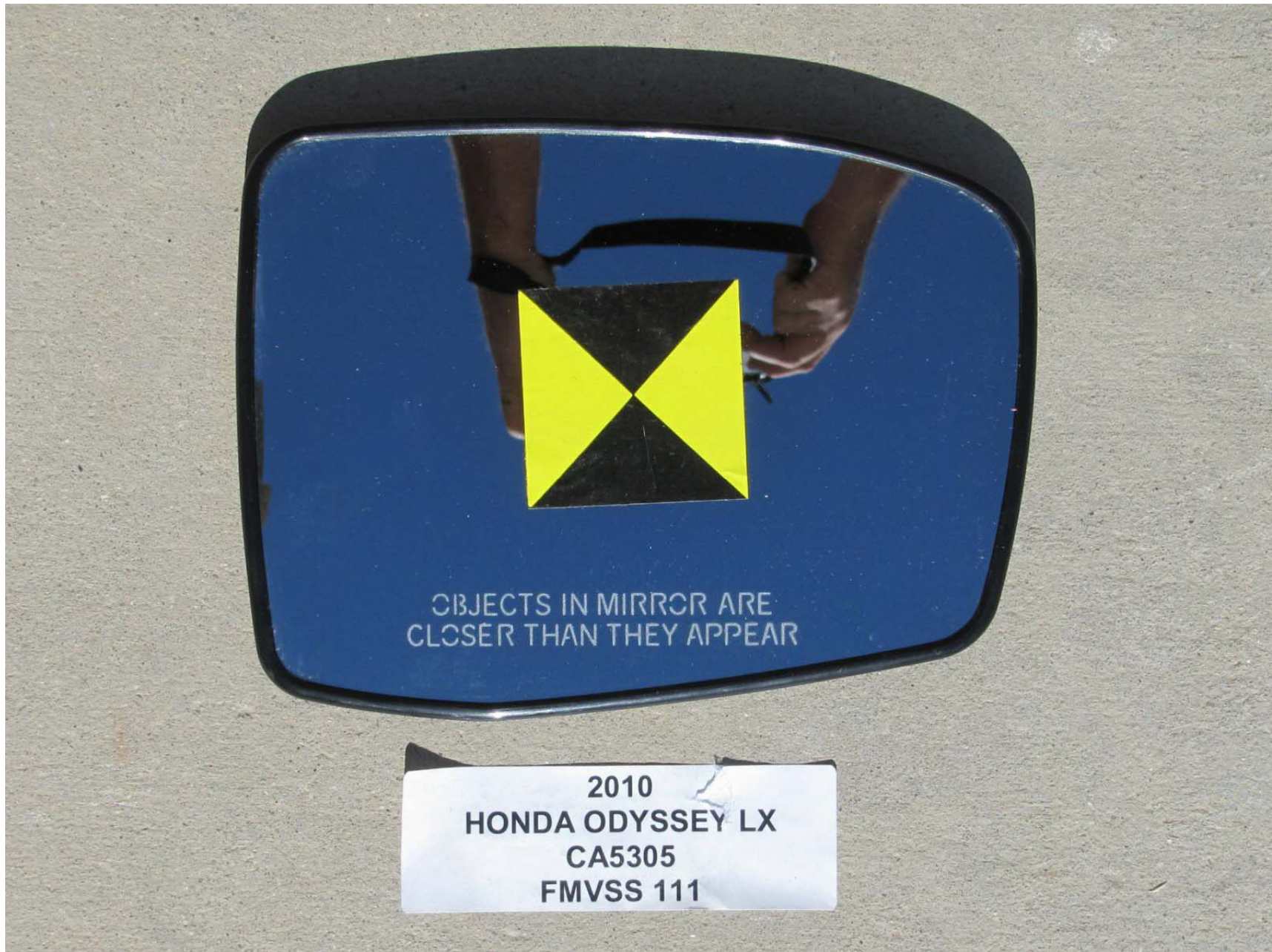
FIGURE 15: MIRROR SET-UP FOR AREA MEASUREMENT
