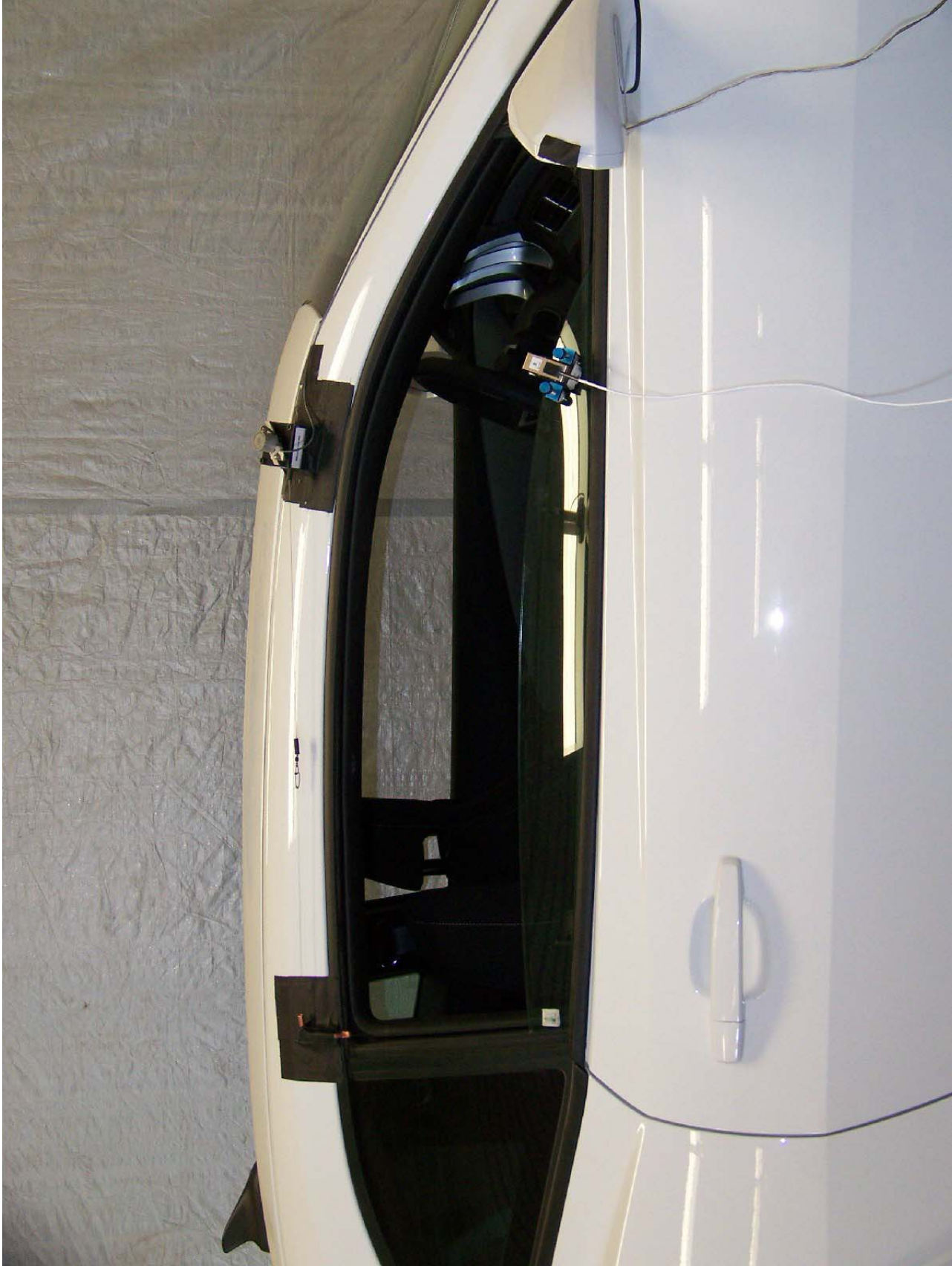
Figure 16: Right Front Window Test Set-Up Leading Edge
