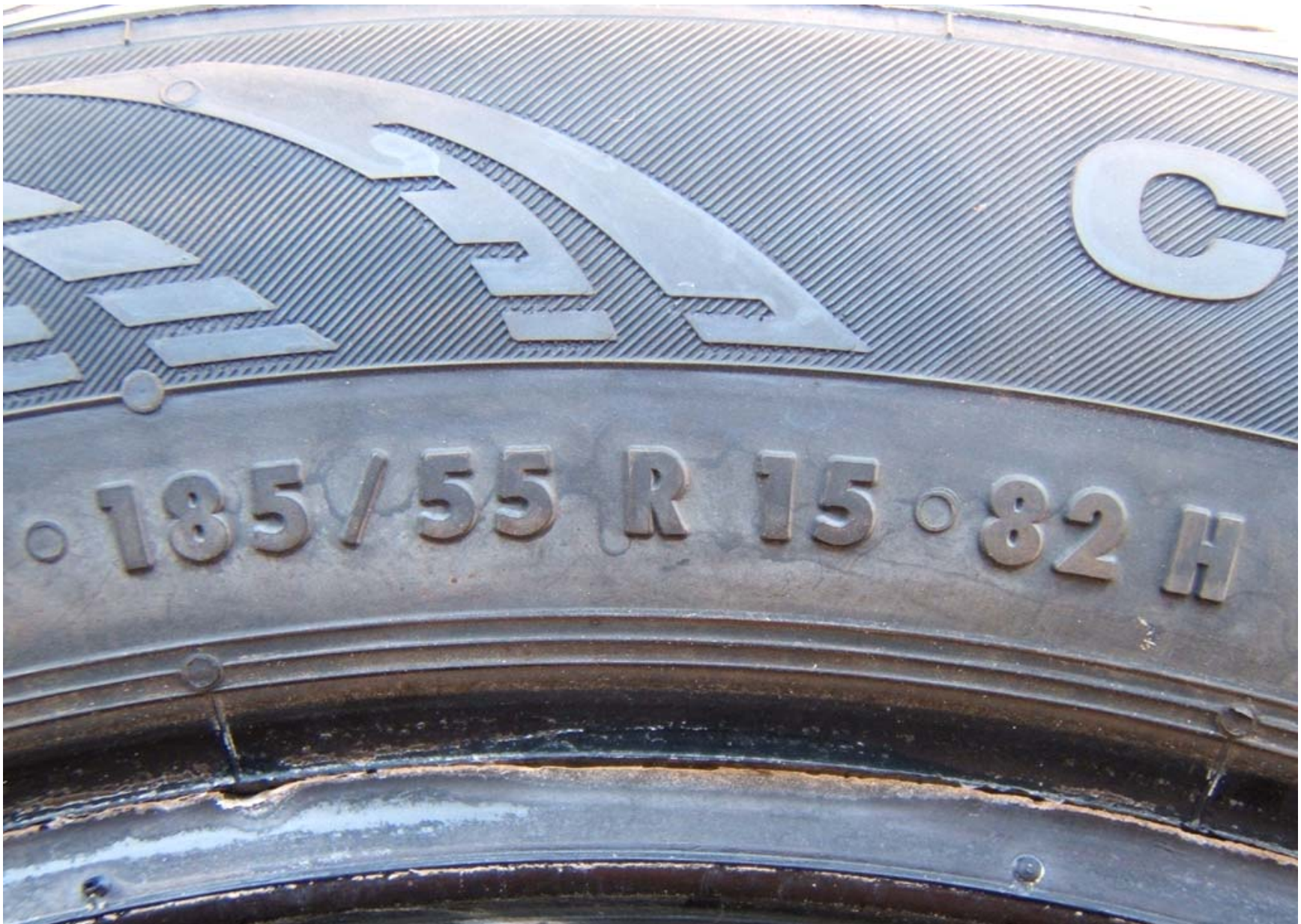
FIGURE 5.7 TIRE SHOWING SIZE, LOAD INDEX, AND SPEED SYMBOL
