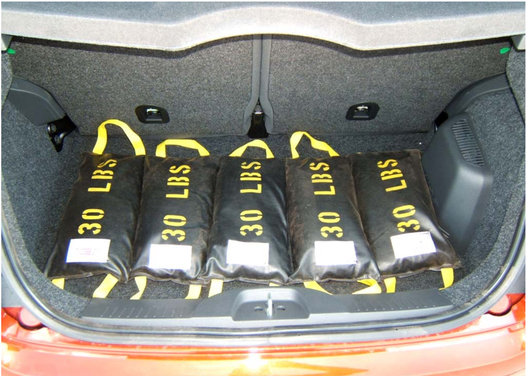
FIGURE 5.15 VEHICLE TRUNK BALLASTED FOR MAXIMUM LOAD
