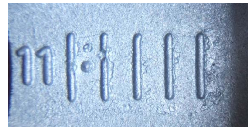
FIGURE 5.11 RIGHT FRONT RIM SHOWING MANUFACTURER, DATE OF MANUFACTURE, SIZE, DESIGNATION FOR SOURCE OF PUBLISHED DIMENSIONS, DOT SYMBOL, AND OTHER RIM MARKINGS
