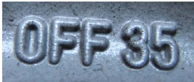
FIGURE 5.11 RIGHT FRONT RIM SHOWING MANUFACTURER, DATE OF MANUFACTURE, SIZE, DESIGNATION FOR SOURCE OF PUBLISHED DIMENSIONS, DOT SYMBOL, AND OTHER RIM MARKINGS
