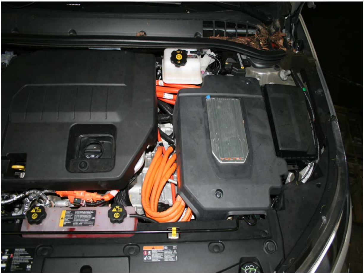
Power Inverter Warning Label/Location
