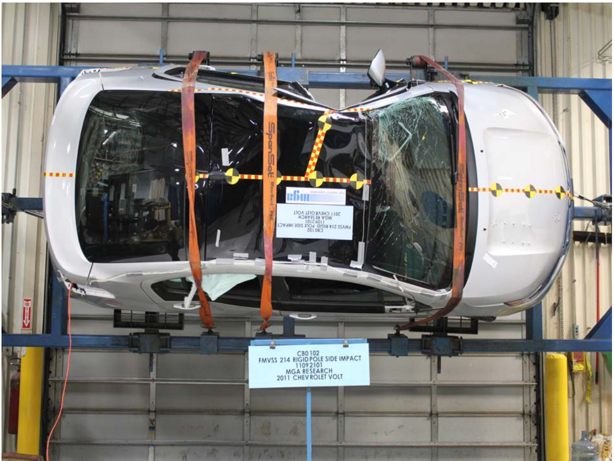
Vehicle at 90 Degrees on Static Rollover Device
