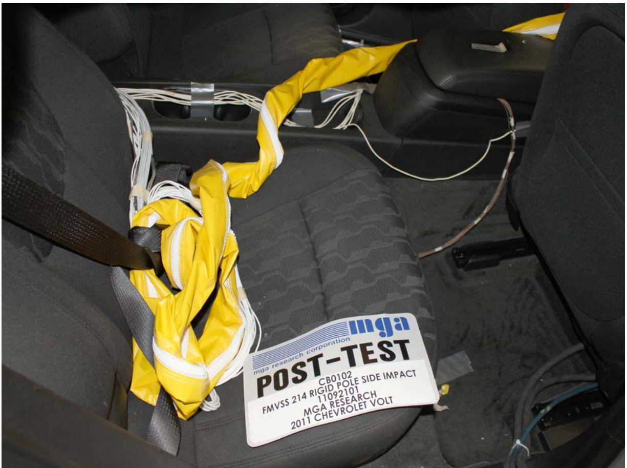
Post-Test View of Vehicle's Passenger Compartment Adjacent to Propulsion Battery
