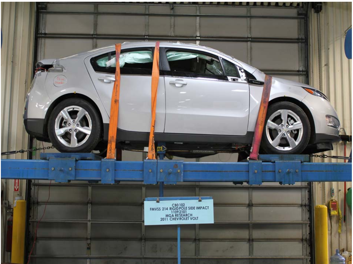
Vehicle at 360 Degrees on Static Rollover Device
