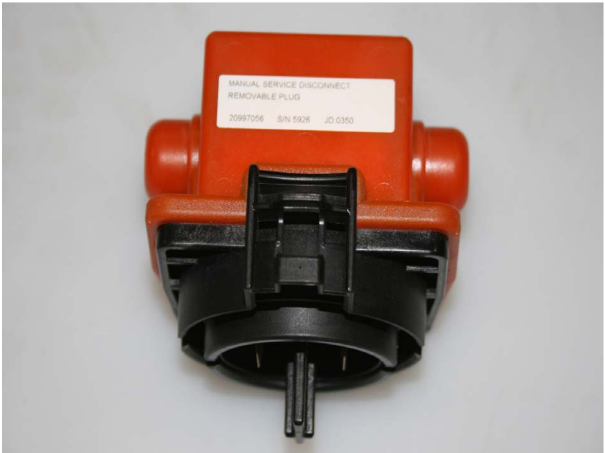
Manual High Voltage Service Disconnect
