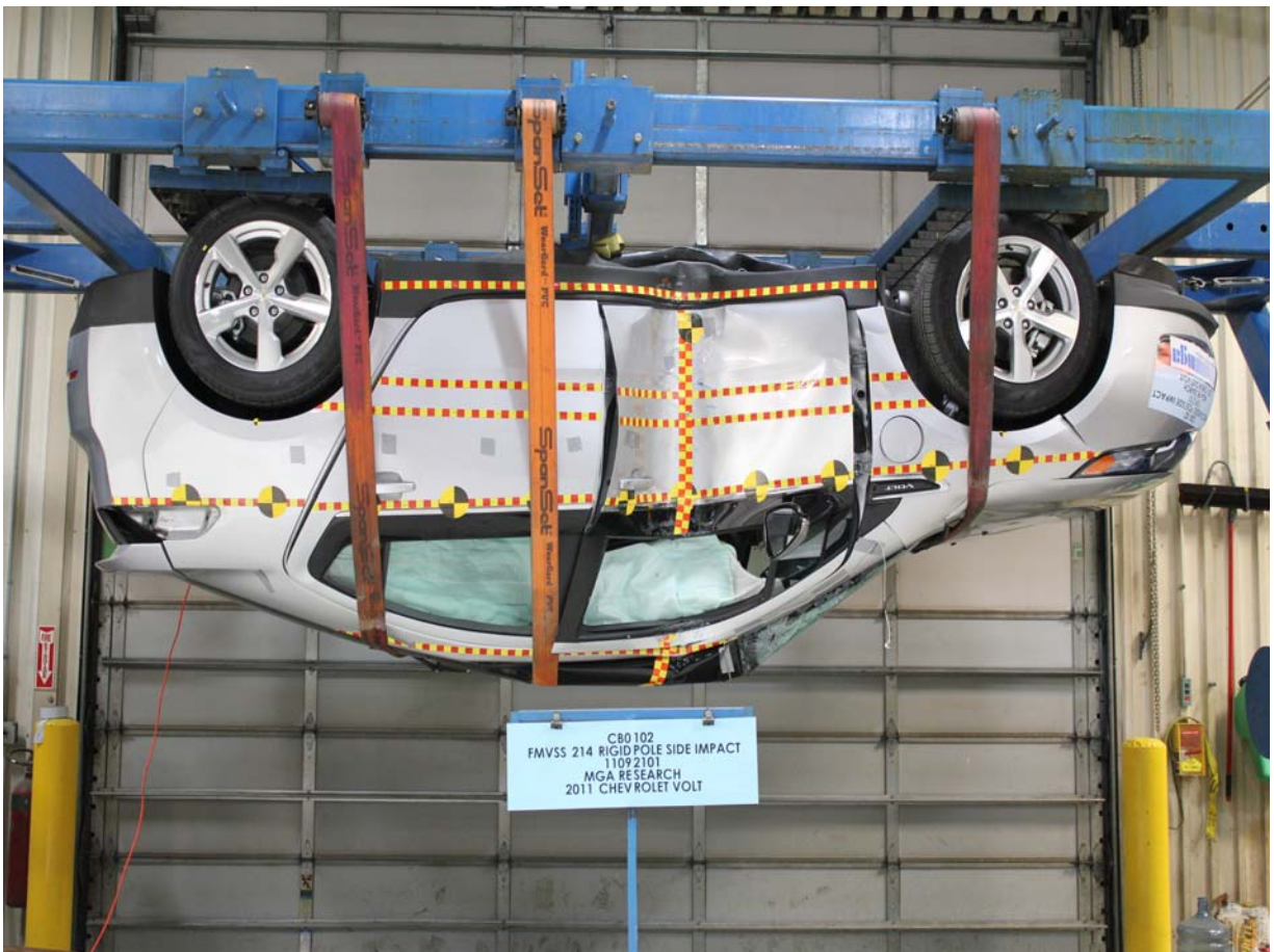
Vehicle at 180 Degrees on Static Rollover Device
