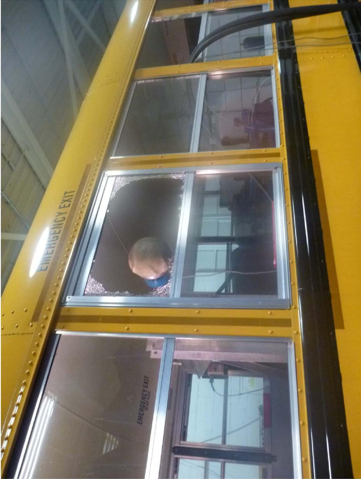
Window Retention Test of W19 Emergency Exit Upper Pane Post-Test (Passenger Side)
