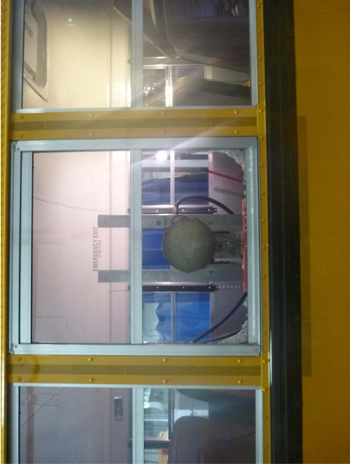
Window Retention Test of W5 Emergency Exit Lower Pane Post-Test (Driver Side)
