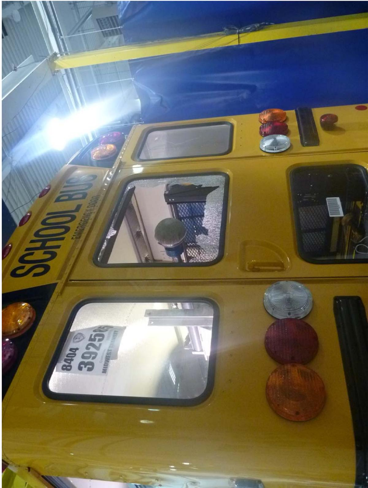
Window Retention Test of Rear Emergency Door Upper Pane Post-Test
