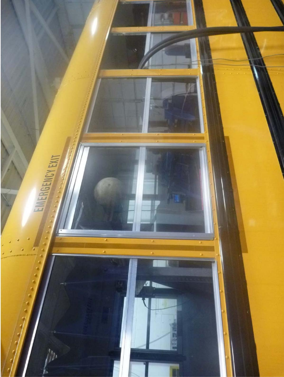
Window Retention Test of W19 Emergency Exit Upper Pane Pre-Test (Passenger Side)
