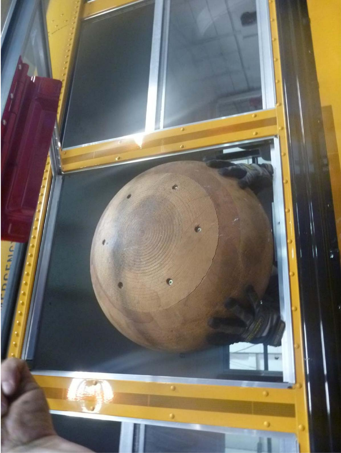
Emergency Exit Window Ellipsoid Clearance
