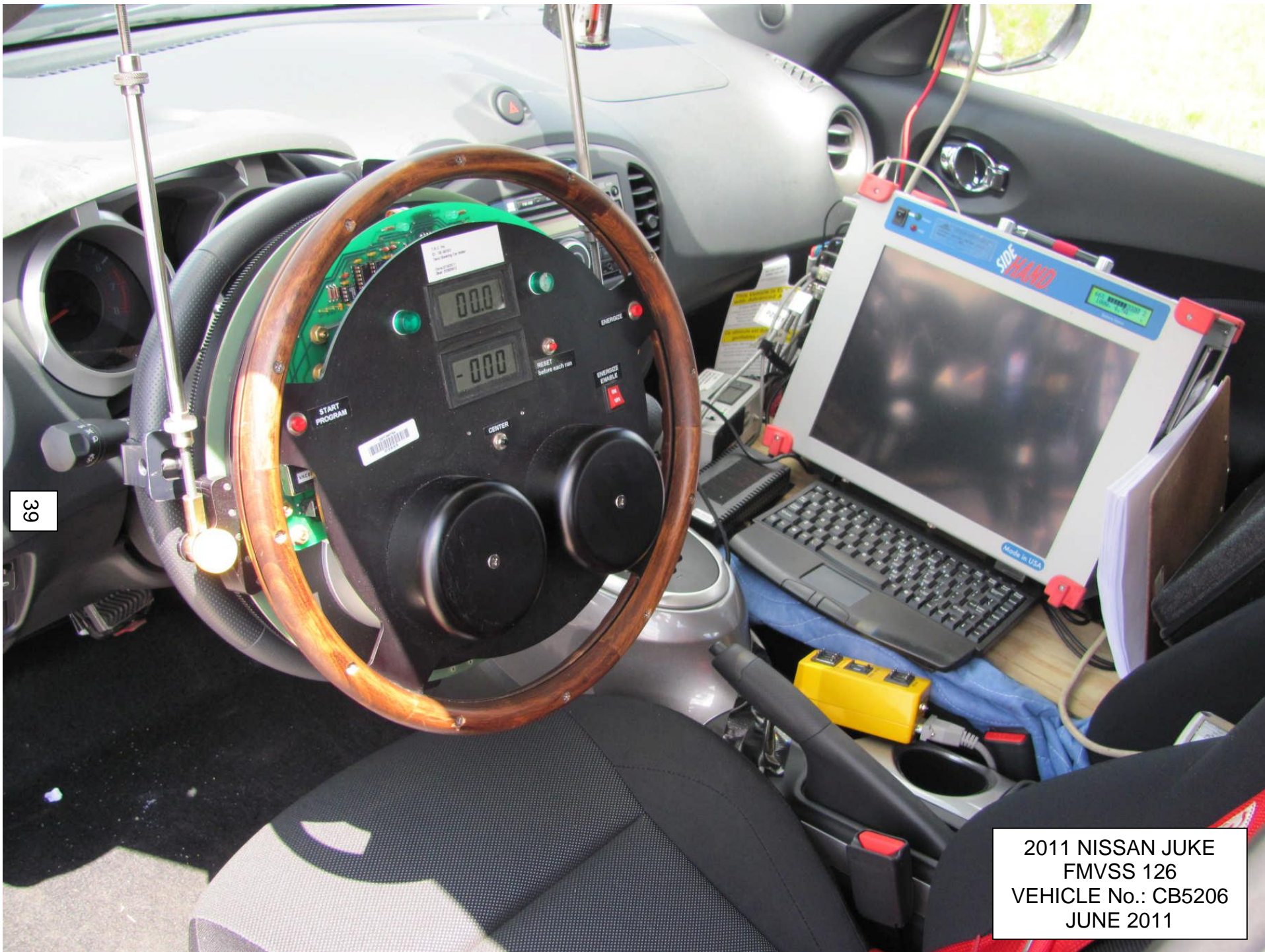
5.11 STEERING WHEEL CONTROLLER AND DATA ACQUISITION SYSTEM
