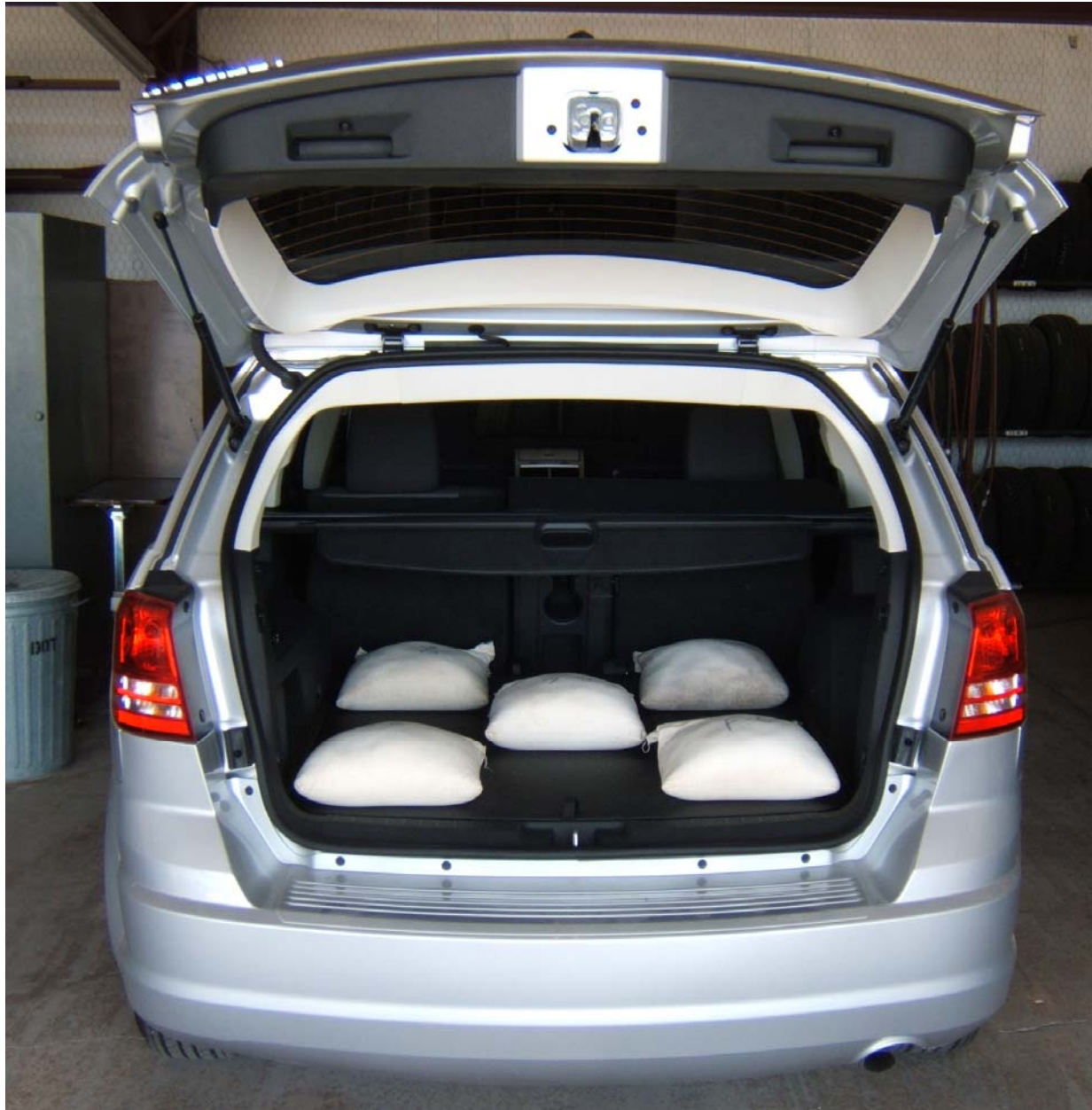
FIGURE 5.18 CARGO AREA SHOWN BALLASTED FOR MAXIMUM LOAD
