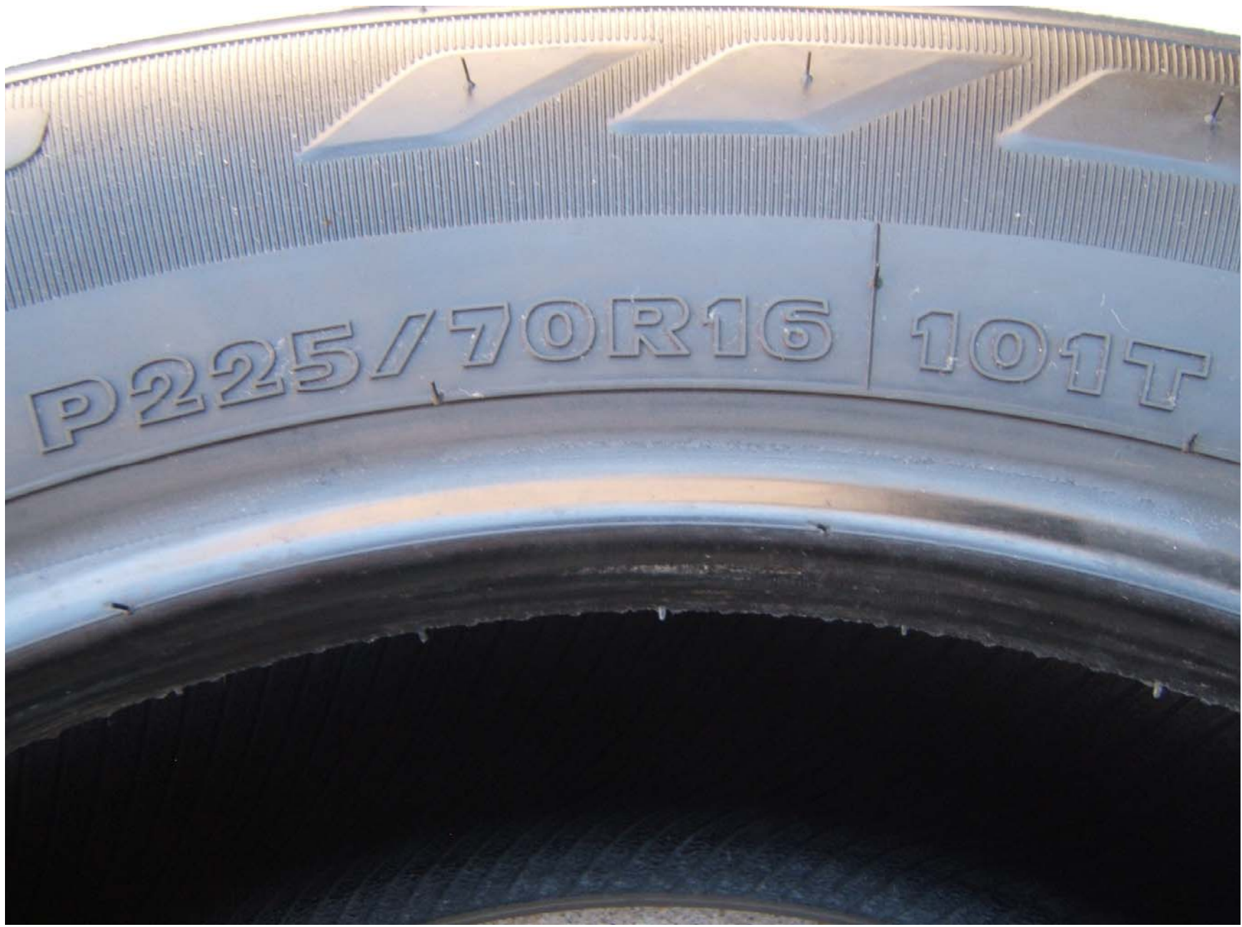
FIGURE 5.7 TIRE SHOWING SIZE, LOAD INDEX, AND SPEED SYMBOL
