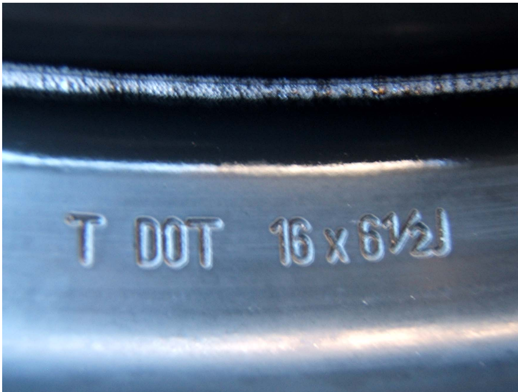
FIGURE 5.12 RIM SHOWING SOURCE OF PUBLISHED DIMENSIONS, DOT SYMBOL, AND SIZE
