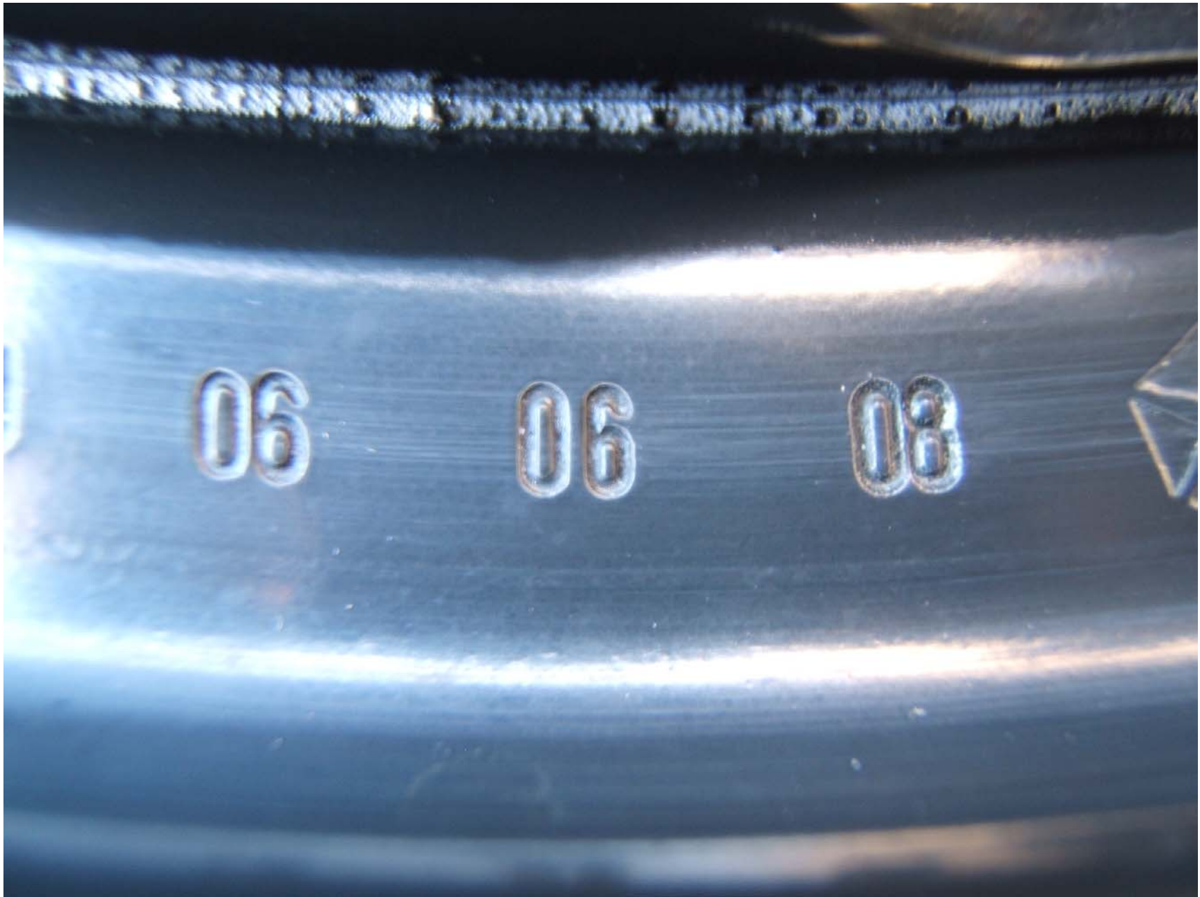
FIGURE 5.11 RIM SHOWING MANUFACTURE DATE
