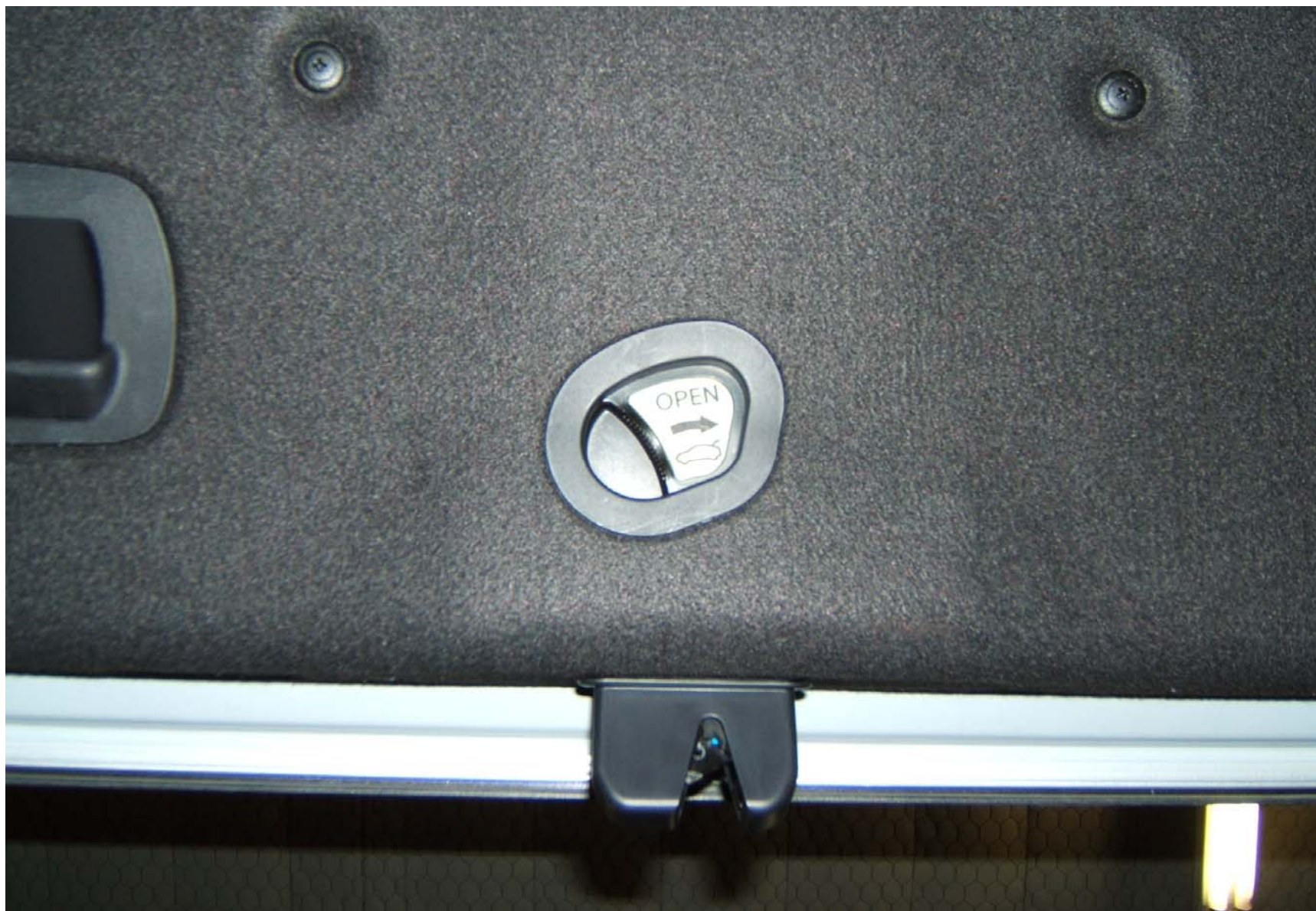
FIGURE 5.8 VEHICLE TRUNK COMPARTMENT MANUAL RELEASE MECHANISM
