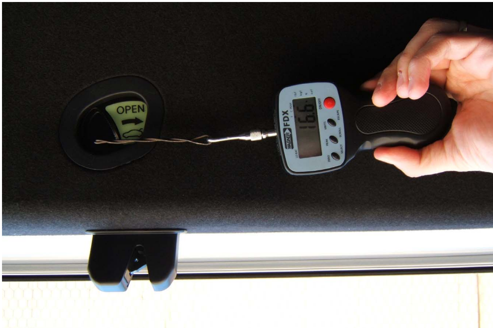
FIGURE 5.9 RELEASE MECHANISM WITH TEST EQUIPMENT ATTACHED
