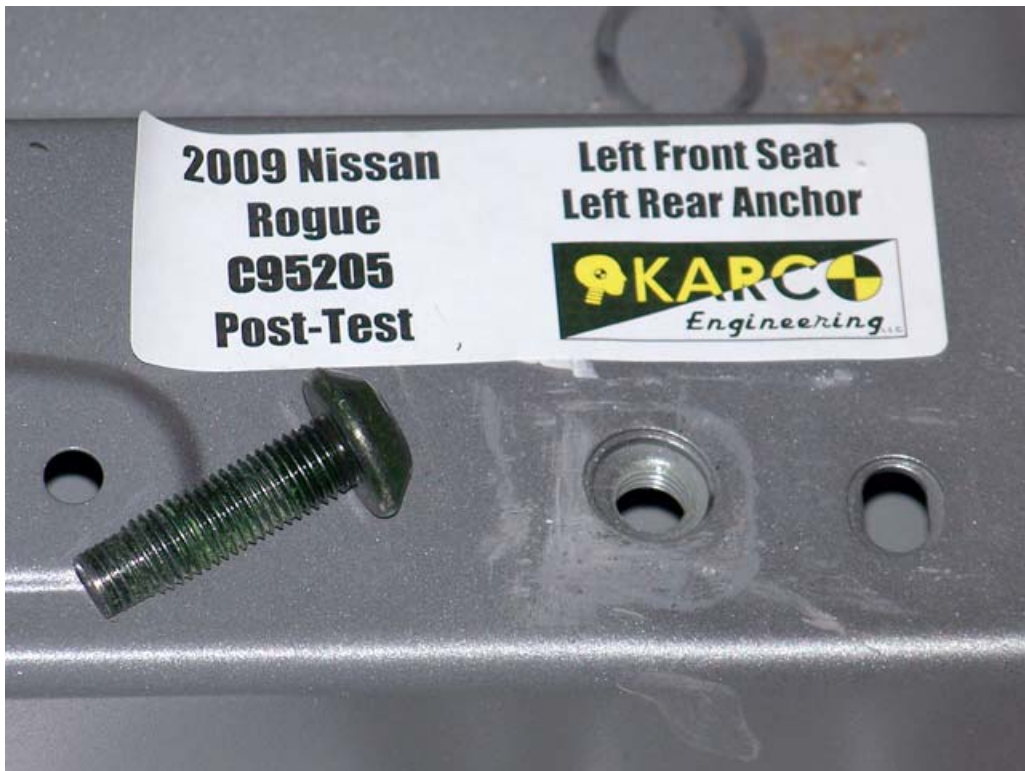
FIGURE 52. Floor Pan Anchor, P1, Post-Test
