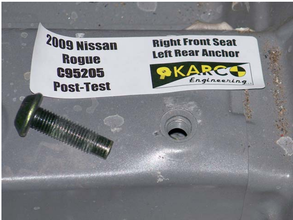
FIGURE 80. Floor Pan Anchor, P2, Post-Test
