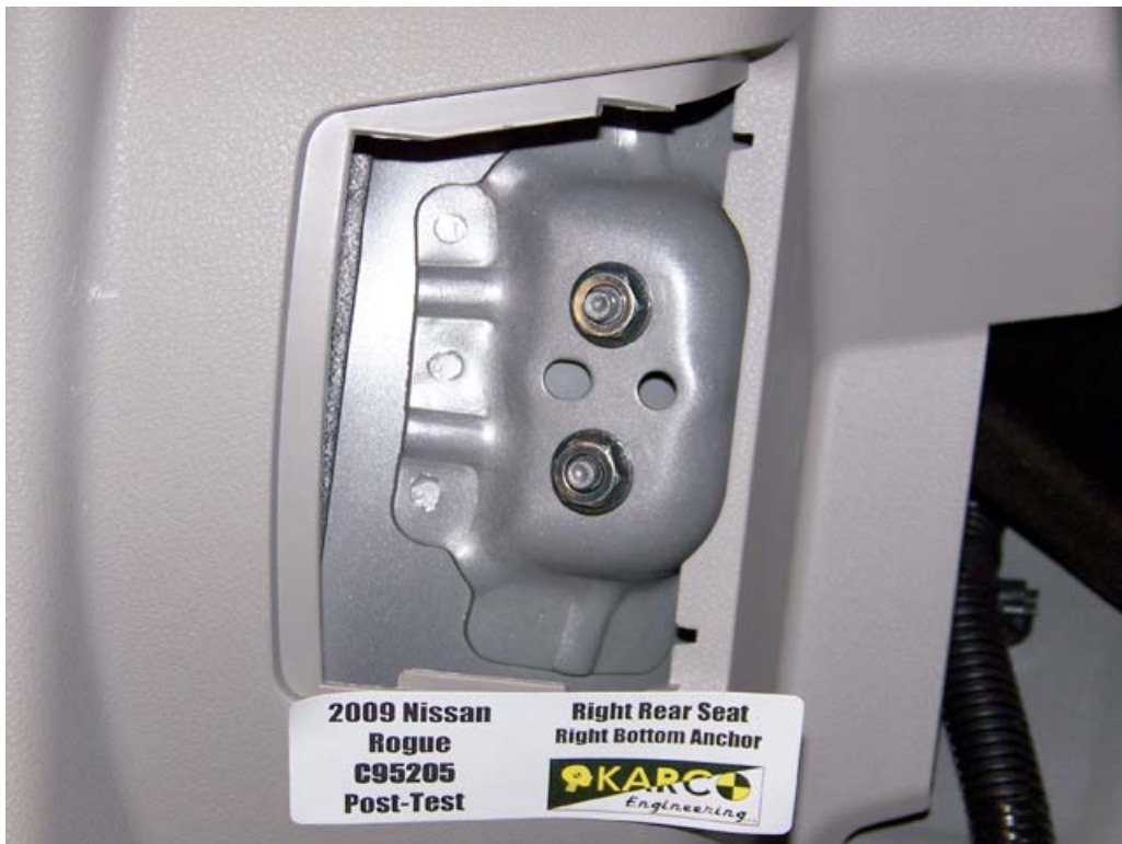
FIGURE 112. Floor Pan Anchor, P3, Post-Test
