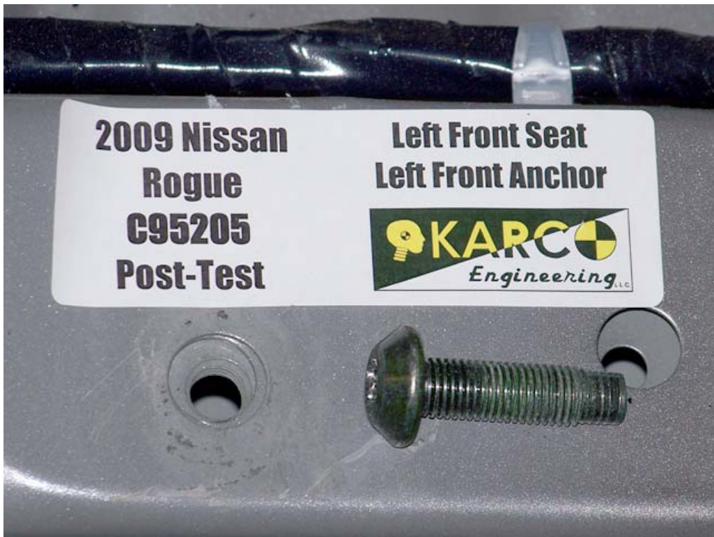
FIGURE 44. Floor Pan Anchor, P1, Post-Test
