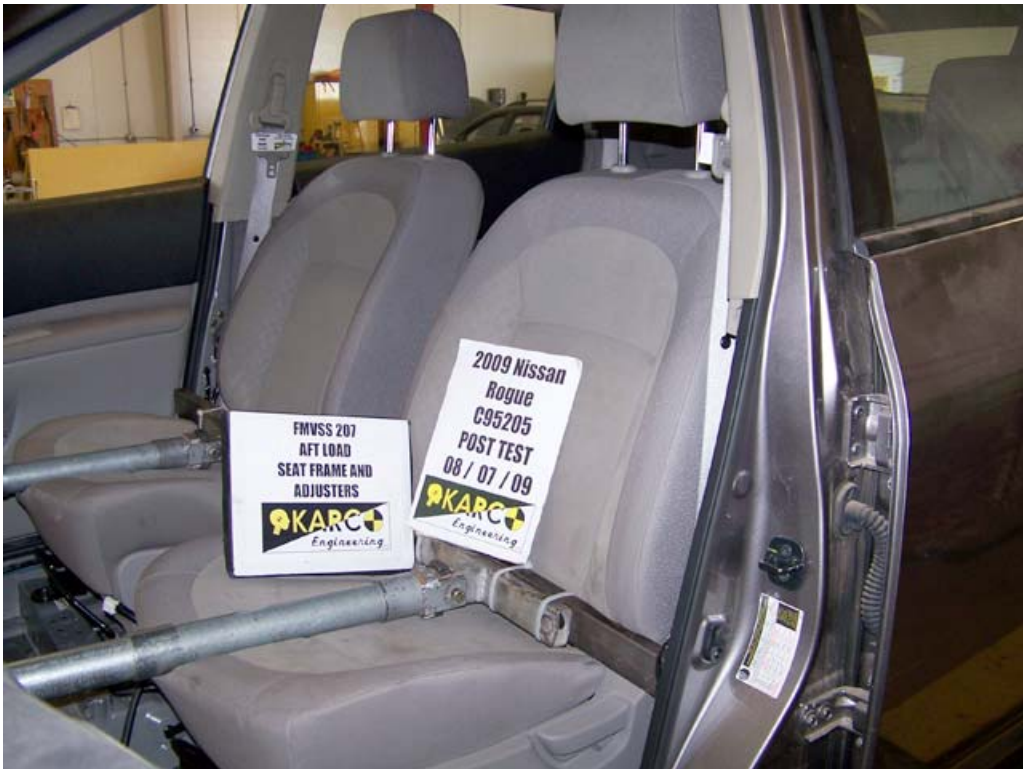
FIGURE 20. Aft Load on Seat Frame and Adjusters, P1, Post-Test
