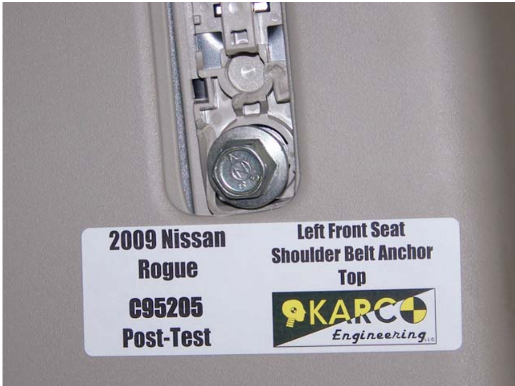
FIGURE 60. Shoulder Belt Anchor, P1, Post-Test
