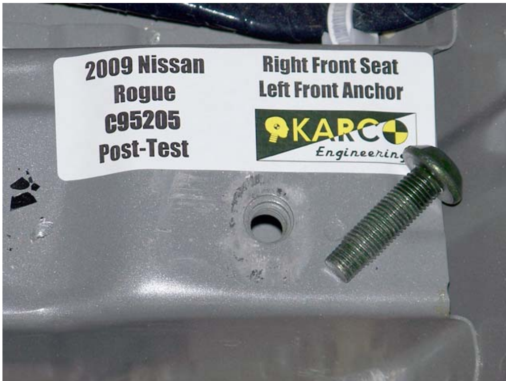
FIGURE 72. Floor Pan Anchors, P2, Post-Test
