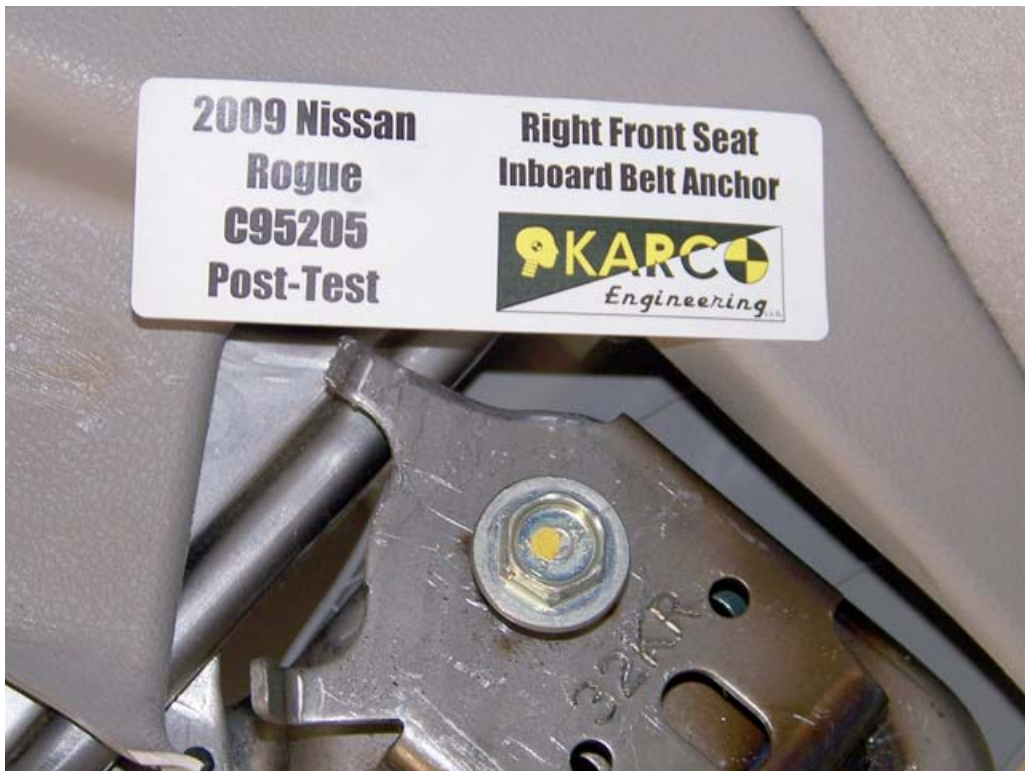
FIGURE 94. Belt Anchor, P2, Post-Test
