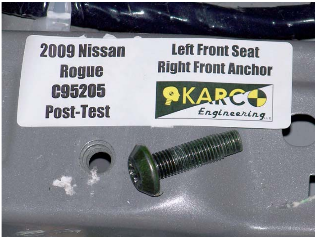
FIGURE 48. Floor Pan Anchor, P1, Post-Test
