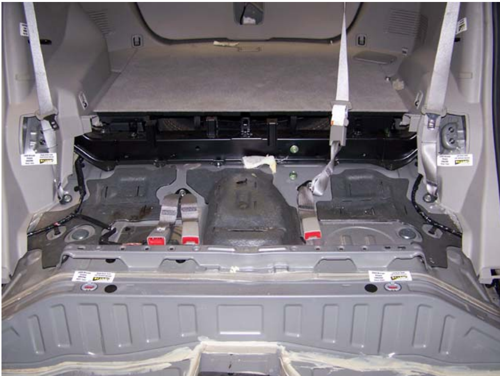
FIGURE 96. Floor Pan Anchors, P3-P4 Overall, Post-Test
