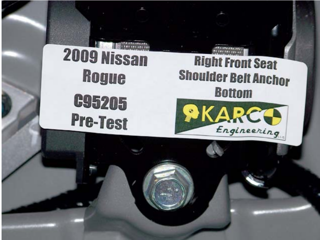
FIGURE 89. Shoulder Belt Anchor, P2, Pre-Test
