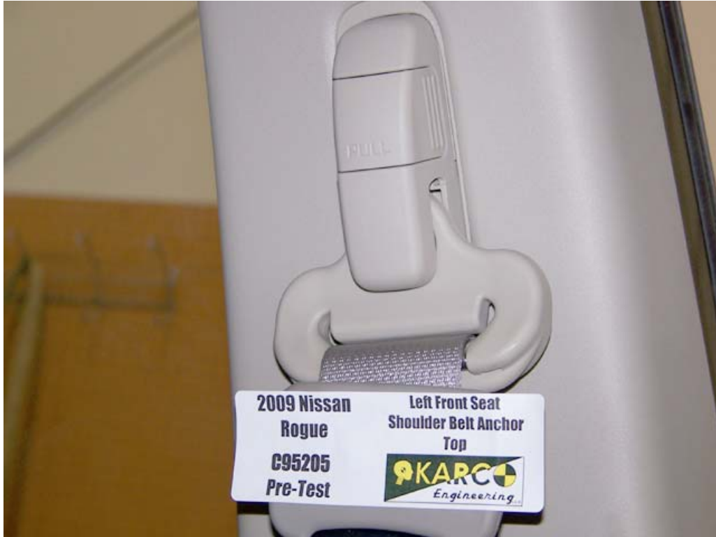
FIGURE 59. Shoulder Belt Anchor, P1, Pre-Test
