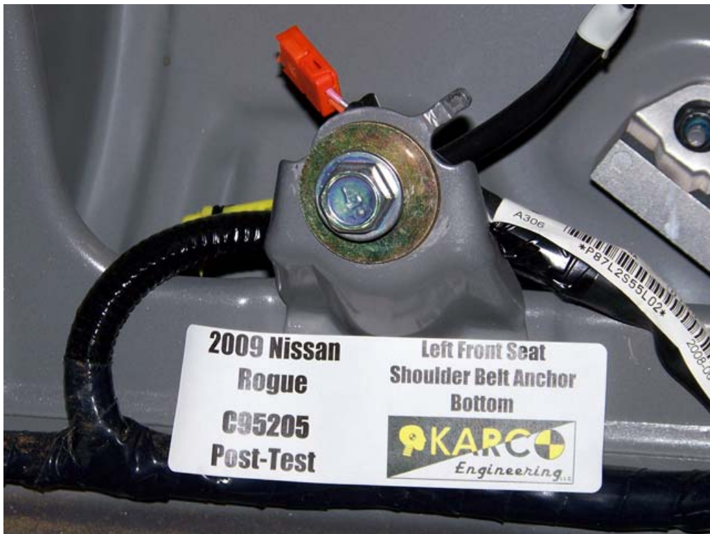
FIGURE 62. Shoulder Belt Anchor, P1, Post-Test
