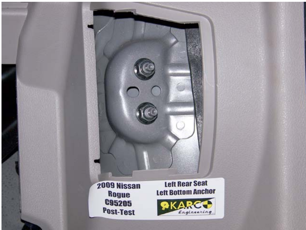
FIGURE 104. Floor Pan Anchor, P4, Post-Test
