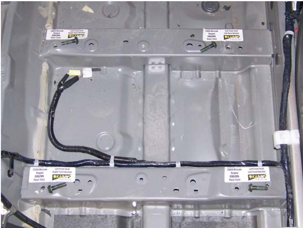
FIGURE 40. Floor Pan Anchors, P1 Overall, Post-Test
