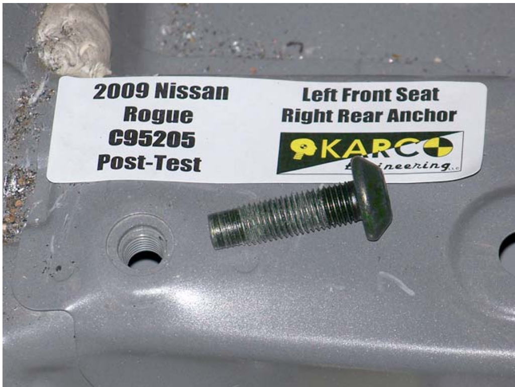
FIGURE 56. Floor Pan Anchor, P1, Post-Test
