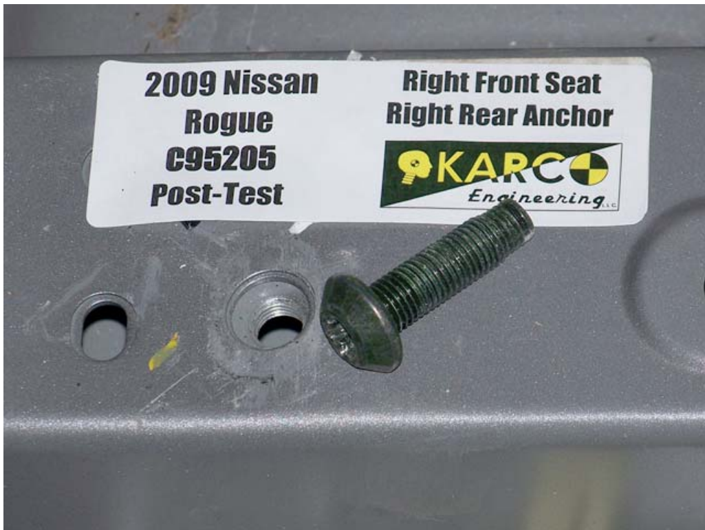
FIGURE 84. Floor Pan Anchor, P2, Post-Test
