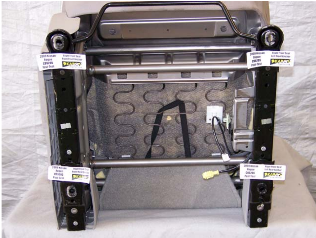
FIGURE 70. Seat Anchors, P2 Overall, Post-Test
