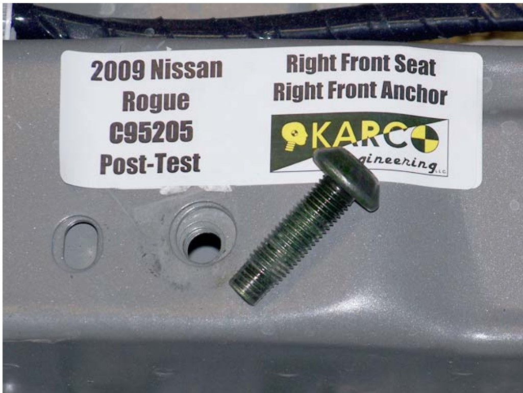
FIGURE 76. Floor Pan Anchors, P2, Post-Test
