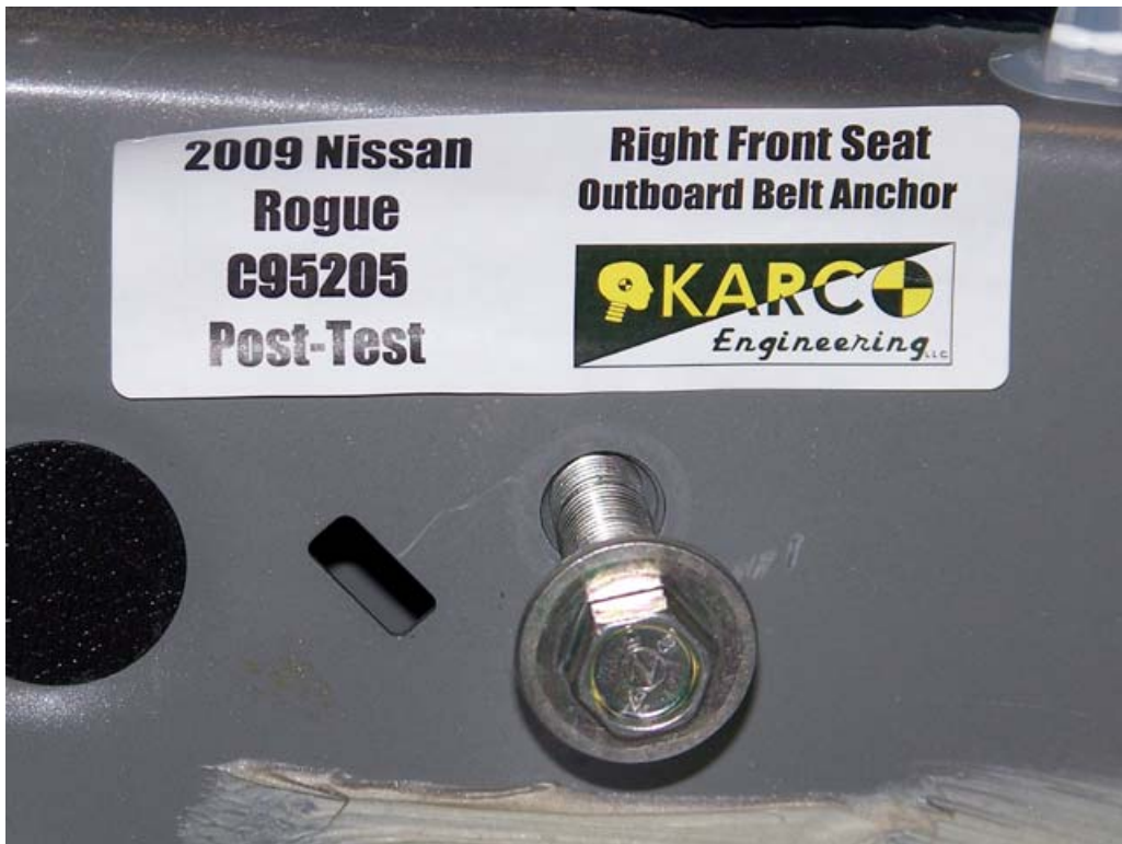
FIGURE 92. Belt Anchor, P2, Post-Test
