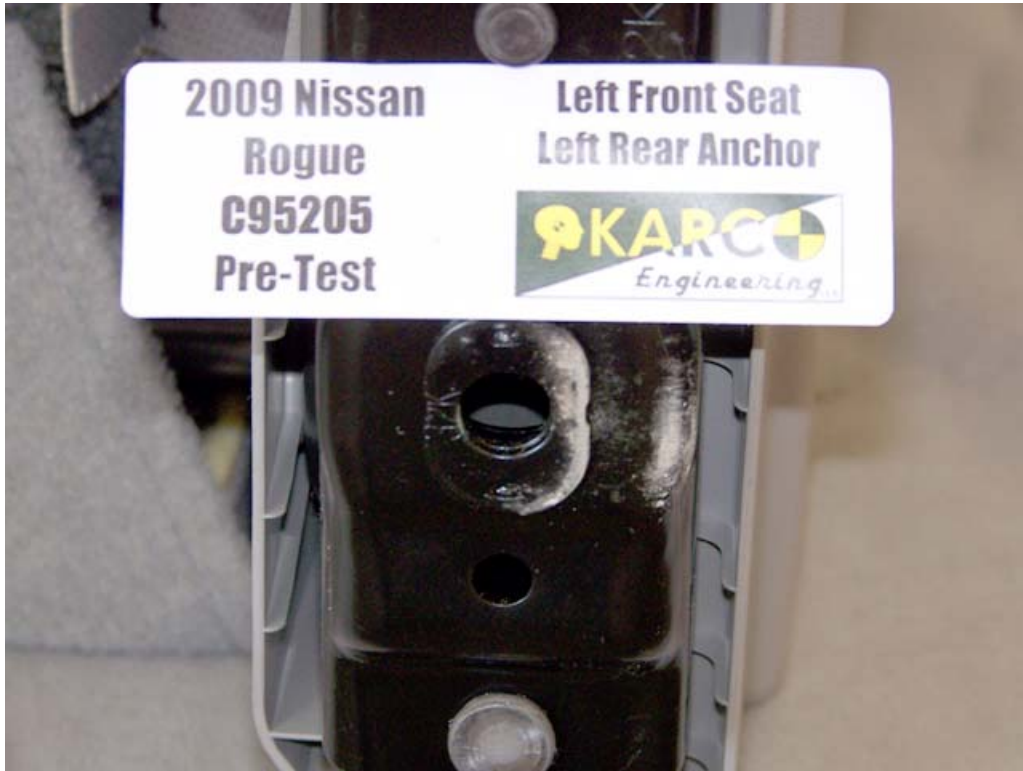
FIGURE 53. Seat Anchor, P1, Pre-Test
