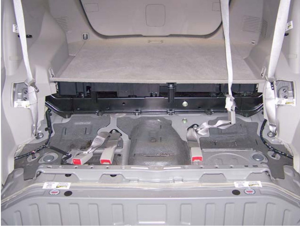
FIGURE 95. Floor Pan Anchors, P3-P4 Overall, Pre-Test
