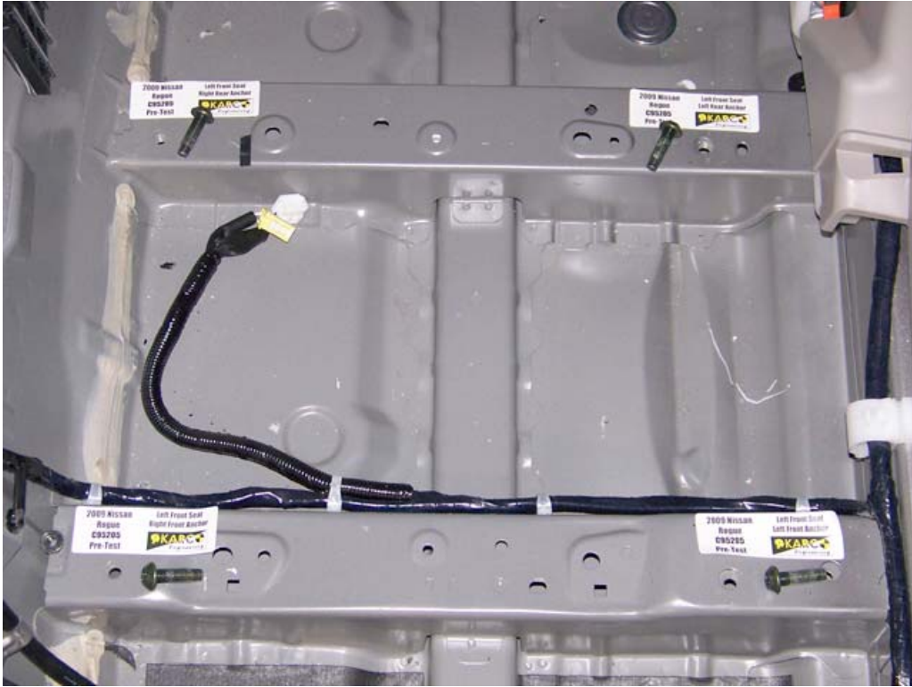
FIGURE 39. Floor Pan Anchors, P1 Overall, Pre-Test
