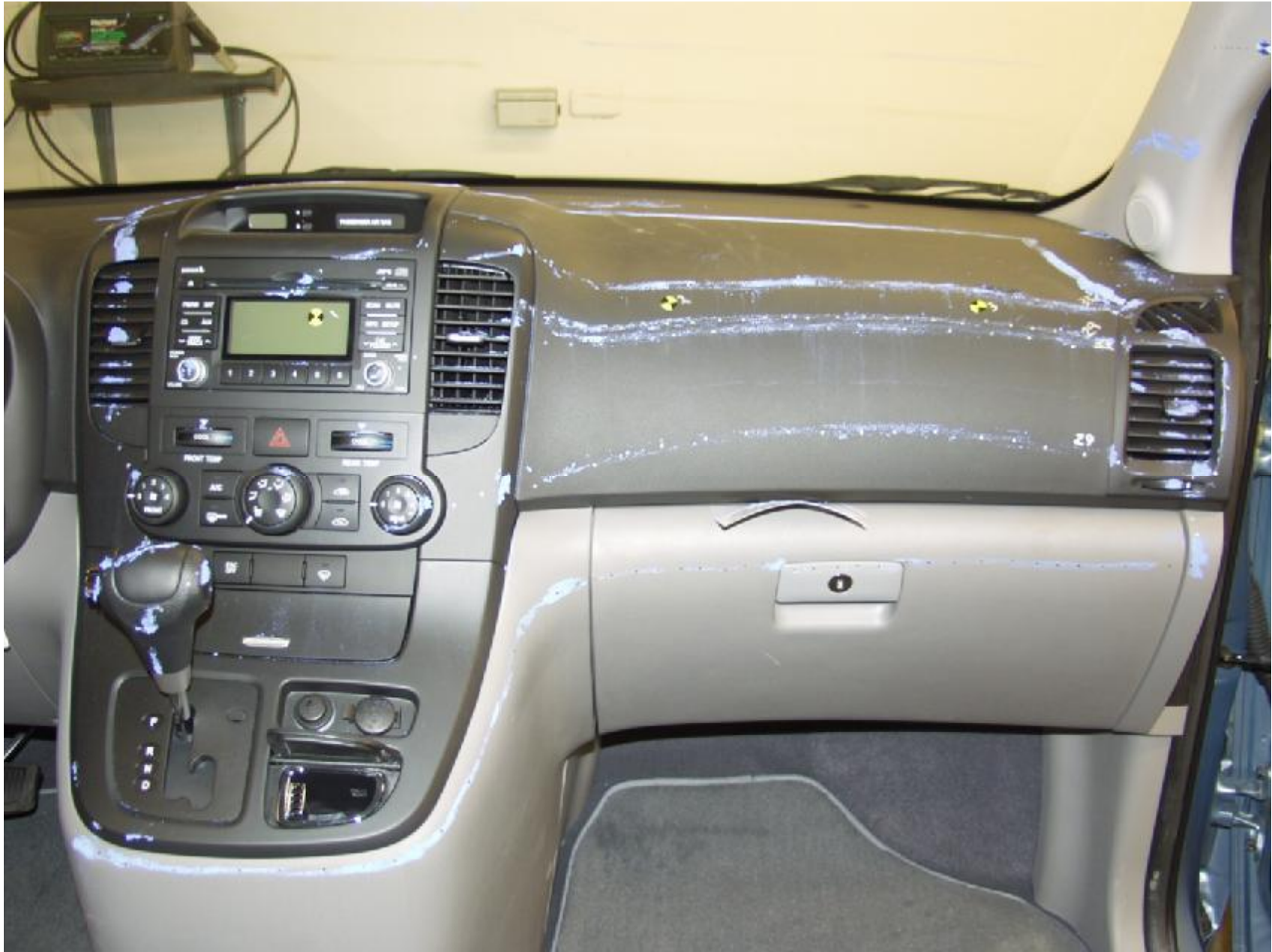
Figure A-13 : DELINEATED INSTRUMENT PANEL IMPACT ZONE PRE-TEST
