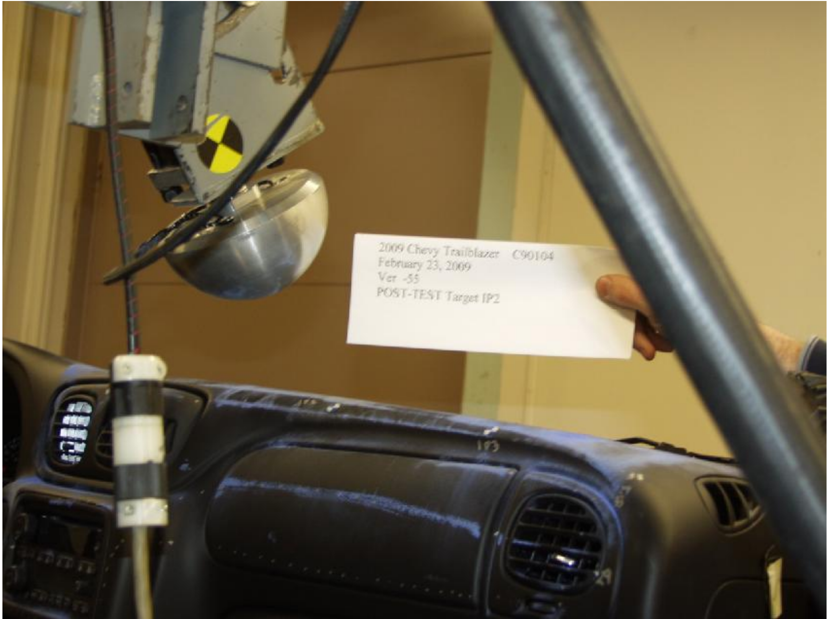
Figure A-17 : INSTRUMENT PANEL IMPACT #2 POST-TEST
