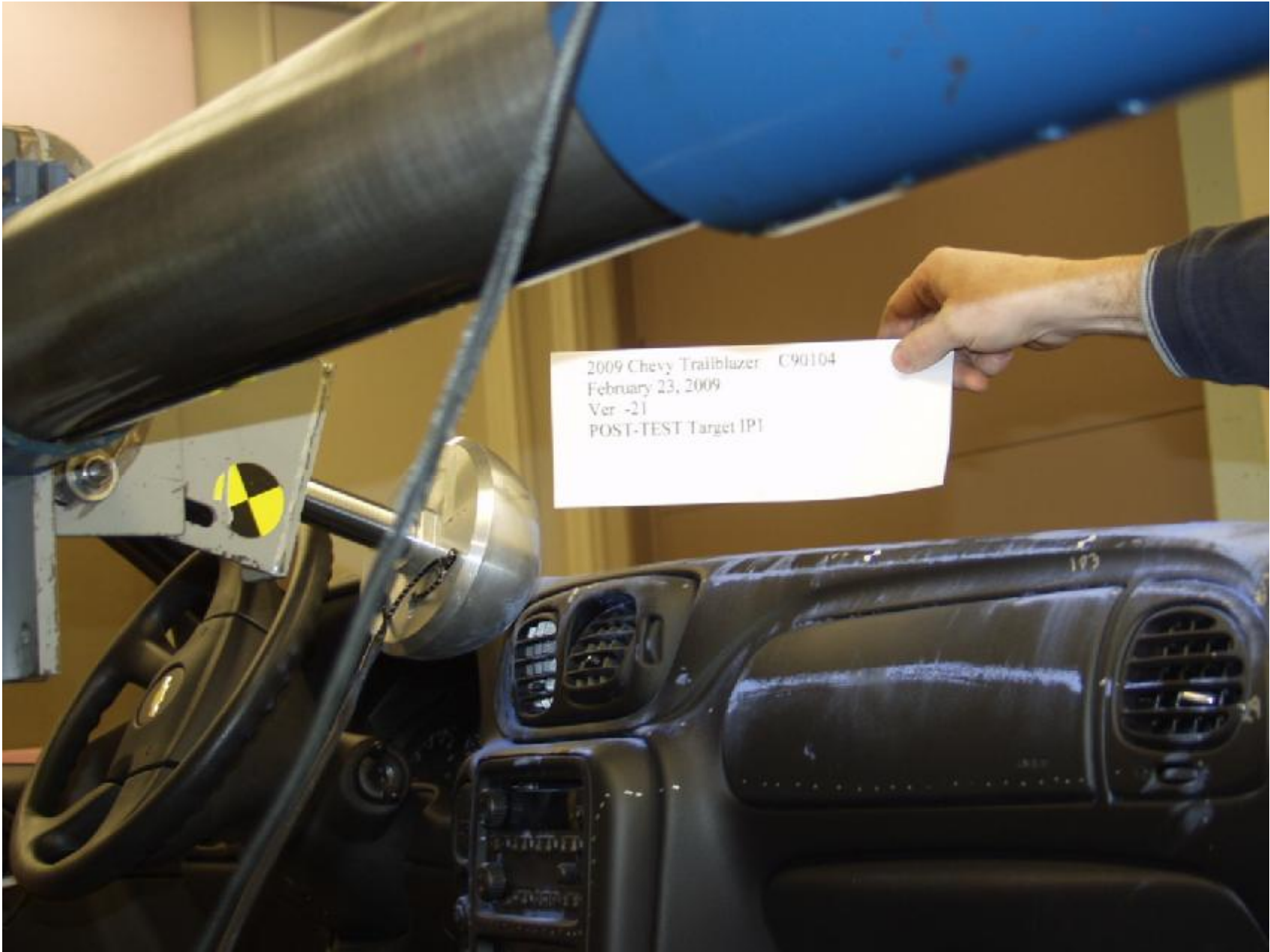
Figure A-15 : INSTRUMENT PANEL IMPACT #1 POST-TEST
