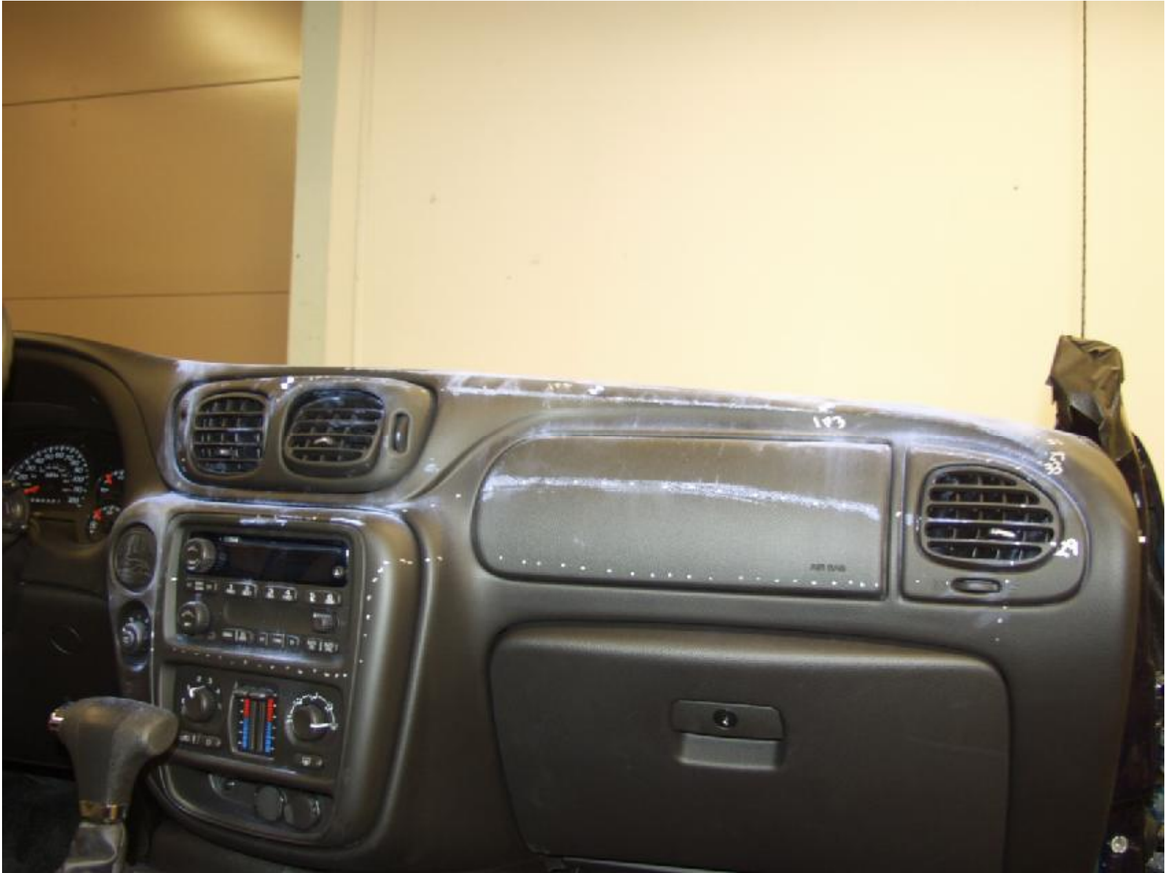
Figure A-13 : DELINEATED INSTRUMENT PANEL IMPACT ZONE POST-TEST
