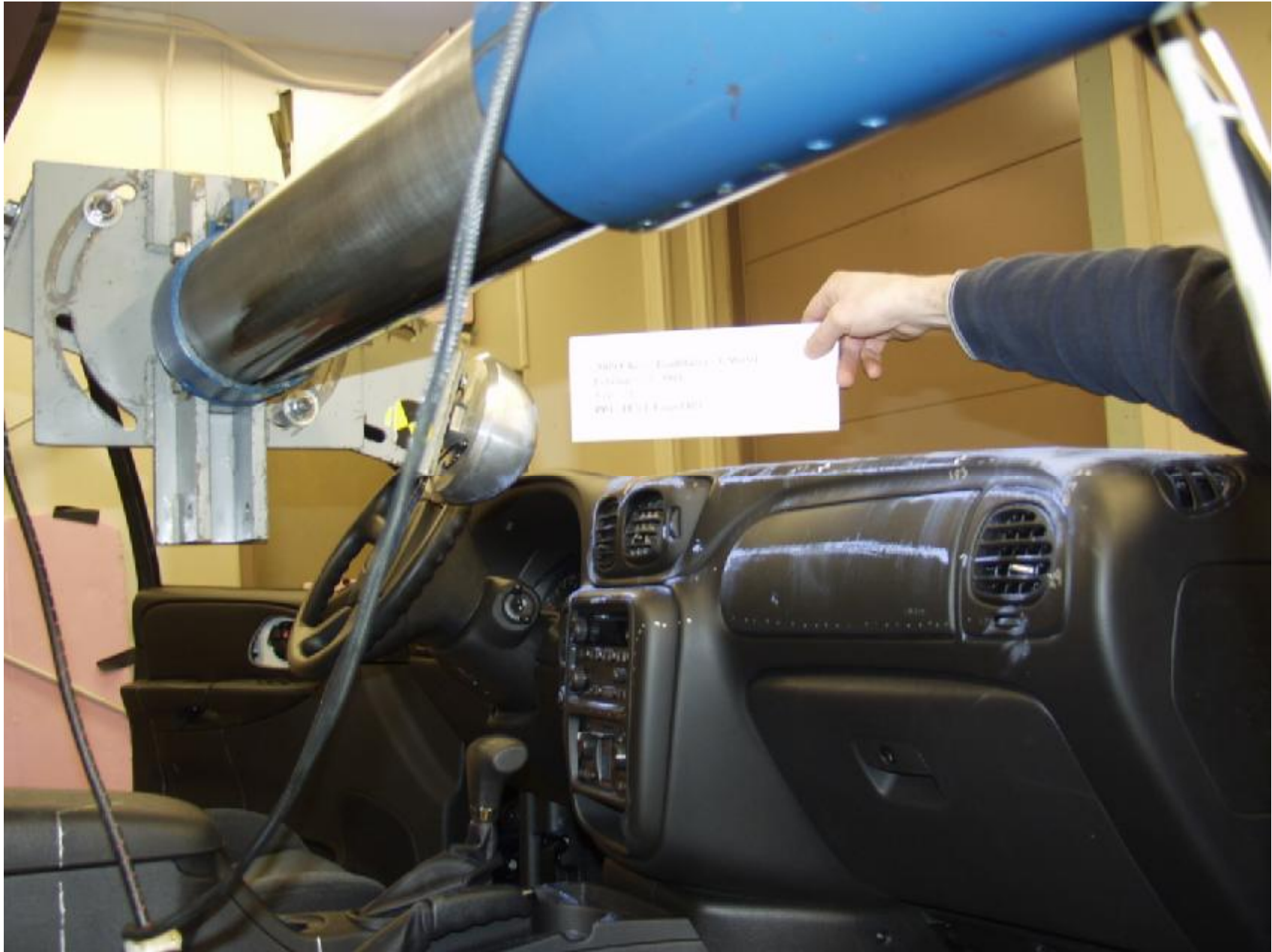
Figure A-14 : INSTRUMENT PANEL IMPACT #1 PRE-TEST
