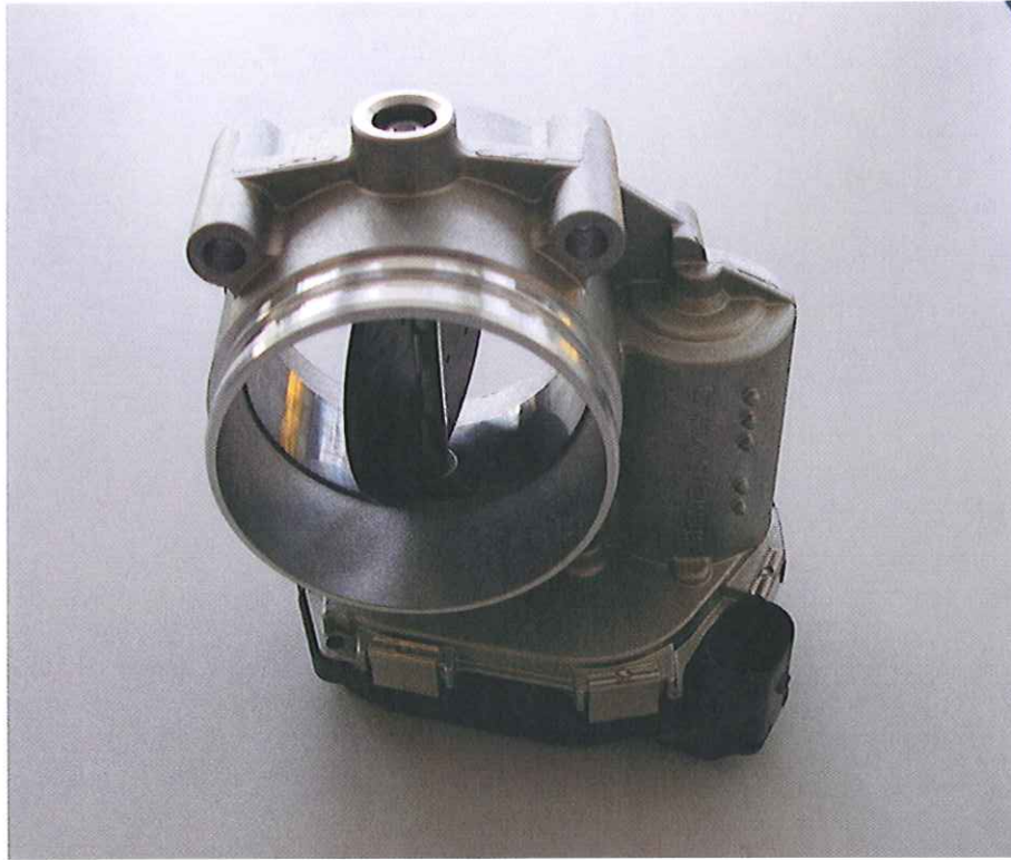
Figure 3: Throttle valve with return spring released (not actuated ► fully opened !)
