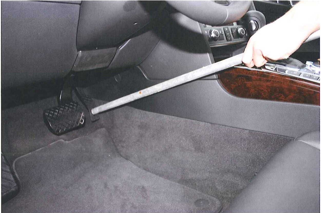
Figure 2: Operating means for accelerator pedal movement.
