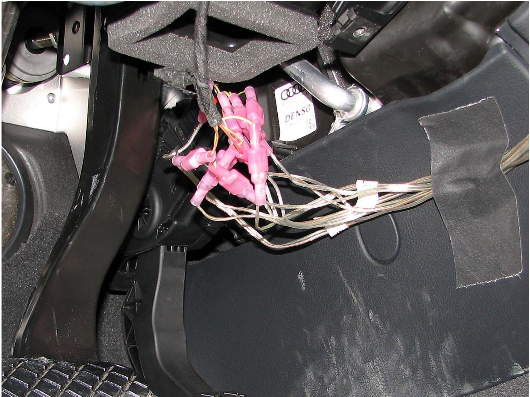
Figure A-12: Accelerator Pedal Test Setup
