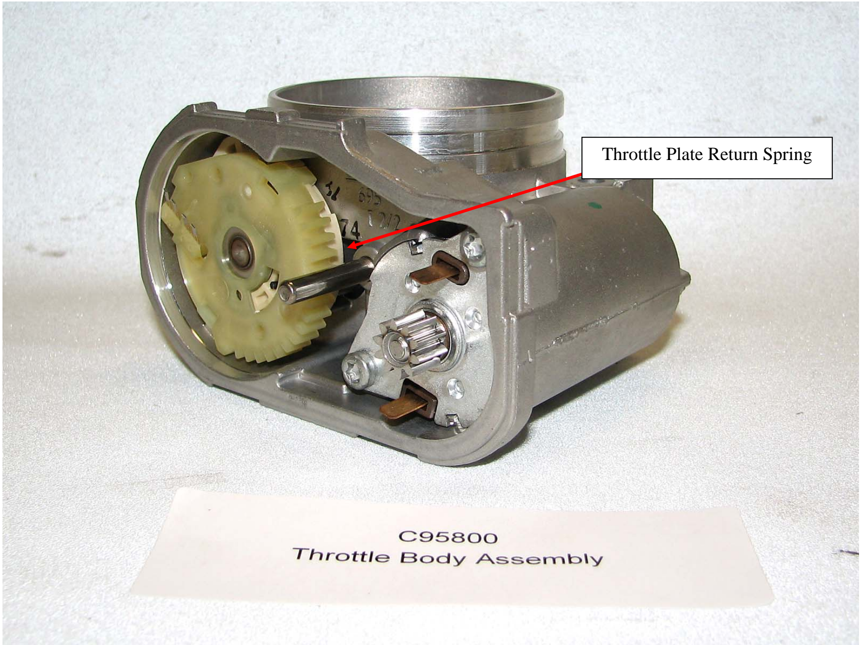
Figure A-8: Throttle Plate Return Spring
