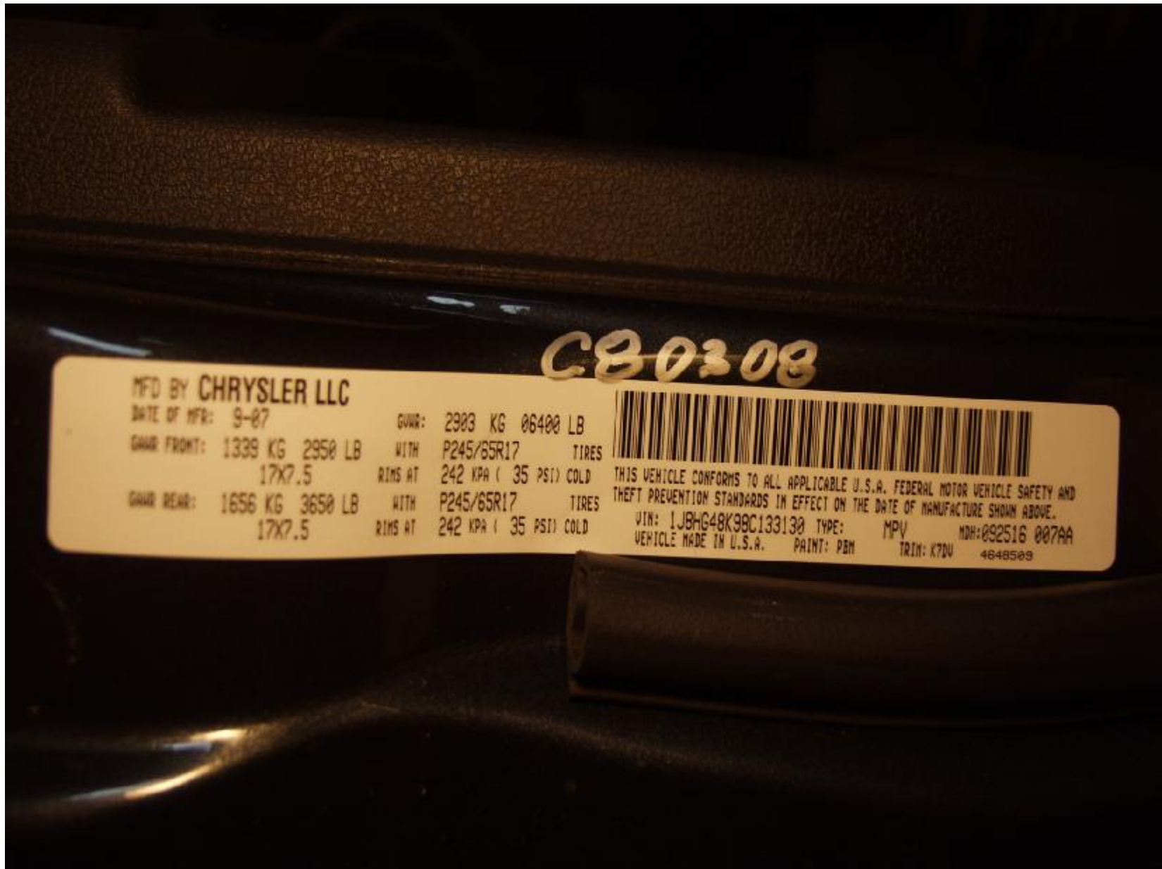
Figure 2: Vehicle Certification Placard
