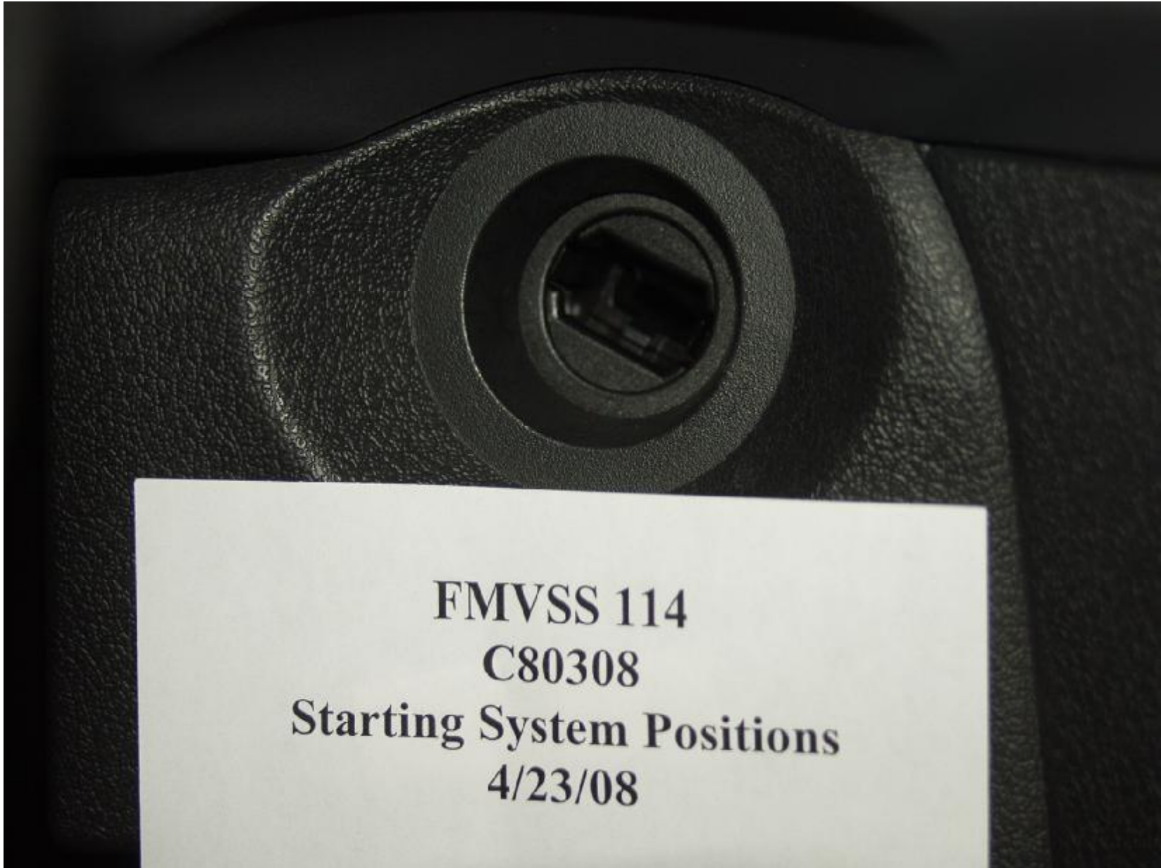
Figure 4: Close-Up of Ignition Switch
