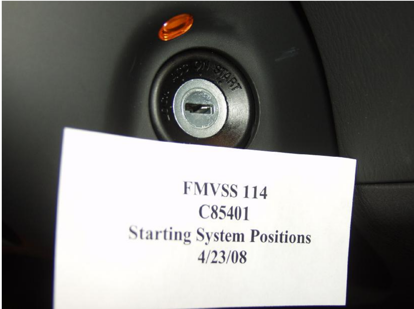
Figure 4: Close-Up of Ignition Switch
