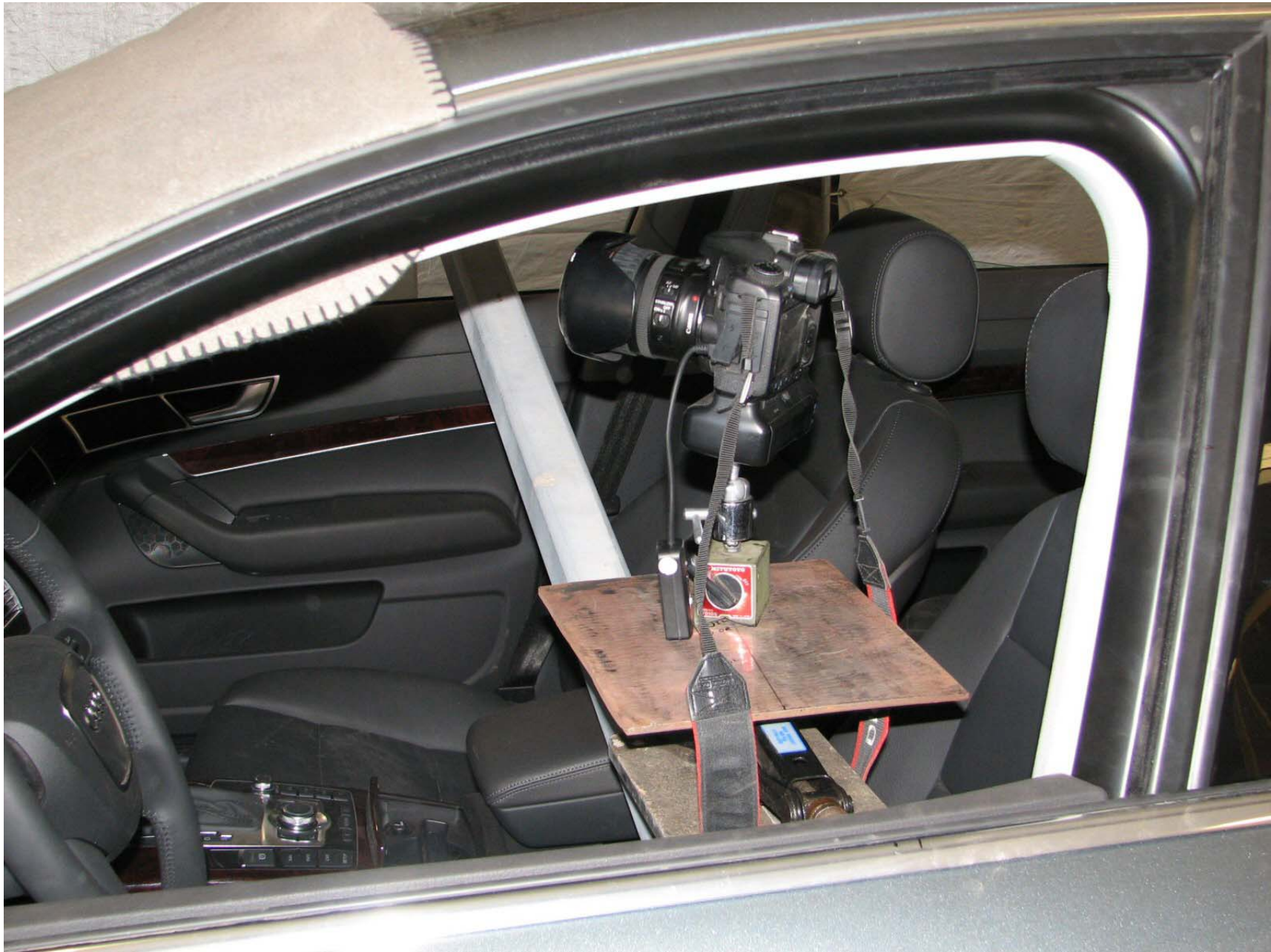
FIGURE 11:CAMERA SET-UP FOR PHOTOGRAPHING REFERENCE BOARD
