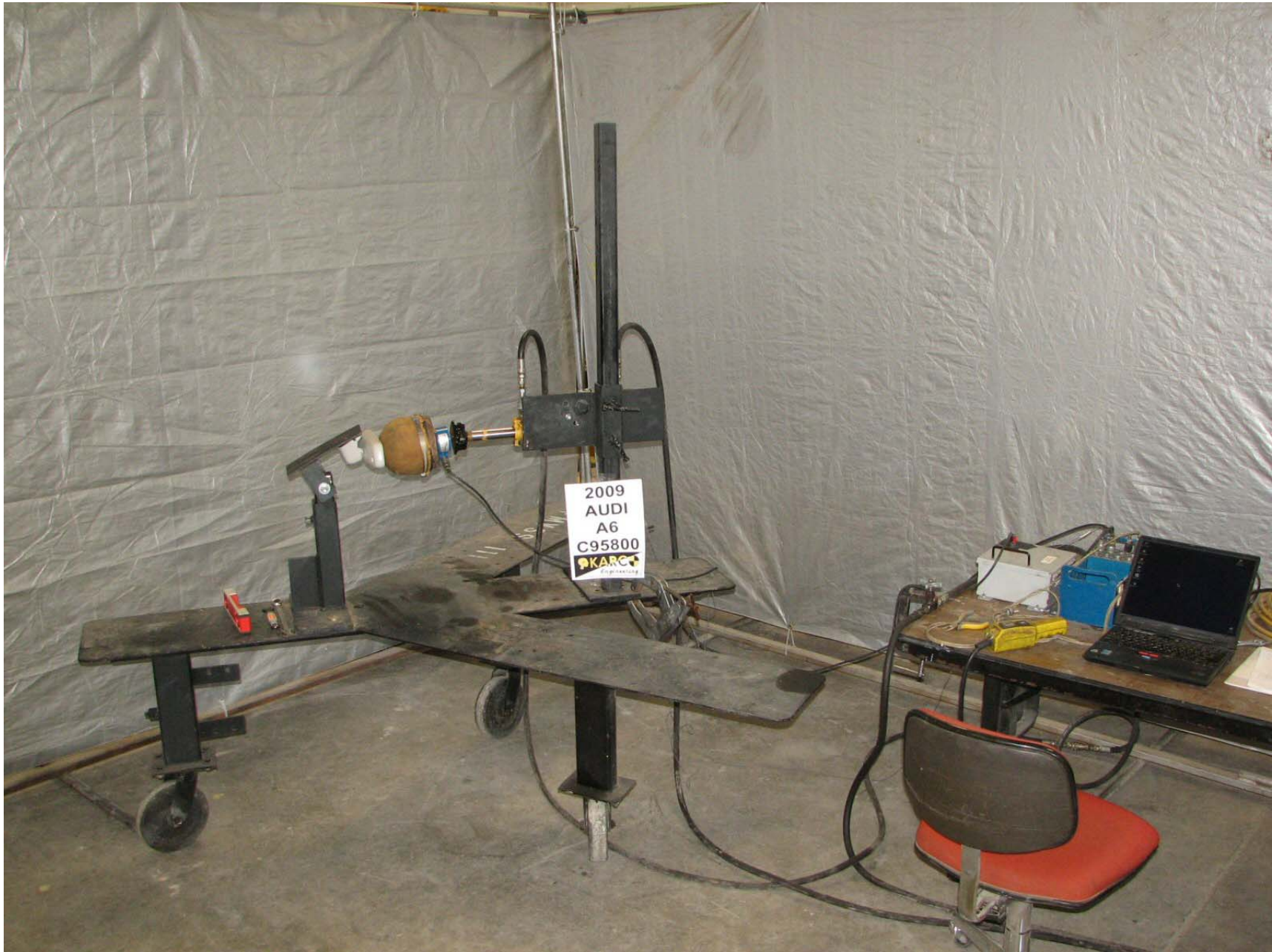
FIGURE 12: OVERALL SET-UP AND INSTRUMENTATION FOR MIRROR BREAK- AWAY TEST
