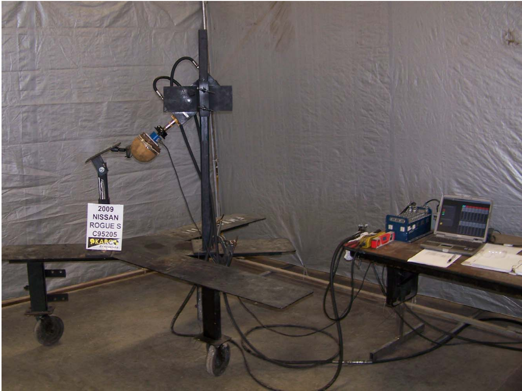
2009 NISSAN ROGUE S NHTSA NO. C95205 FMVSS NO. 111 FIGURE 12: OVERALL SET-UP AND INSTRUMENTATION FOR MIRROR BREAK- AWAY TEST
