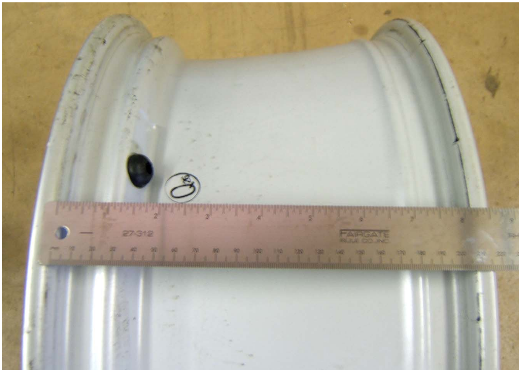
FIGURE 5.10 RIM CONTOUR FOR FULL WIDTH OF CROSS SECTION
