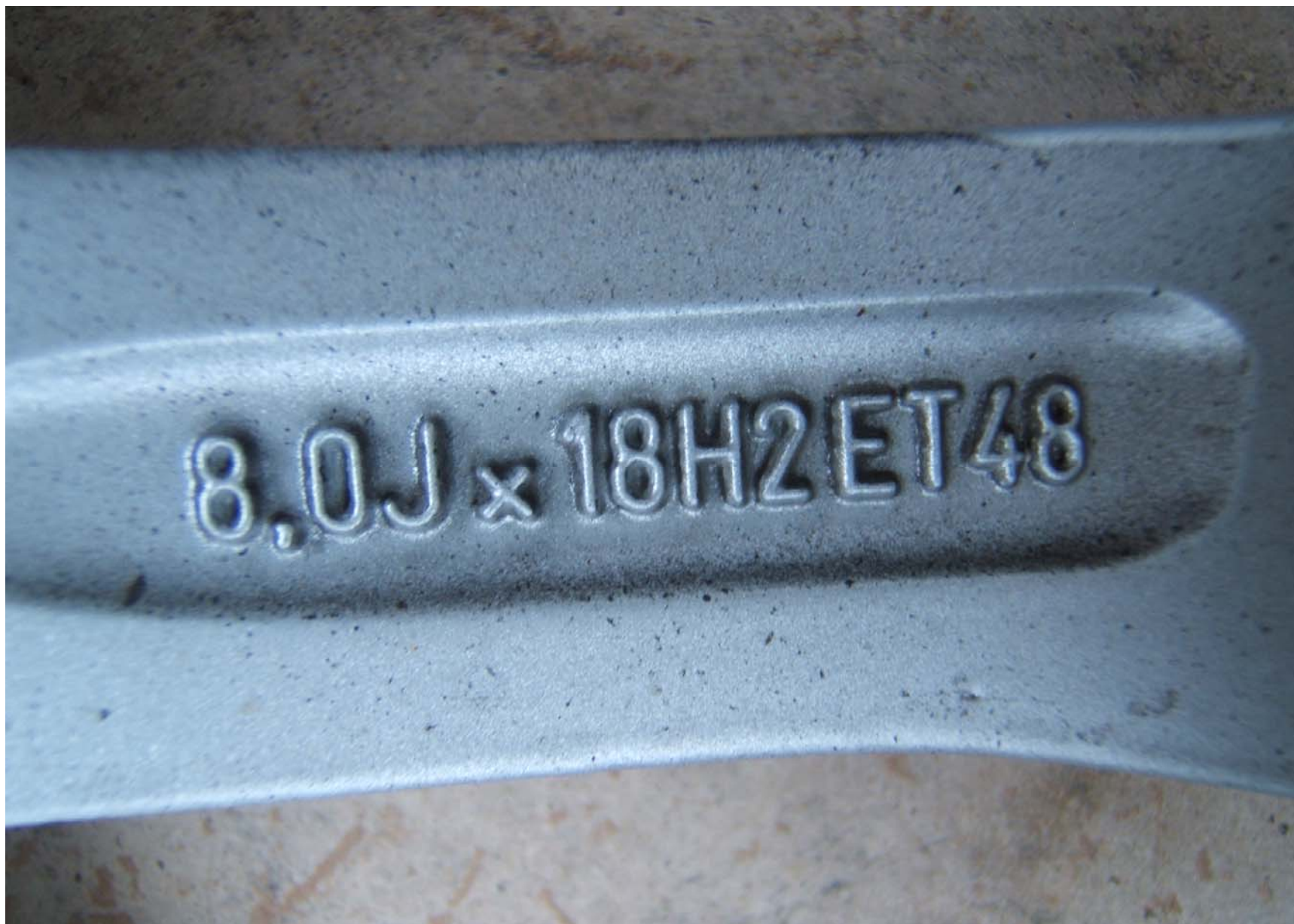
FIGURE 5.11 RIM SHOWING SIZE AND OTHER RIM MARKINGS
