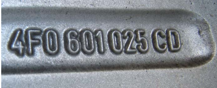
FIGURE 5.14 RIM SHOWING OTHER RIM MARKINGS
