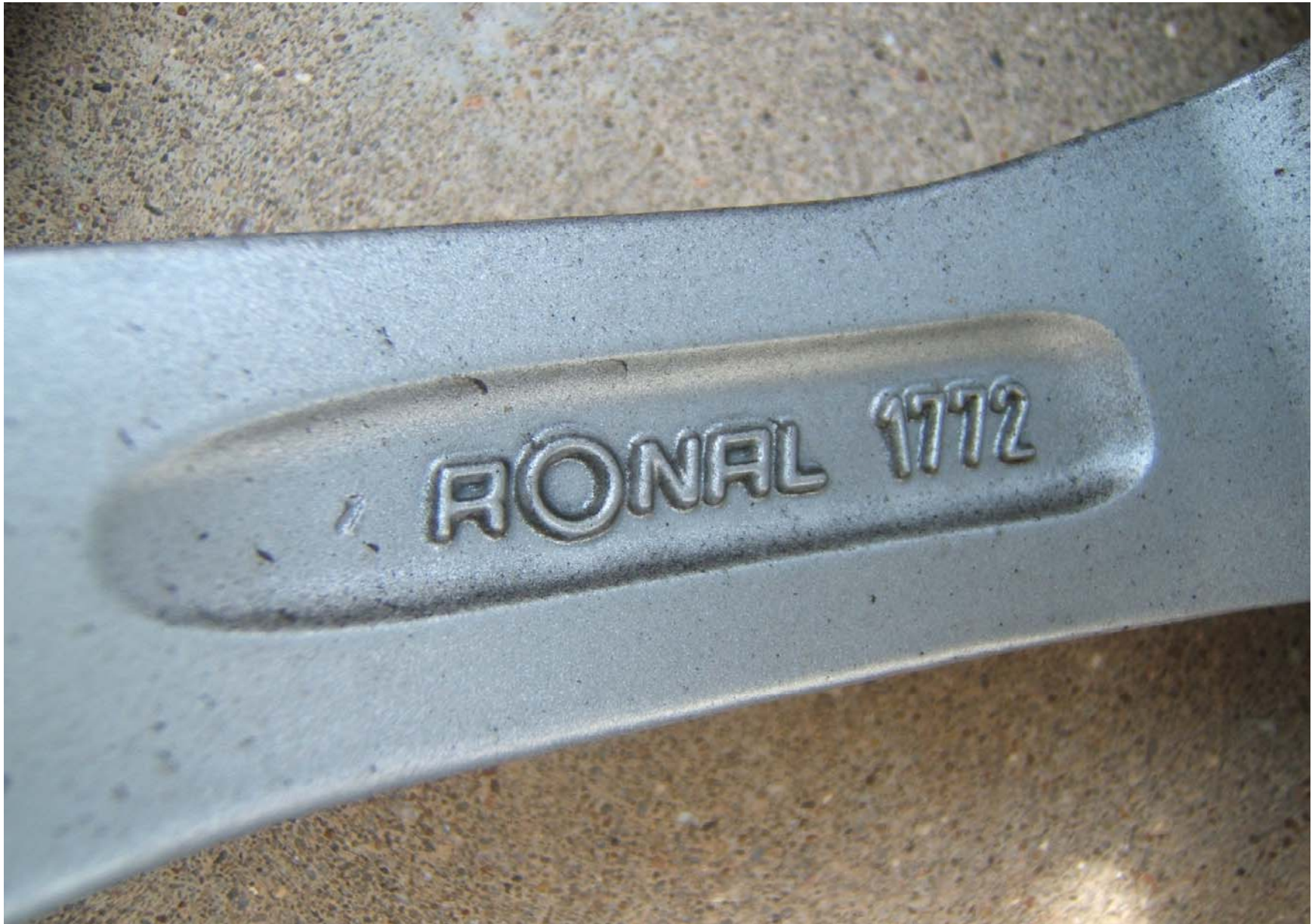
FIGURE 5.12 RIM SHOWING MANUFACTURER'S SYMBOL AND OTHER RIM MARKING
