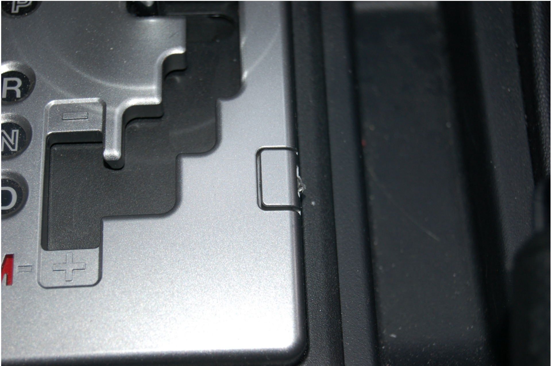
FIGURE 5.7 DEVICE WHICH ALLOWS MOVING GEAR SELECTOR OUT OF PARK POSITION
