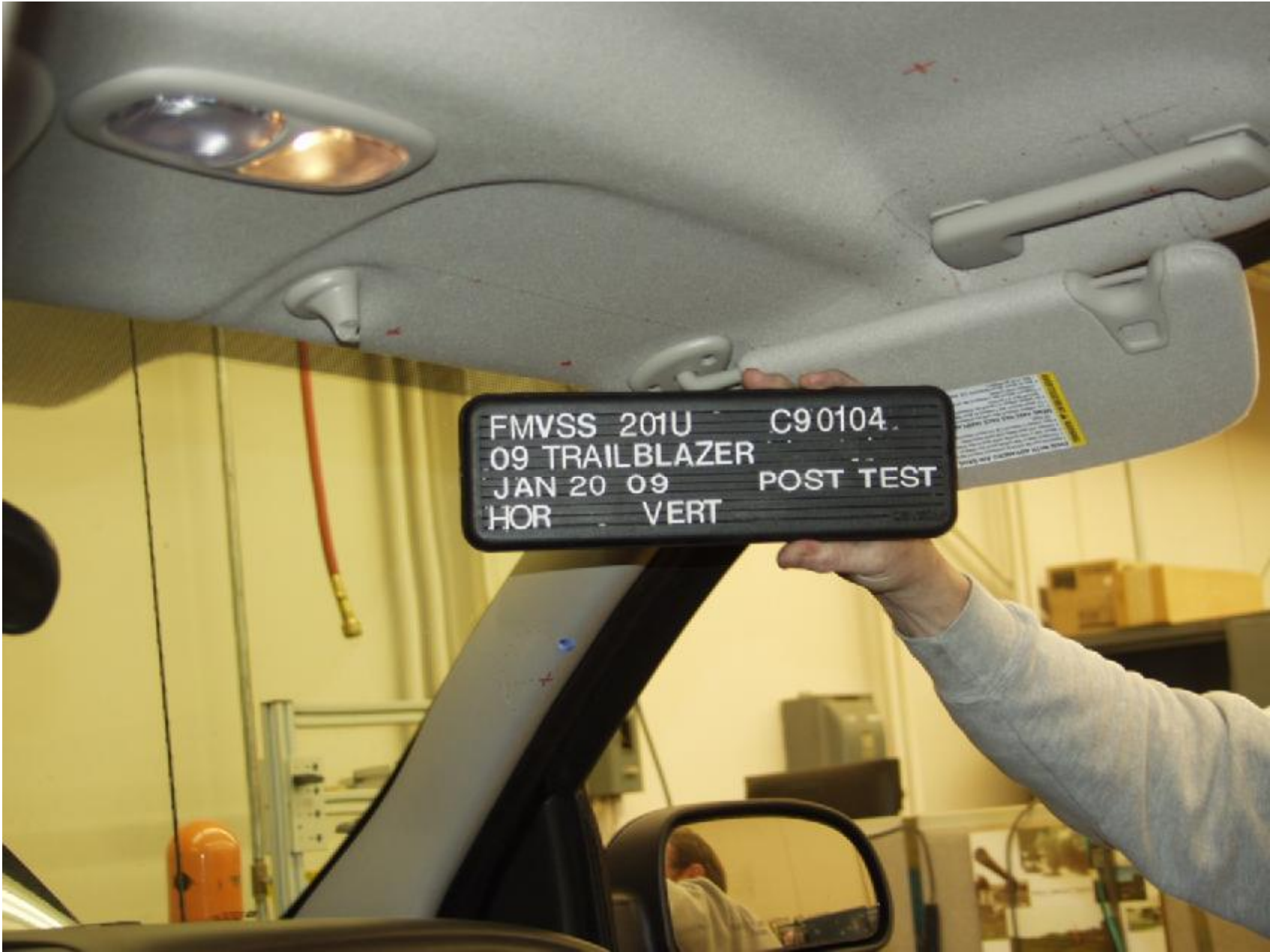
Figure A-23 : POST-TEST PASSENGER SIDE FRONT HEADER
