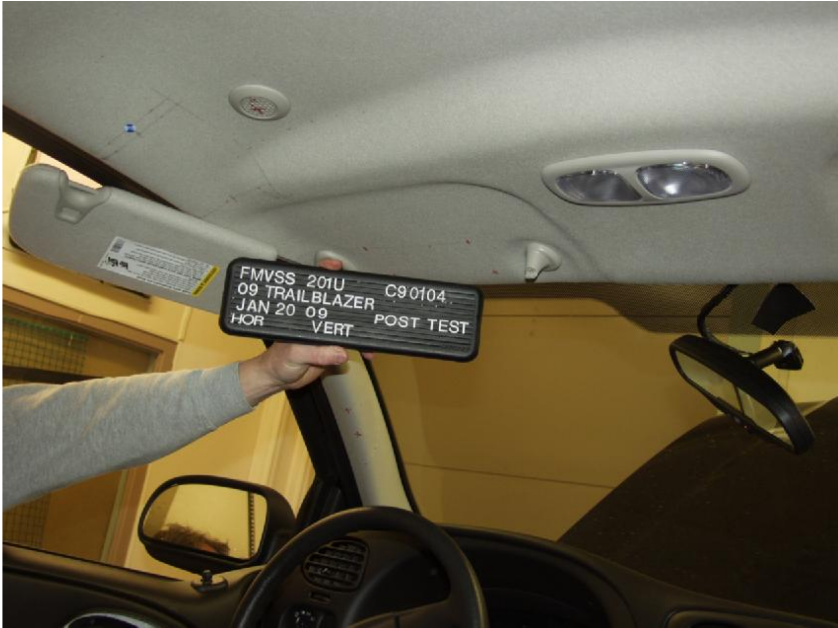
Figure A-18 : POST-TEST DRIVER SIDE FRONT HEADER
