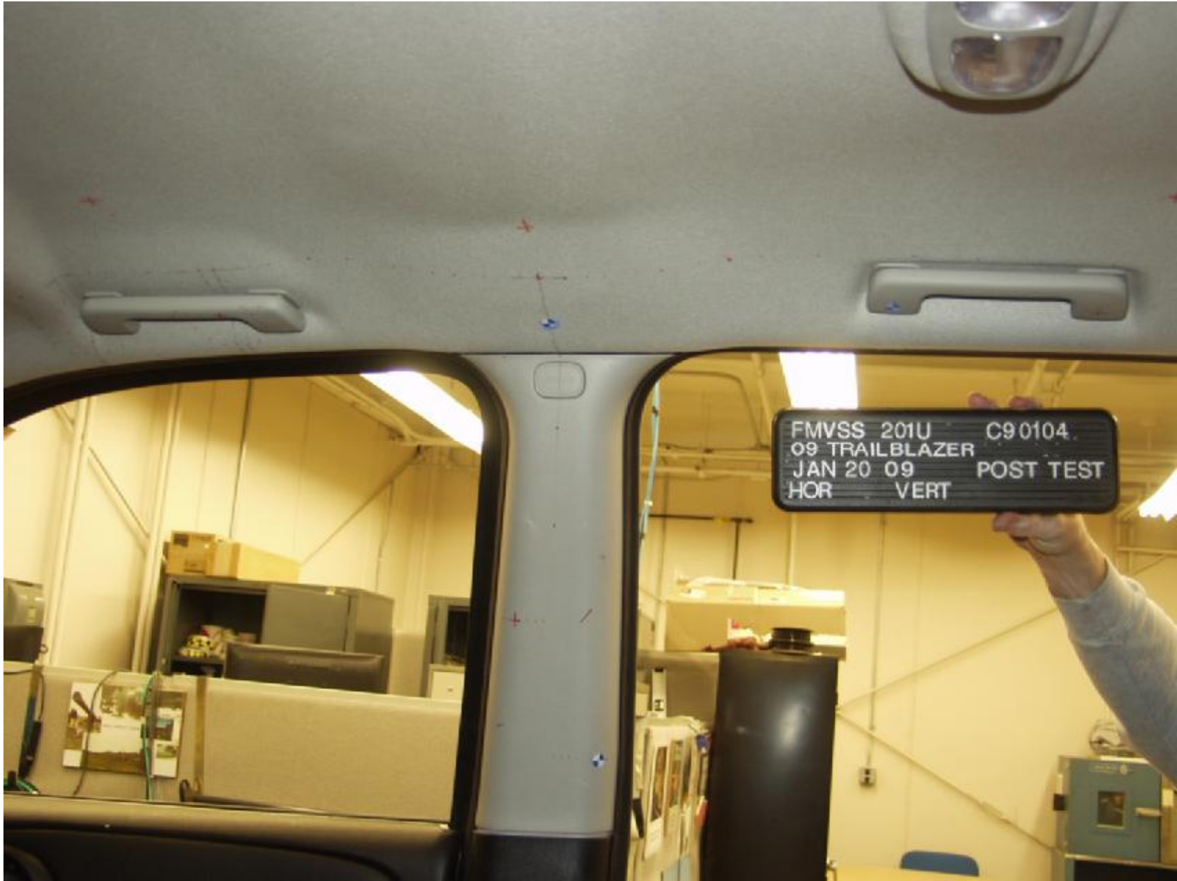
Figure A-25 : POST-TEST PASSENGER SIDE B-PILLAR
