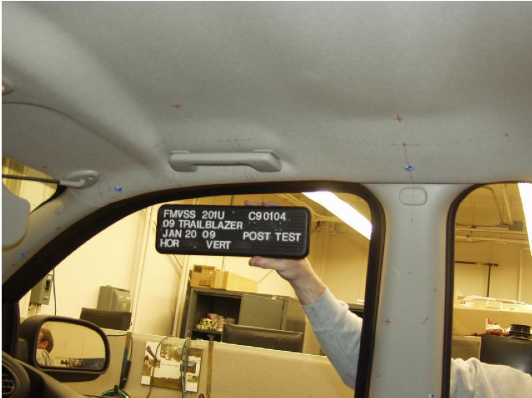
Figure A-24 : POST-TEST PASSENGER SIDE SIDE RAIL
