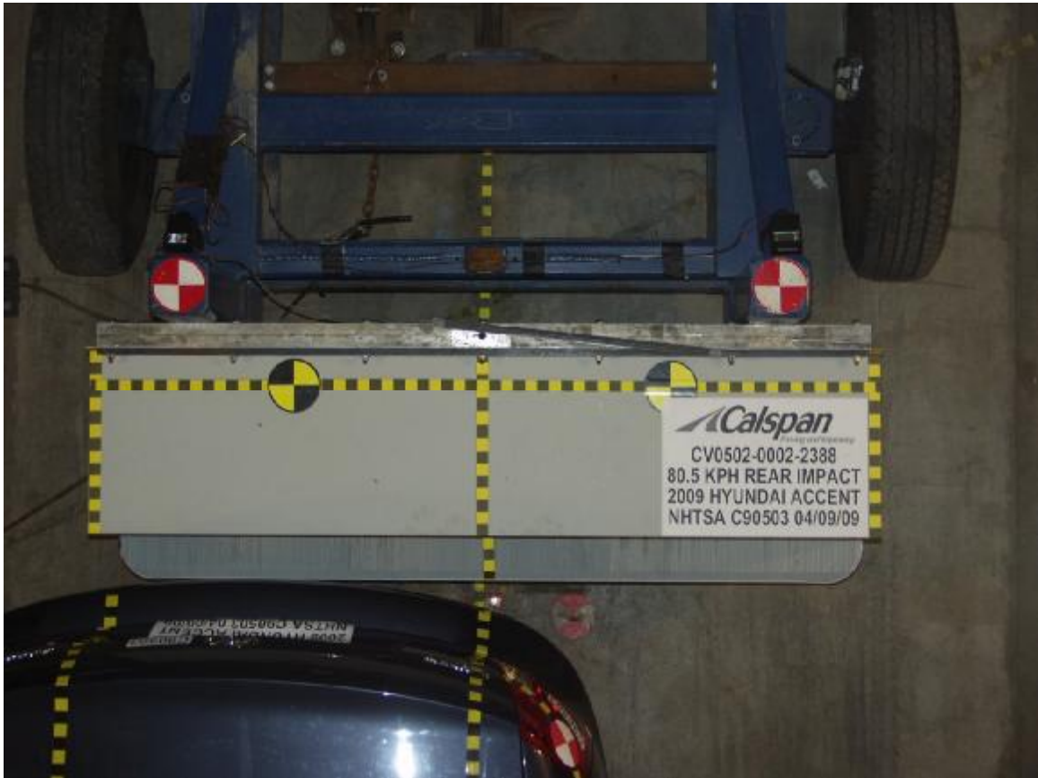
Figure A-25: Pre-Test MDB Top View
