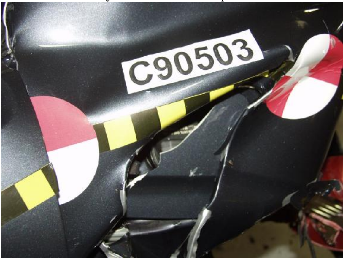
Figure A-36: Post-Test Fuel Filler Cap View
