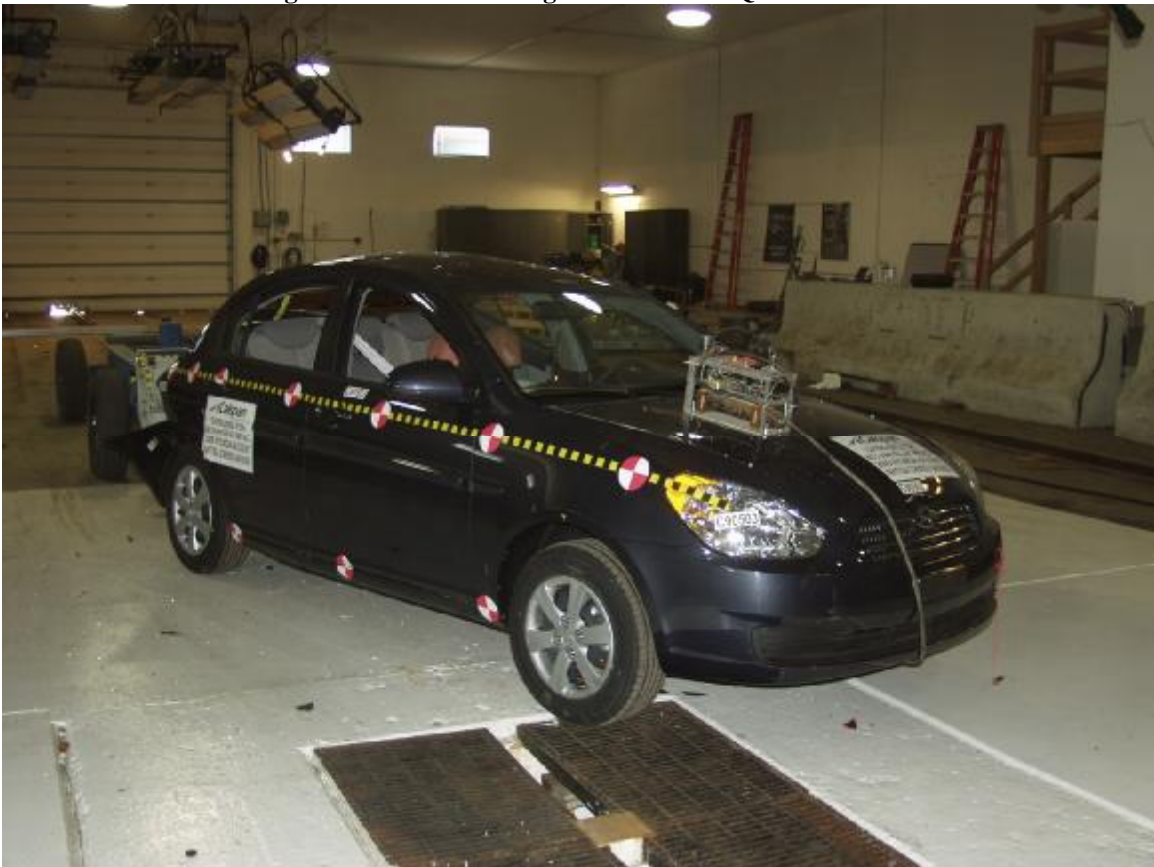
Figure A-12: Post-Test Right Front Three-Quarter View
