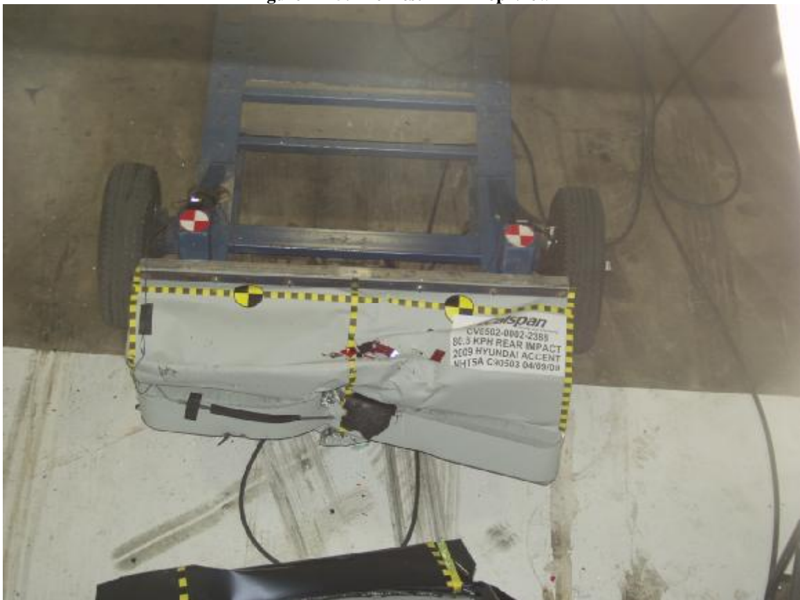
Figure A-26: Post-Test MDB Top View
