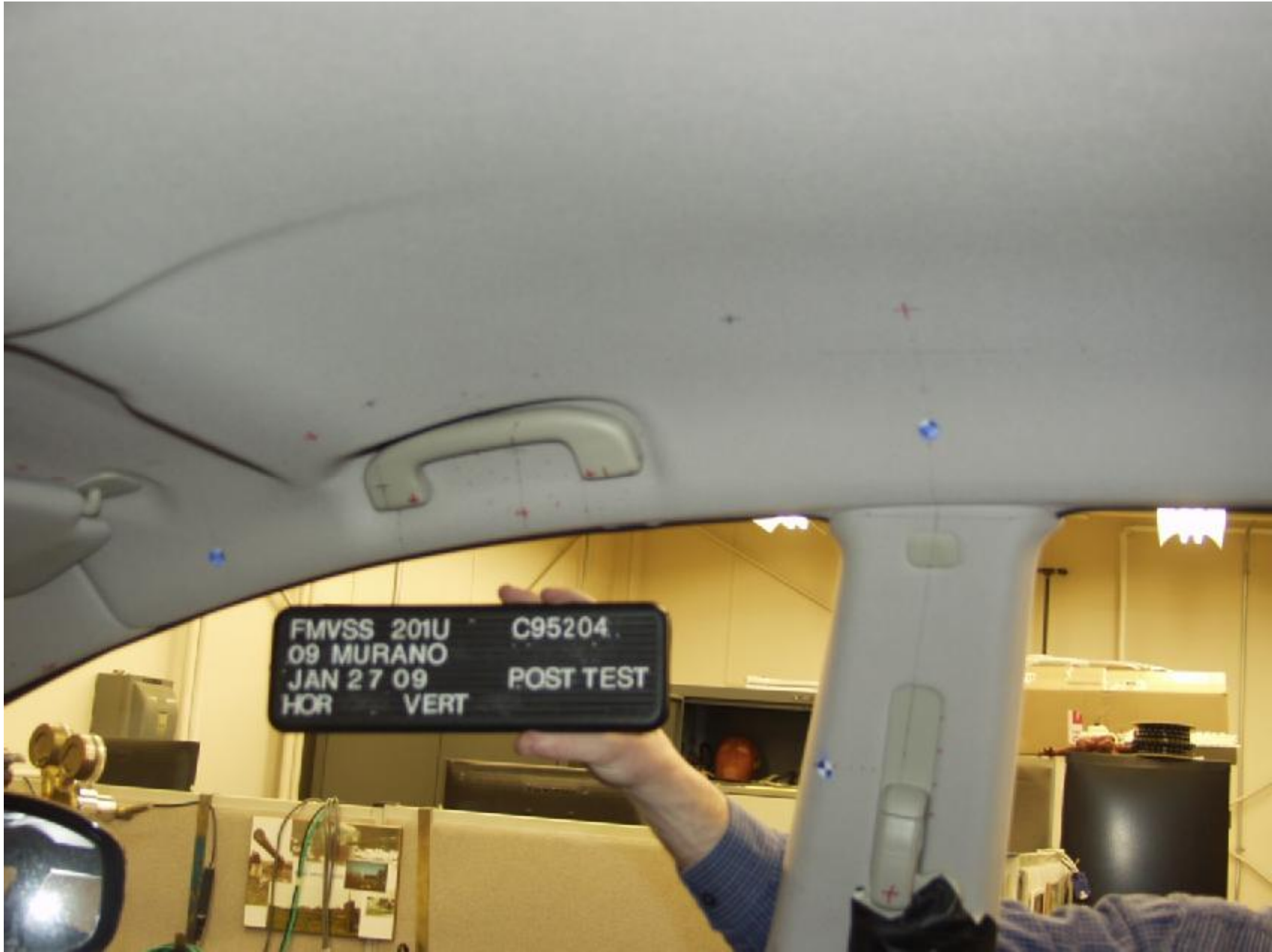
Figure A-24 : POST-TEST PASSENGER SIDE SIDE RAIL
