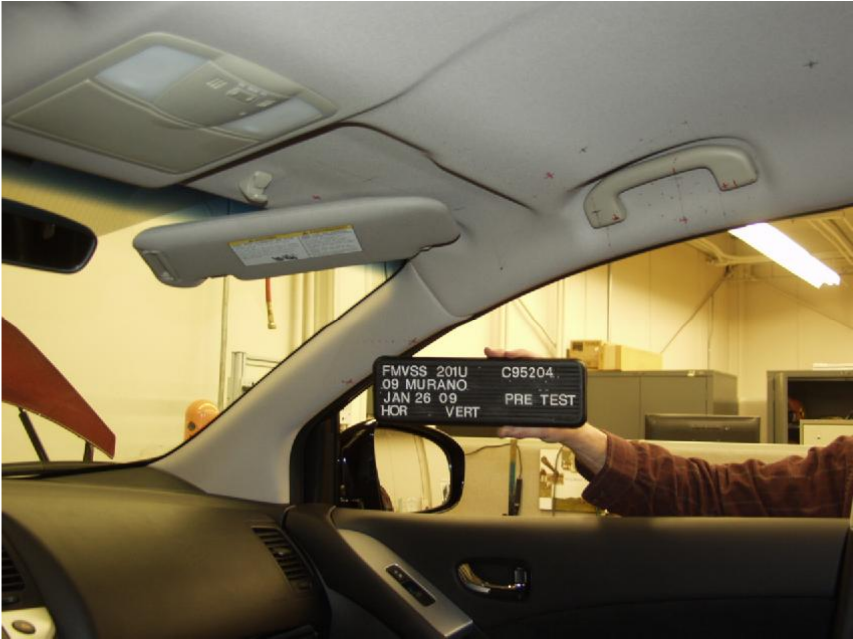
Figure A-12 : PRE-TEST PASSENGER SIDE A-PILLAR
