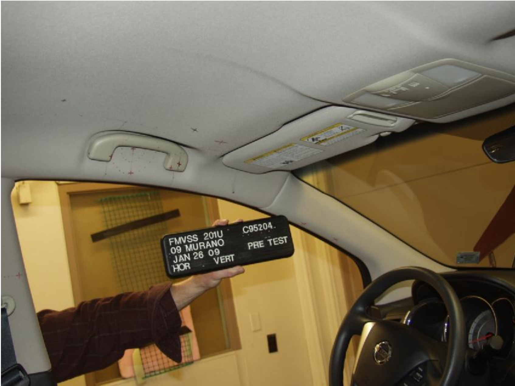
Figure A-7 : PRE-TEST DRIVER SIDE A-PILLAR
