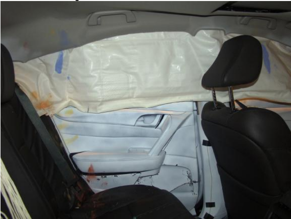
Figure A-46: Post-Test Left Rear Interior Trim
