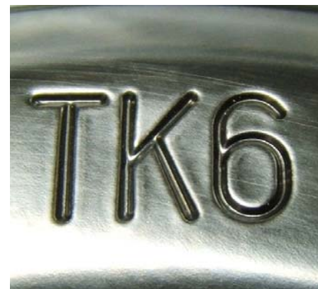
FIGURE 5.11 RIGHT FRONT RIM SHOWING LETTER DESIGNATION FOR SOURCE OF PUBLISHED DIMENSIONS, SIZE, DOT SYMBOL, MANUFACTURER'S SYMBOL, DATE OF MANUFACTURE, AND OTHER RIM MARKINGS
