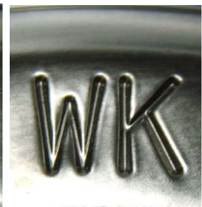
FIGURE 5.11 RIGHT FRONT RIM SHOWING LETTER DESIGNATION FOR SOURCE OF PUBLISHED DIMENSIONS, SIZE, DOT SYMBOL, MANUFACTURER'S SYMBOL, DATE OF MANUFACTURE, AND OTHER RIM MARKINGS
