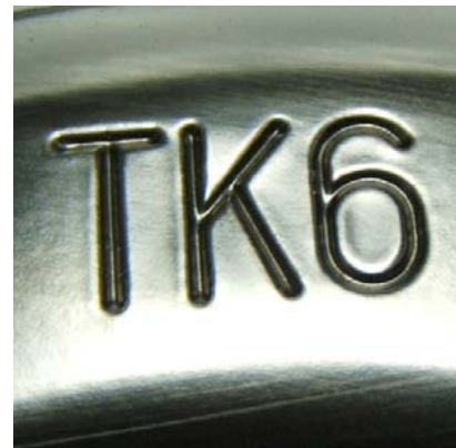
LEFT REAR RIM SHOWING LETTER DESIGNATION FOR SOURCE OF PUBLISHED DIMENSIONS, SIZE, DOT SYMBOL, MANUFACTURER'S SYMBOL, DATE OF MANUFACTURE, AND OTHER RIM MARKINGS
