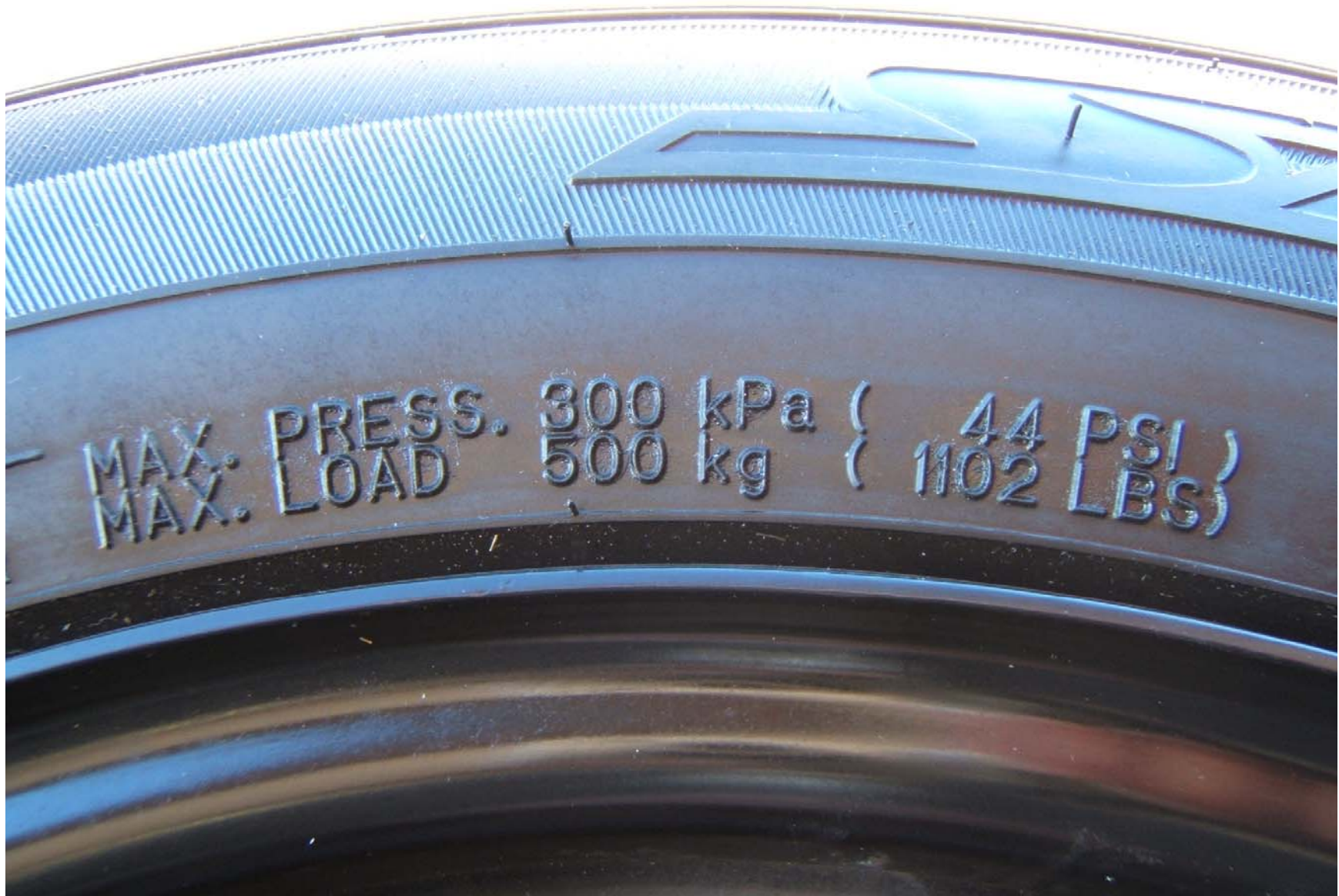
FIGURE 5.8 TIRE SHOWING MAX INFLATION PRESSURE AND MAX LOAD RATING
