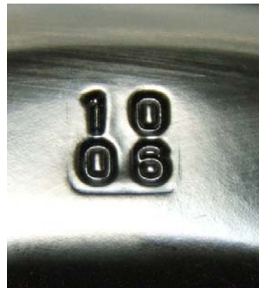
LEFT REAR RIM SHOWING LETTER DESIGNATION FOR SOURCE OF PUBLISHED DIMENSIONS, SIZE, DOT SYMBOL, MANUFACTURER'S SYMBOL, DATE OF MANUFACTURE, AND OTHER RIM MARKINGS
