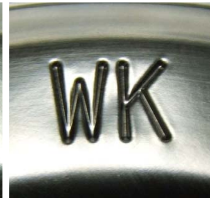
LEFT REAR RIM SHOWING LETTER DESIGNATION FOR SOURCE OF PUBLISHED DIMENSIONS, SIZE, DOT SYMBOL, MANUFACTURER'S SYMBOL, DATE OF MANUFACTURE, AND OTHER RIM MARKINGS
