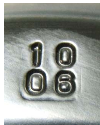
FIGURE 5.11 RIGHT FRONT RIM SHOWING LETTER DESIGNATION FOR SOURCE OF PUBLISHED DIMENSIONS, SIZE, DOT SYMBOL, MANUFACTURER'S SYMBOL, DATE OF MANUFACTURE, AND OTHER RIM MARKINGS
