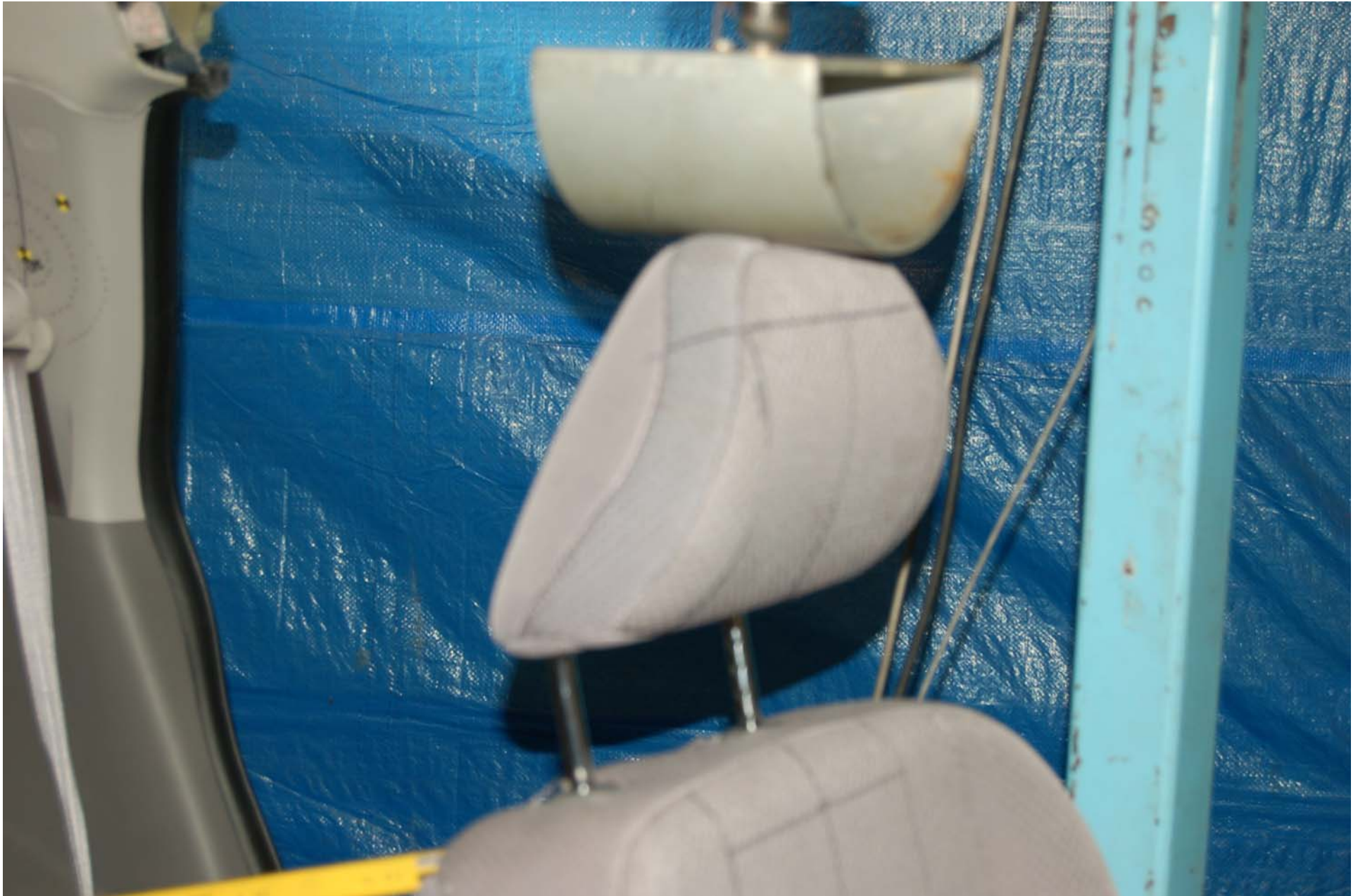
FIGURE 5.23 HEAD RESTRAINT WITH 50 N LOAD FOR HEIGHT RETENTION
