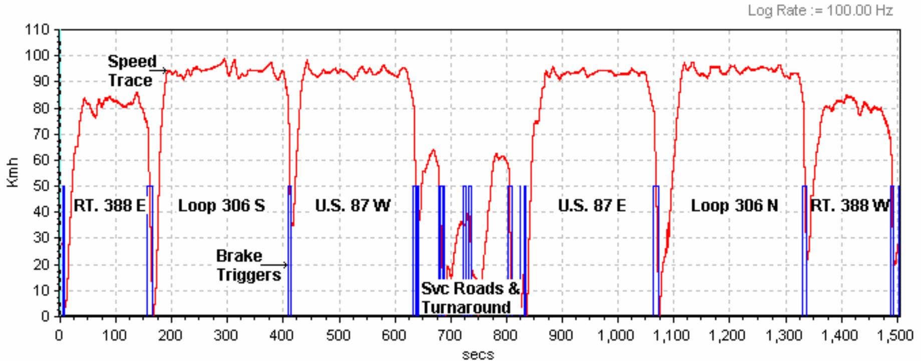
LF Detection Phase: Telltale illumination in 45.5 seconds. Driving above 50 km/h (31 mph) was not required.
