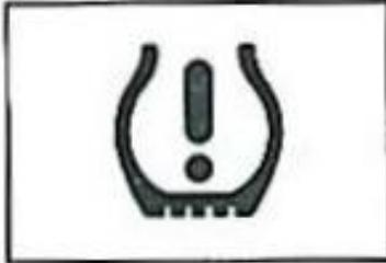
For vehicles with a tire pressure light, this light comes on briefly when the engine is started.
