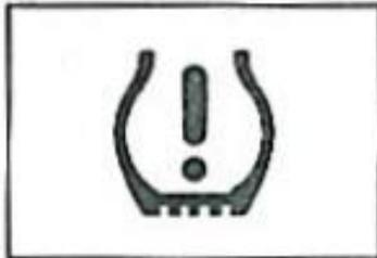
When a low tire pressure condition is detected, the TPMS illuminates the low tire pressure warning light located on the instrument panel cluster.
