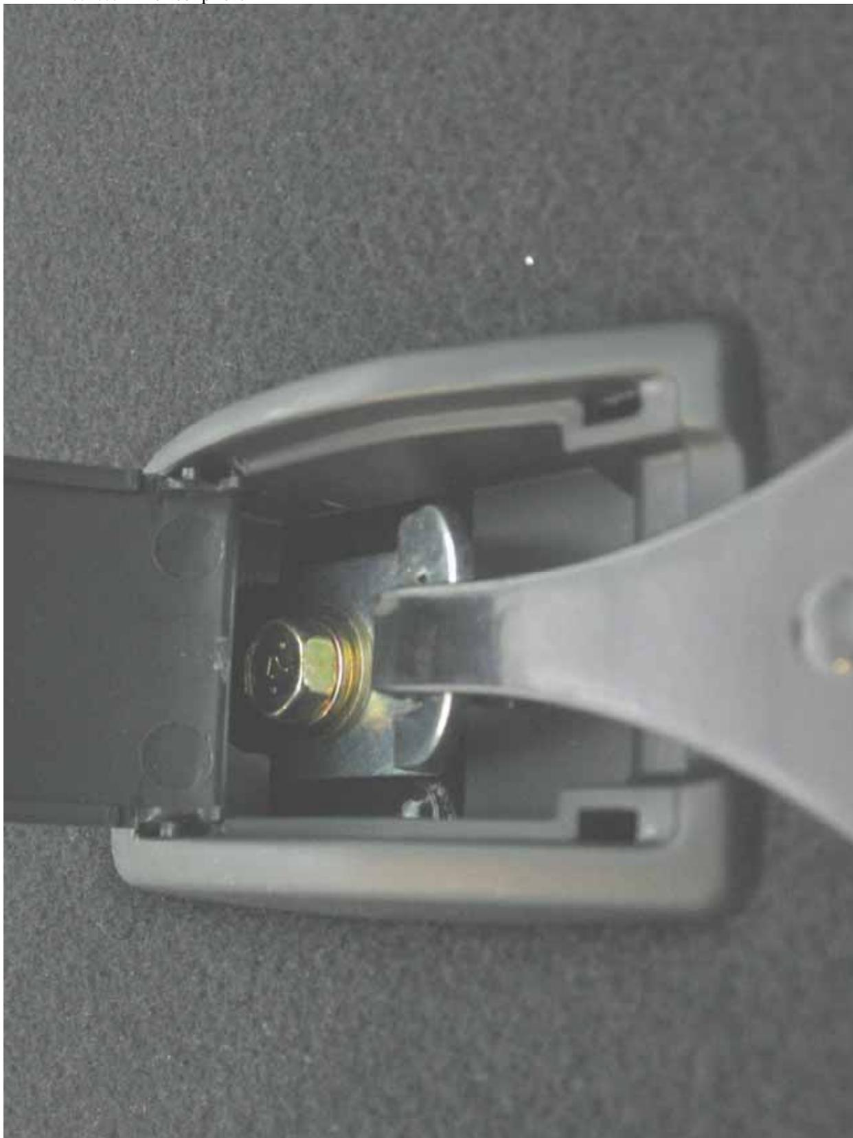
6.11 Post-test condition of each child restraint anchorage system
