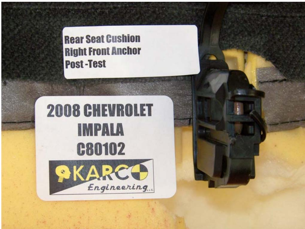
FIGURE 132. Seat Cushion Anchor, P3, Post-Test
