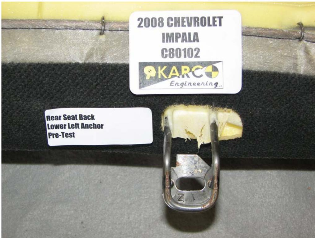
FIGURE 117. Seat Back Anchor, P4, Pre-Test
