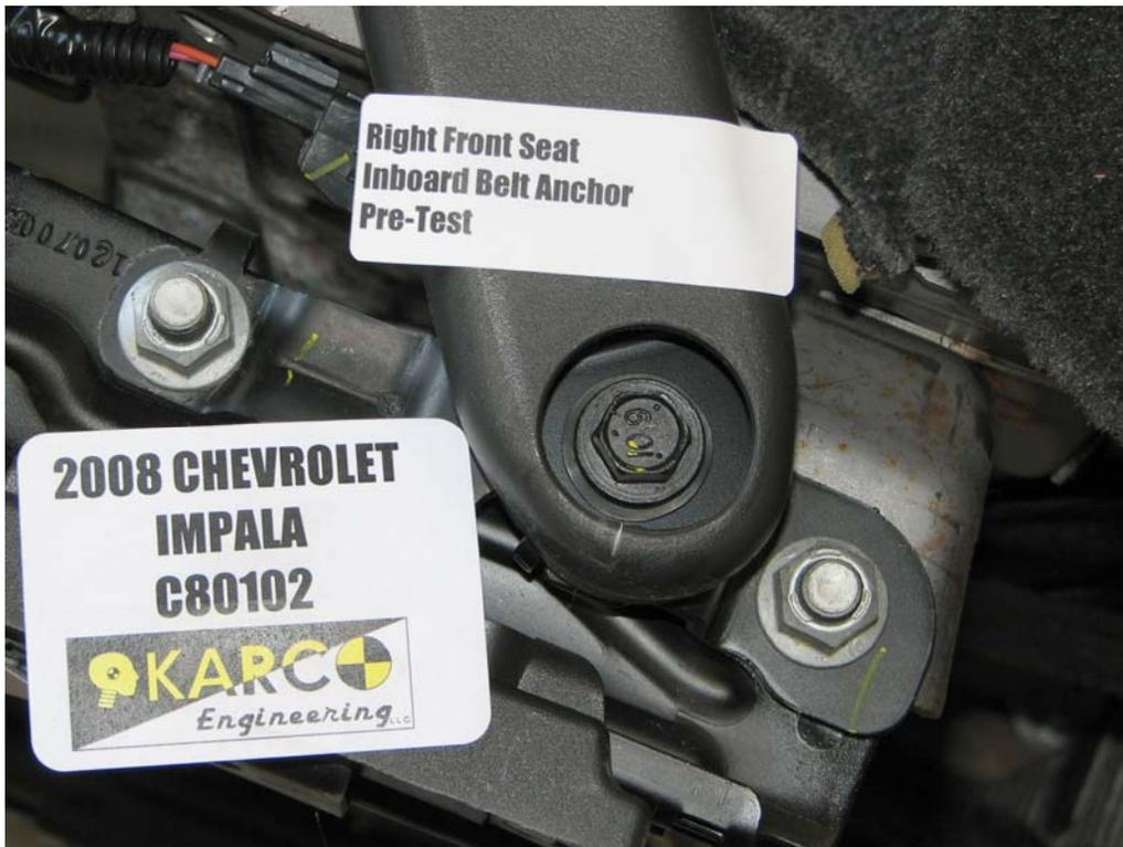
FIGURE 93. Belt Anchor, P2, Pre-Test
