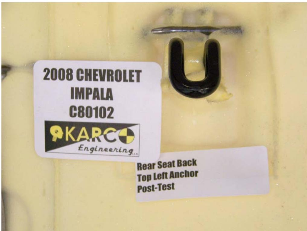
FIGURE 102. Seat Back Anchor, P4, Post-Test
