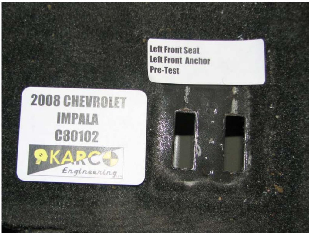
FIGURE 43. Floor Pan Anchor, P1, Pre-Test
