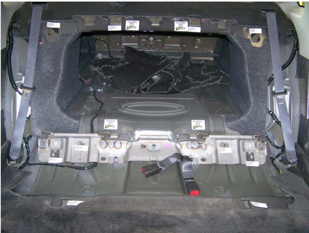
FIGURE 96. Floor Pan Anchors, P3 & P4 Overall, Post-Test
