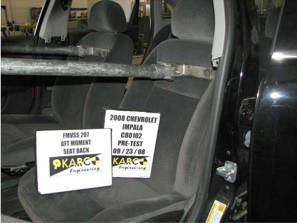
FIGURE 11. Aft Moment on Seat Back, P1, Pre-Test
