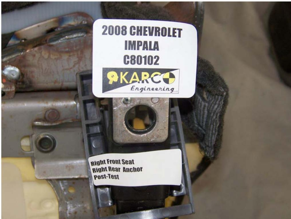
FIGURE 86. Seat Anchor, P2, Post-Test
