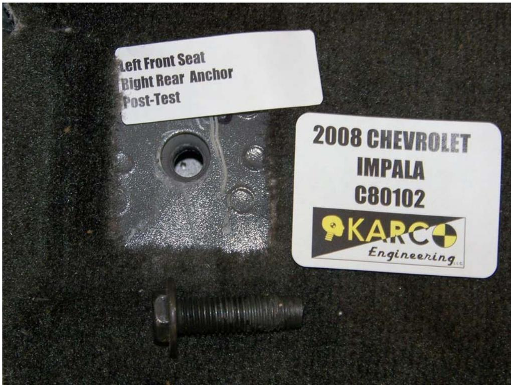
FIGURE 56. Floor Pan Anchor, P1, Post-Test
