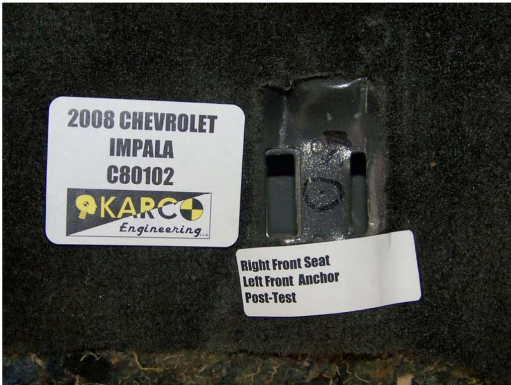
FIGURE 72. Floor Pan Anchor, P2, Post-Test
