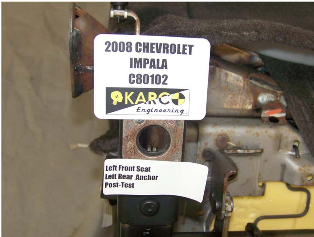
FIGURE 54. Seat Anchor, P1, Post-Test
