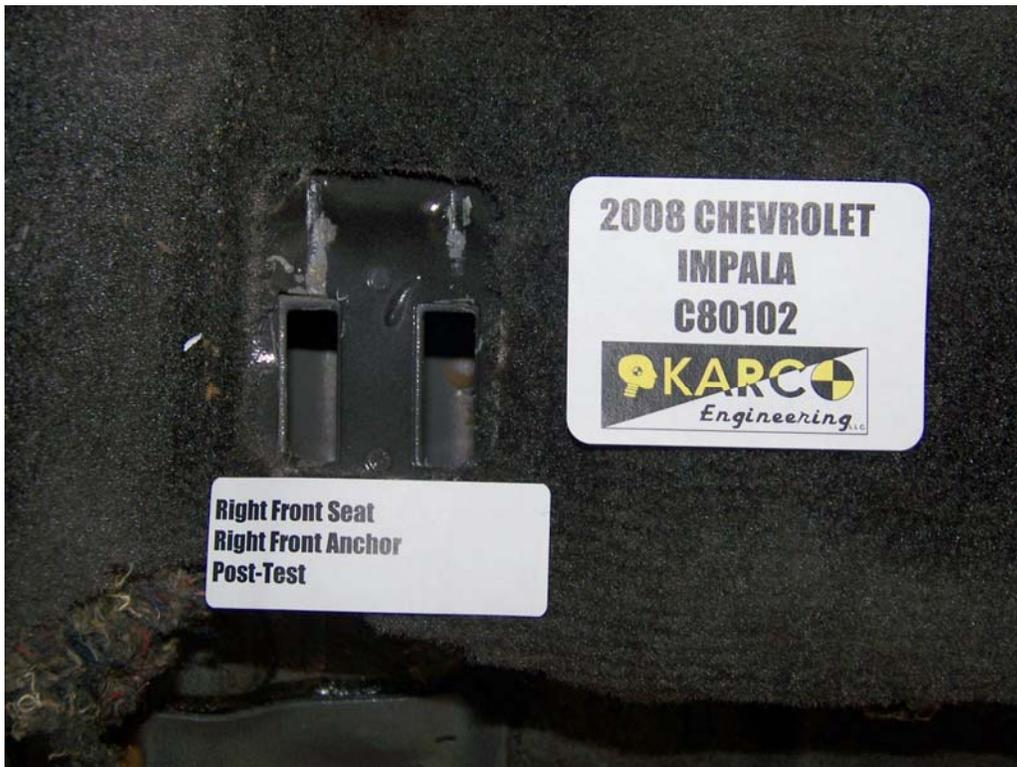
FIGURE 76. Floor Pan Anchor, P2, Post-Test
