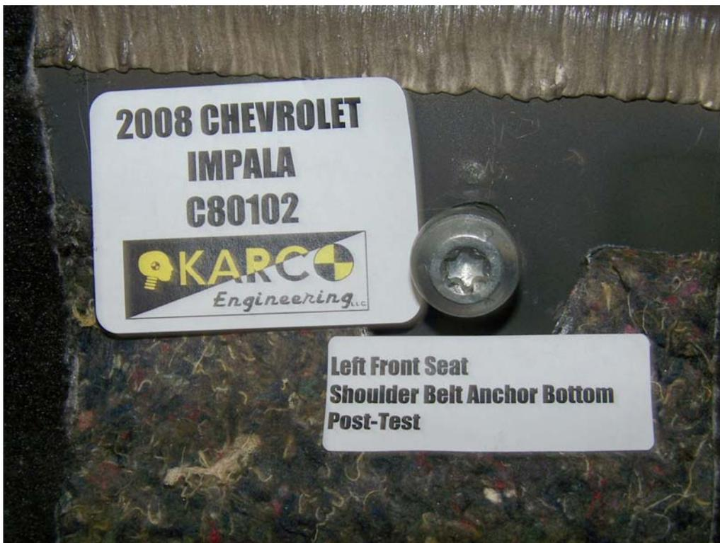
FIGURE 62. Shoulder Belt Anchor, P1, Post-Test
