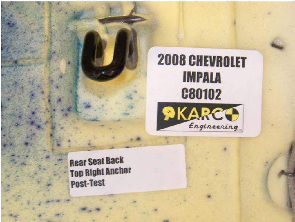
FIGURE 114. Seat Back Anchor, P3, Post-Test
