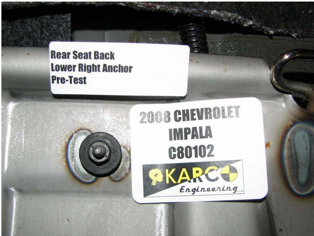
FIGURE 119. Floor Pan Anchor, P3, Pre-Test
