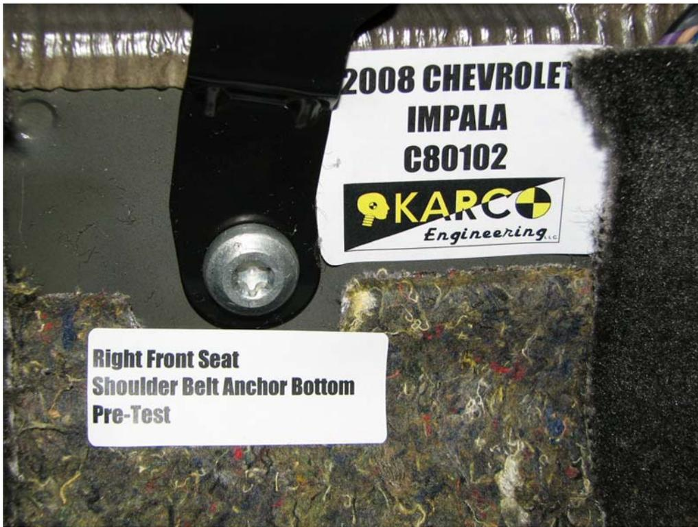
FIGURE 89. Shoulder Belt Anchor, P2, Pre-Test
