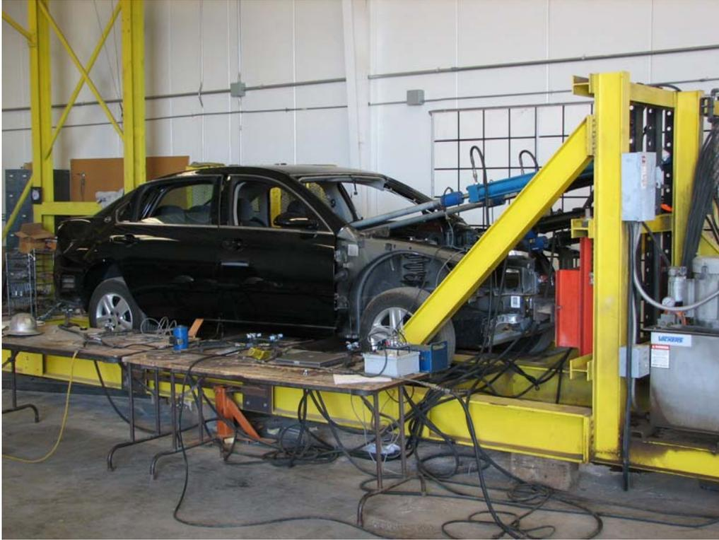
FIGURE 7. Vehicle Mounted in Test Fixture
