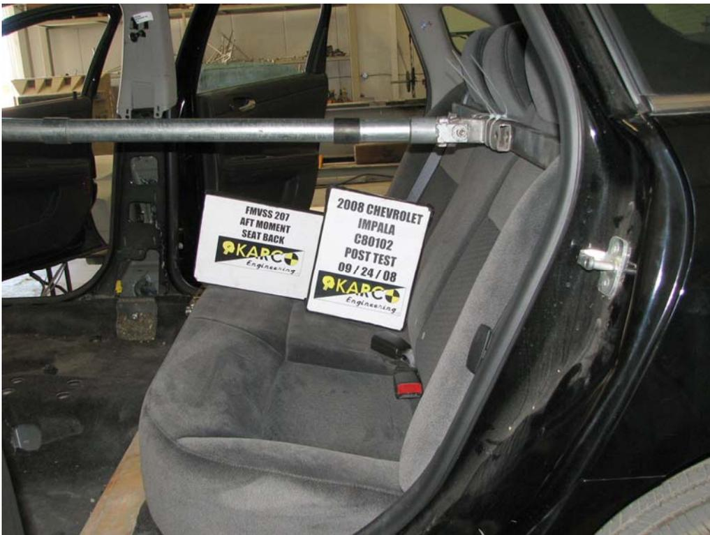
FIGURE 28. Aft Moment on Seat Back, P4, Post-Test
