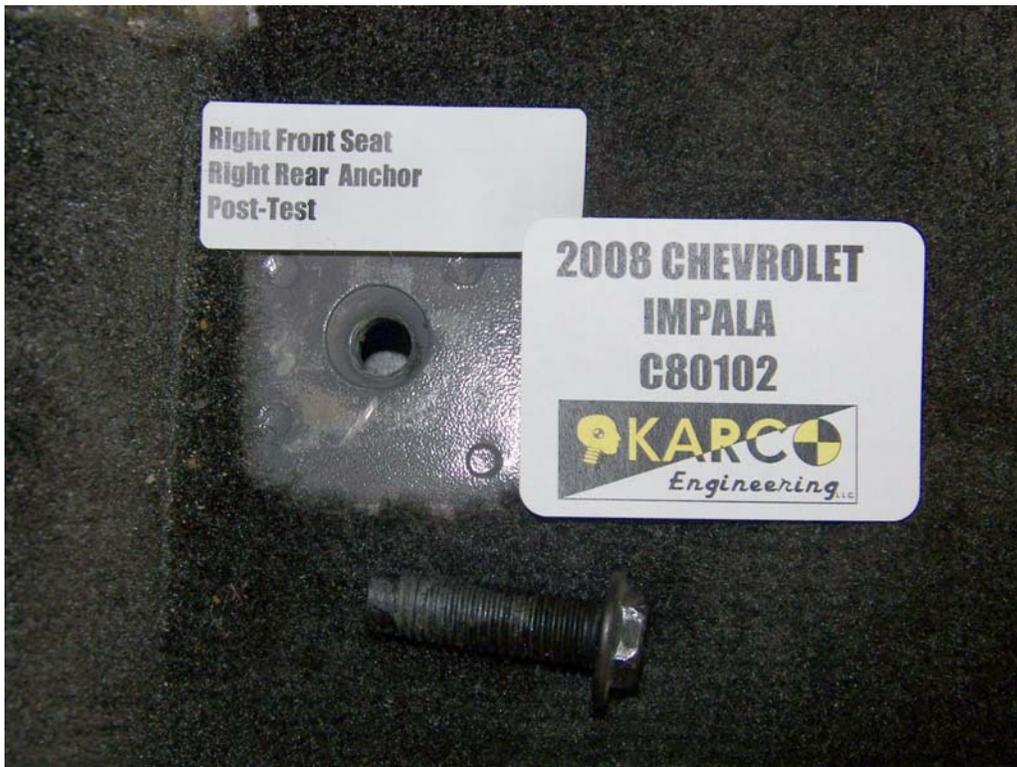
FIGURE 84. Floor Pan Anchor, P2, Post-Test
