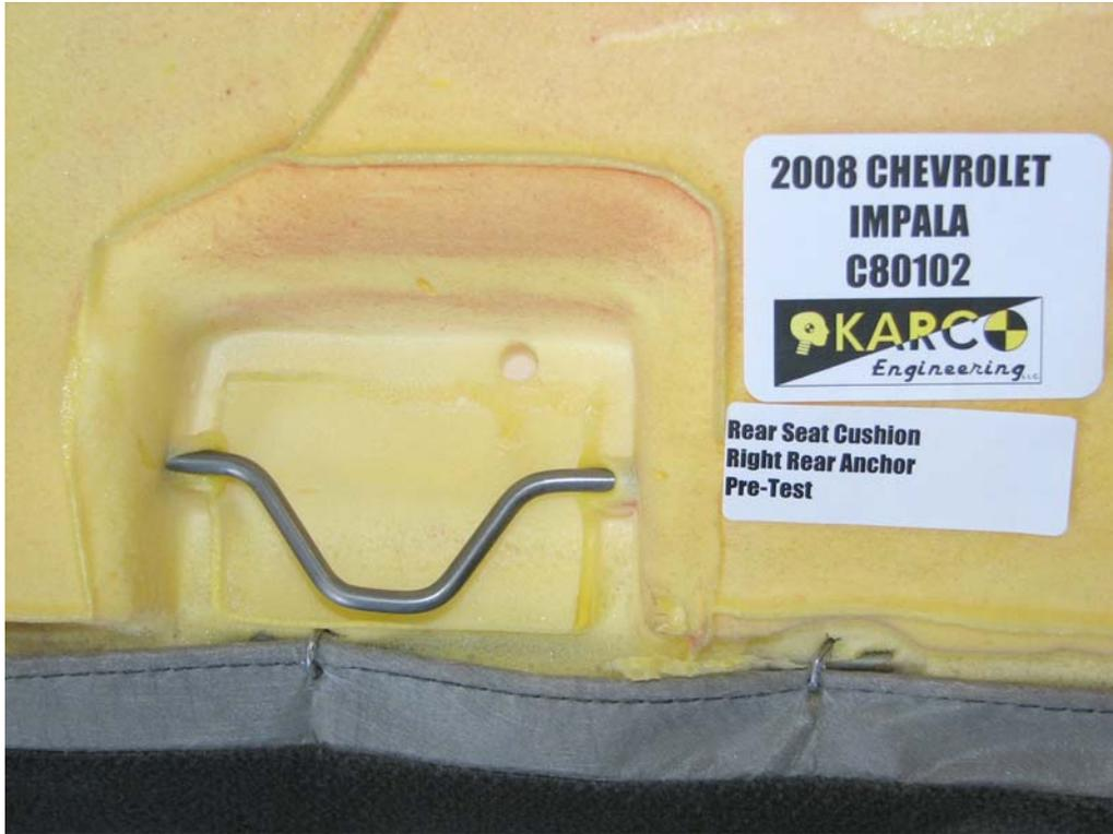
FIGURE 139. Seat Cushion Anchor, P3, Pre-Test
