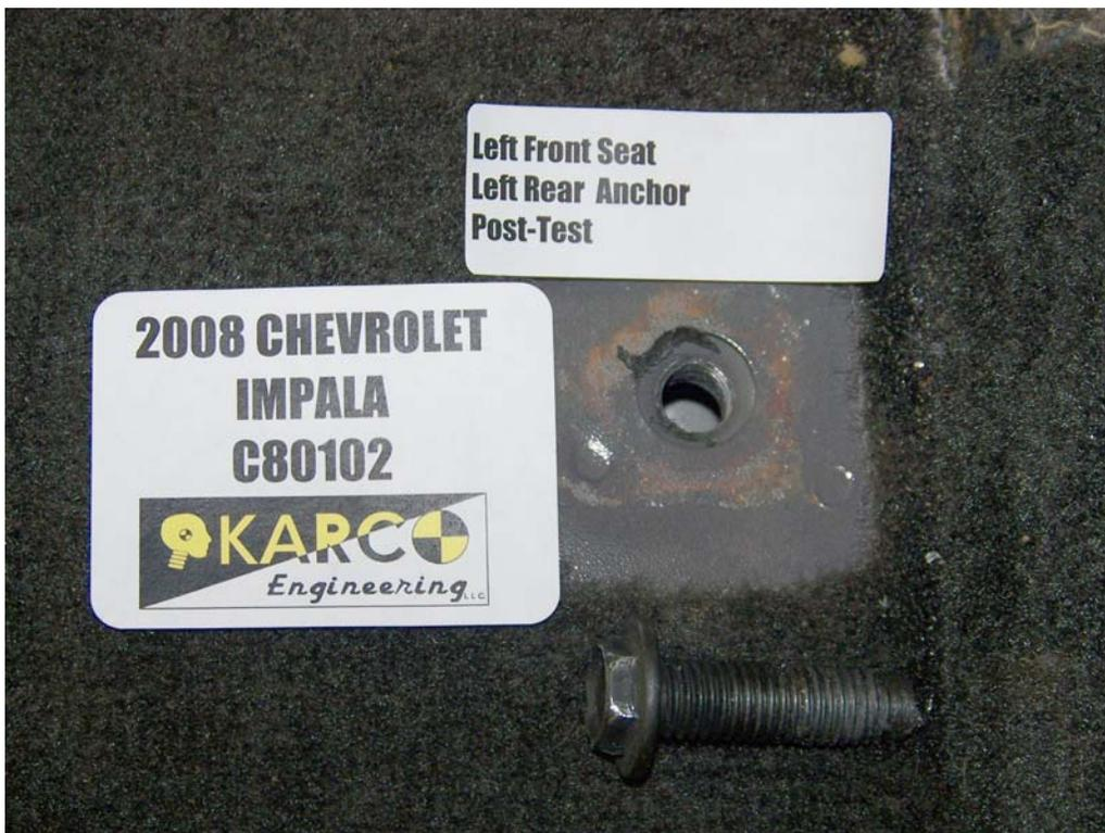
FIGURE 52. Floor Pan Anchor, P1, Post-Test
