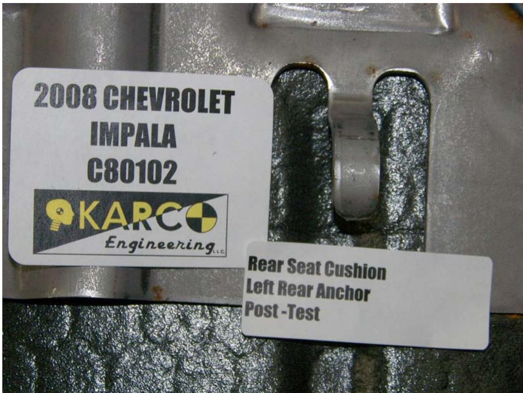
FIGURE 134. Floor Pan Anchor, P4, Post-Test
