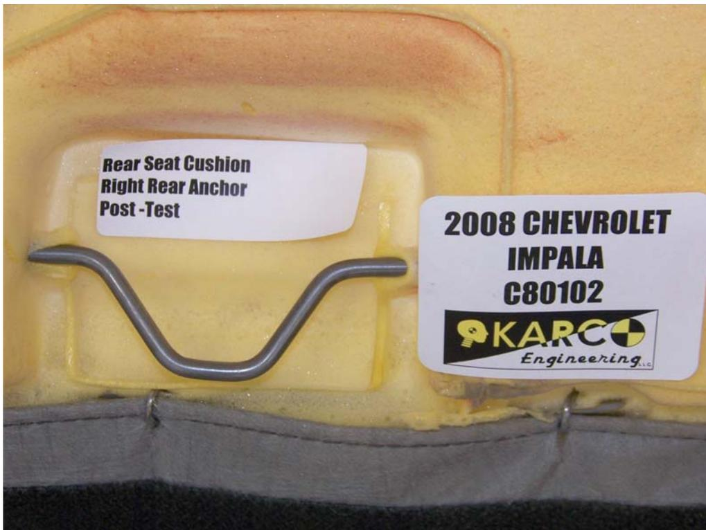
FIGURE 140. Seat Cushion Anchor, P3, Post-Test
