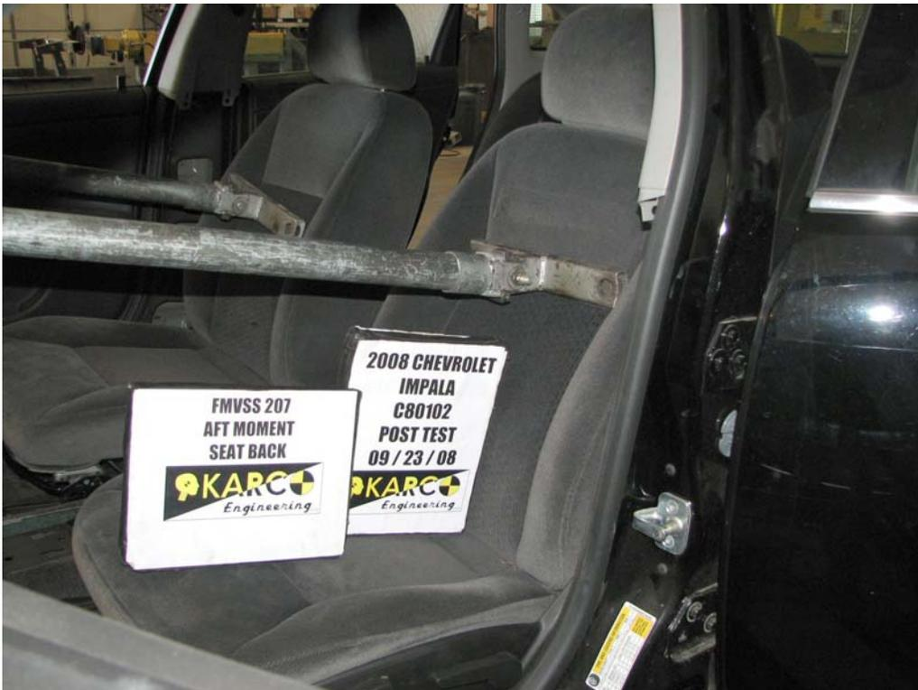
FIGURE 12. Aft Moment on Seat Back, P1, Post-Test
