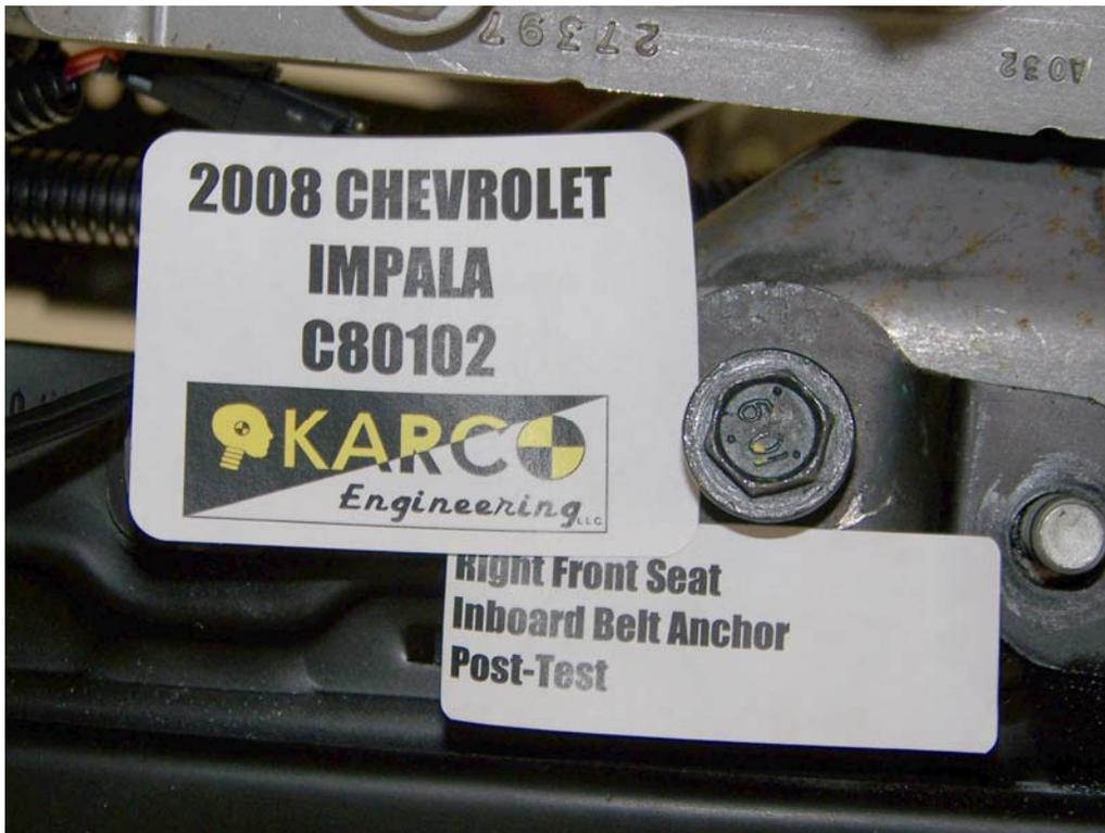
FIGURE 94. Belt Anchor, P2, Post-Test
