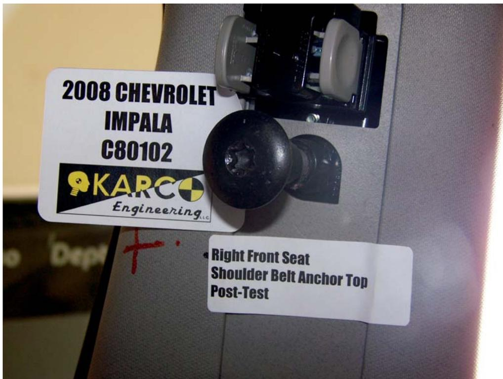
FIGURE 88. Shoulder Belt Anchor, P2, Post-Test
