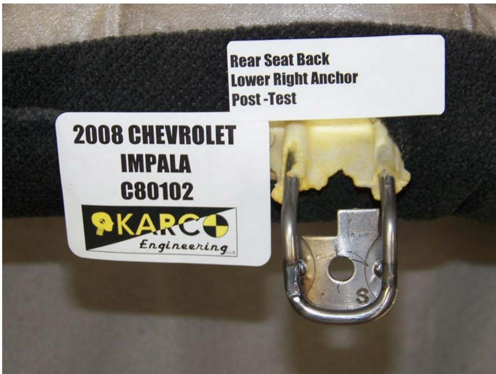
FIGURE 122. Seat Back Anchor, P3, Post-Test
