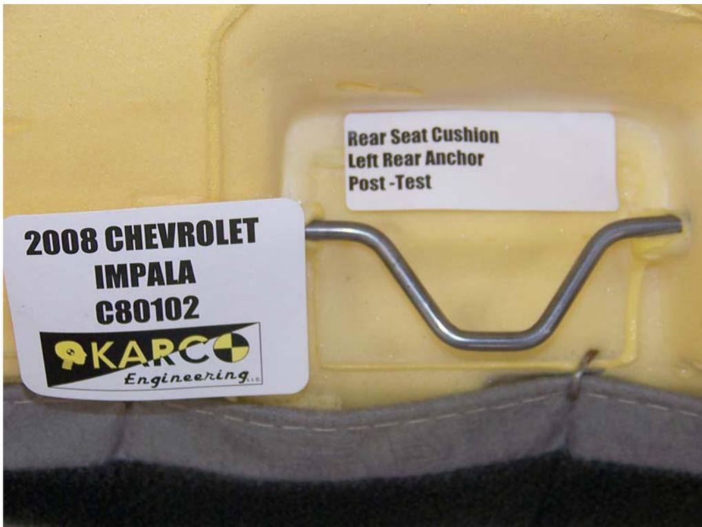
FIGURE 136. Seat Cushion Anchor, P4, Post-Test
