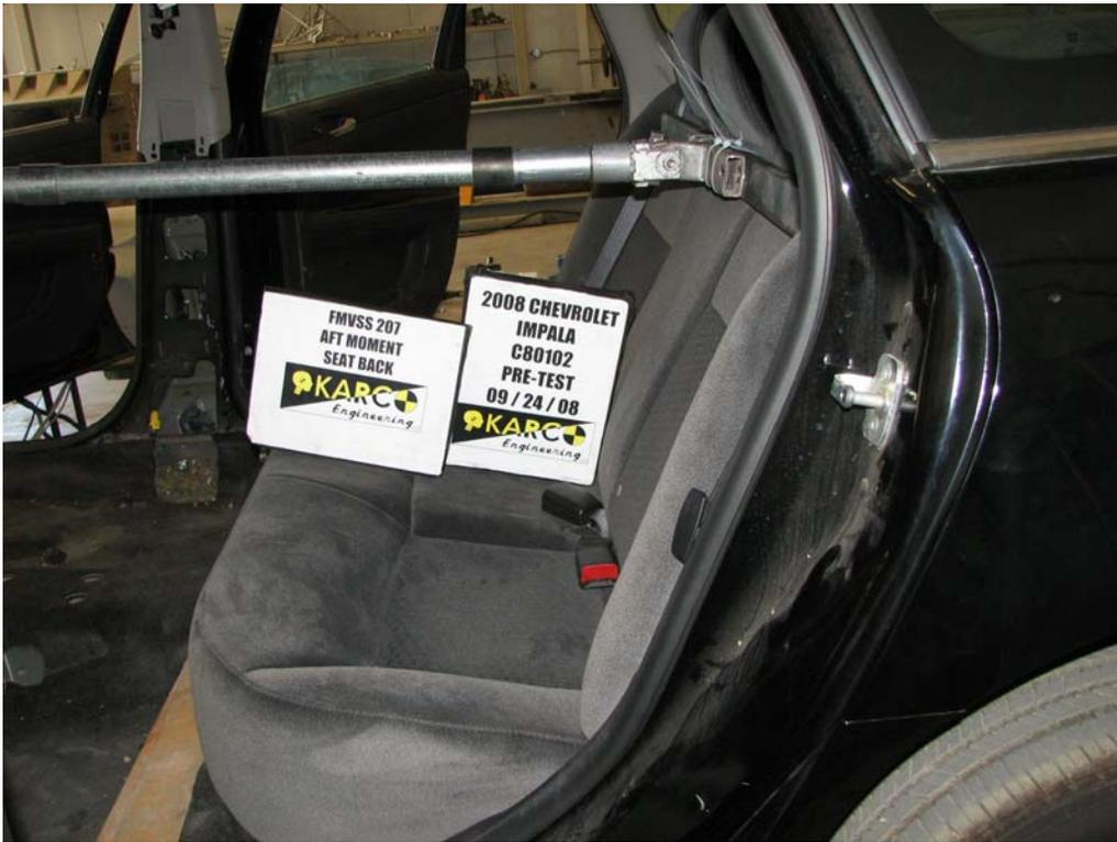
FIGURE 27. Aft Moment on Seat Back, P4, Pre-Test
