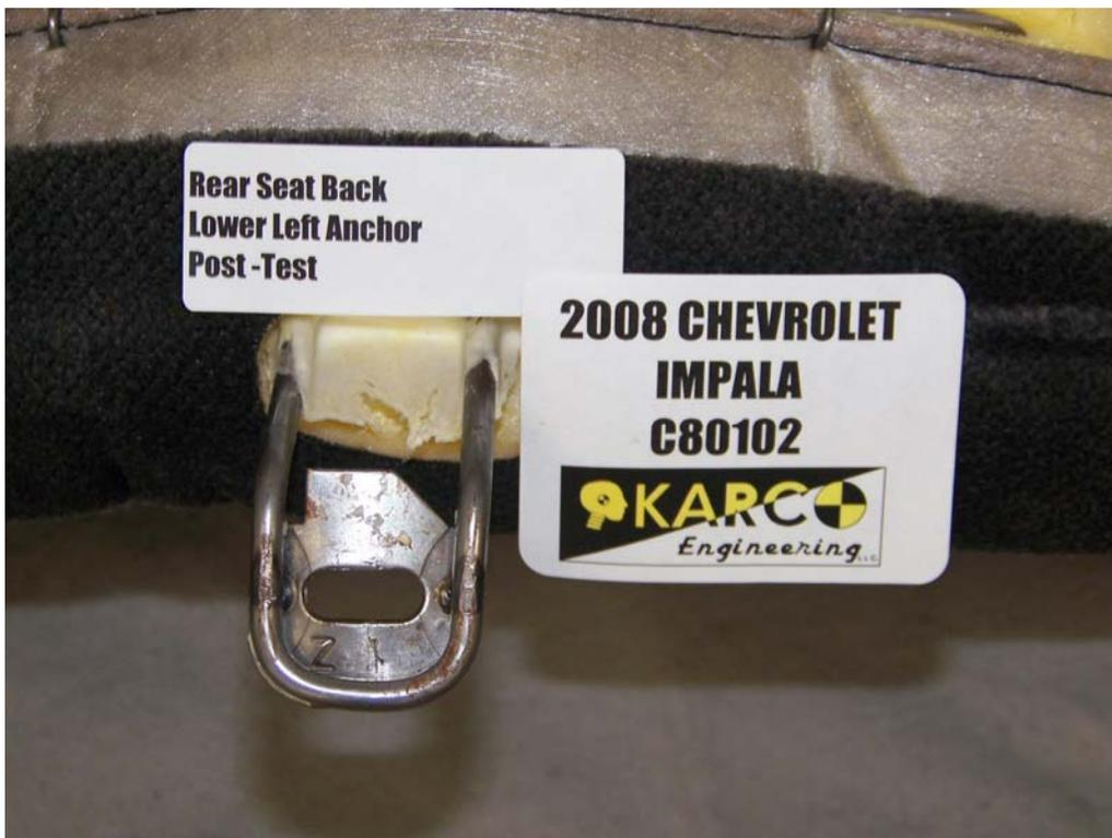
FIGURE 118. Seat Back Anchor, P4, Post-Test
