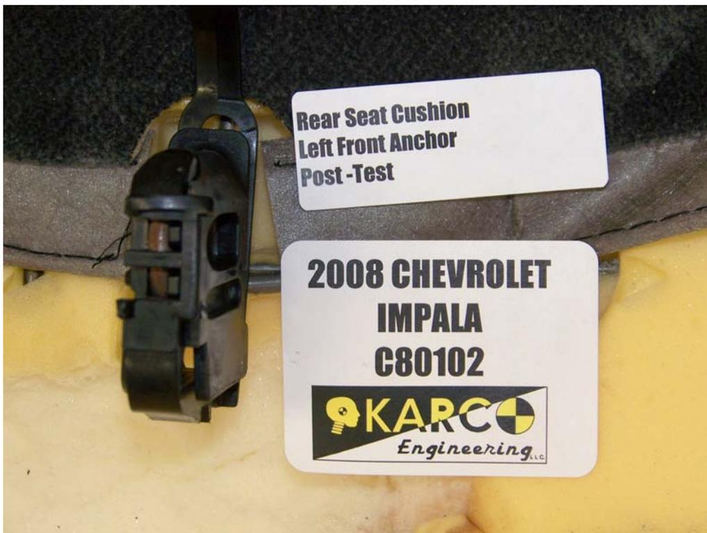
FIGURE 128. Seat Cushion Anchor, P4, Post-Test
