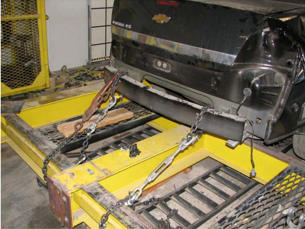
FIGURE 9. Vehicle Mounted in Test Fixture
