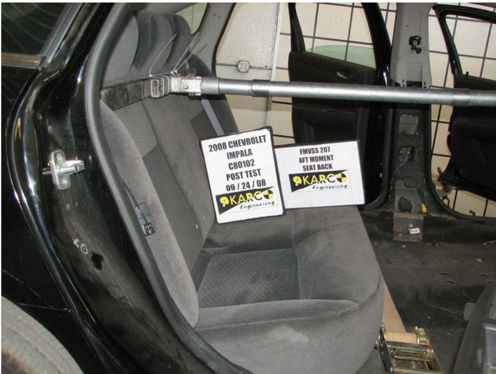
FIGURE 30. Aft Moment on Seat Back, P3, Post-Test
