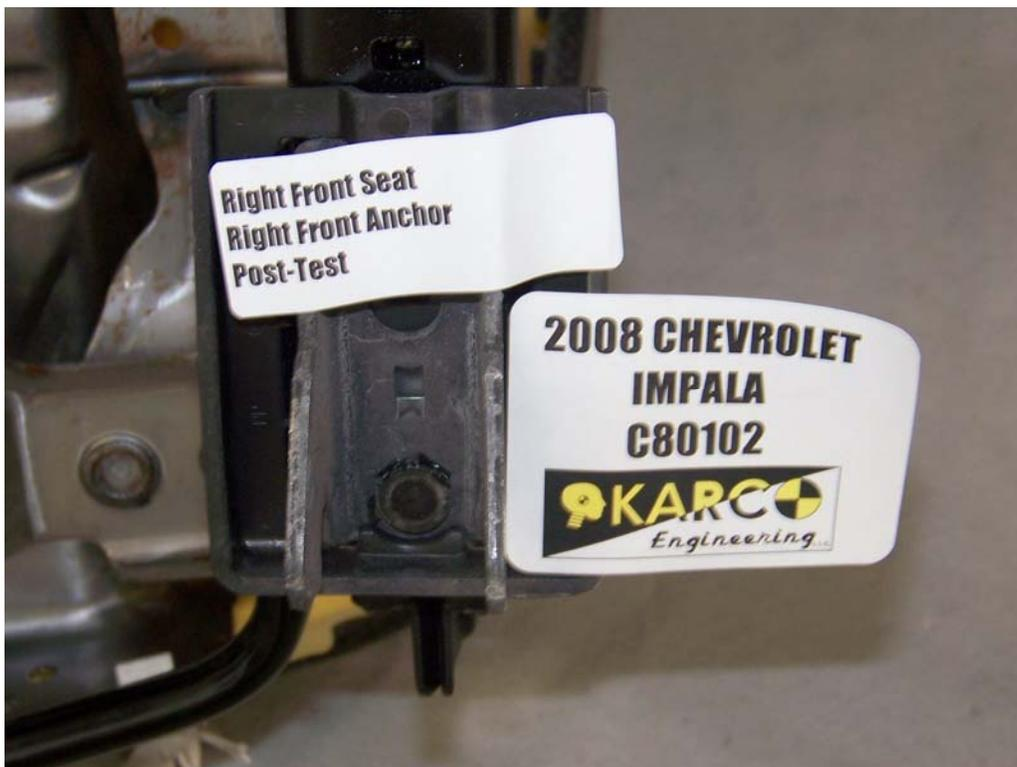
FIGURE 78. Seat Anchor, P2, Post-Test
