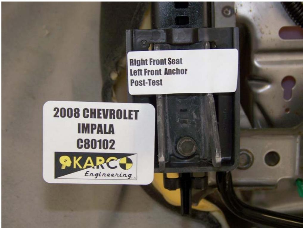
FIGURE 74. Seat Anchor, P2, Post-Test
