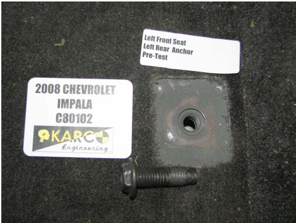
FIGURE 51. Floor Pan Anchor, P1, Pre-Test
