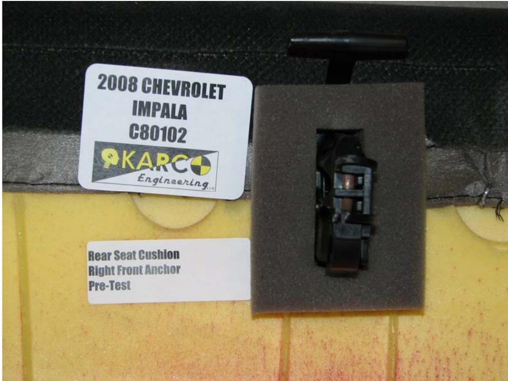
FIGURE 131. Seat Cushion Anchor, P3, Pre-Test
