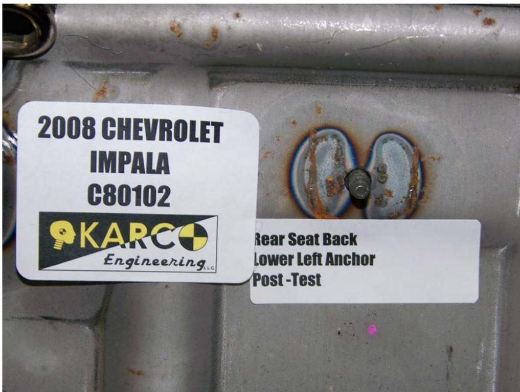
FIGURE 116. Floor Pan Anchor, P4, Post-Test
