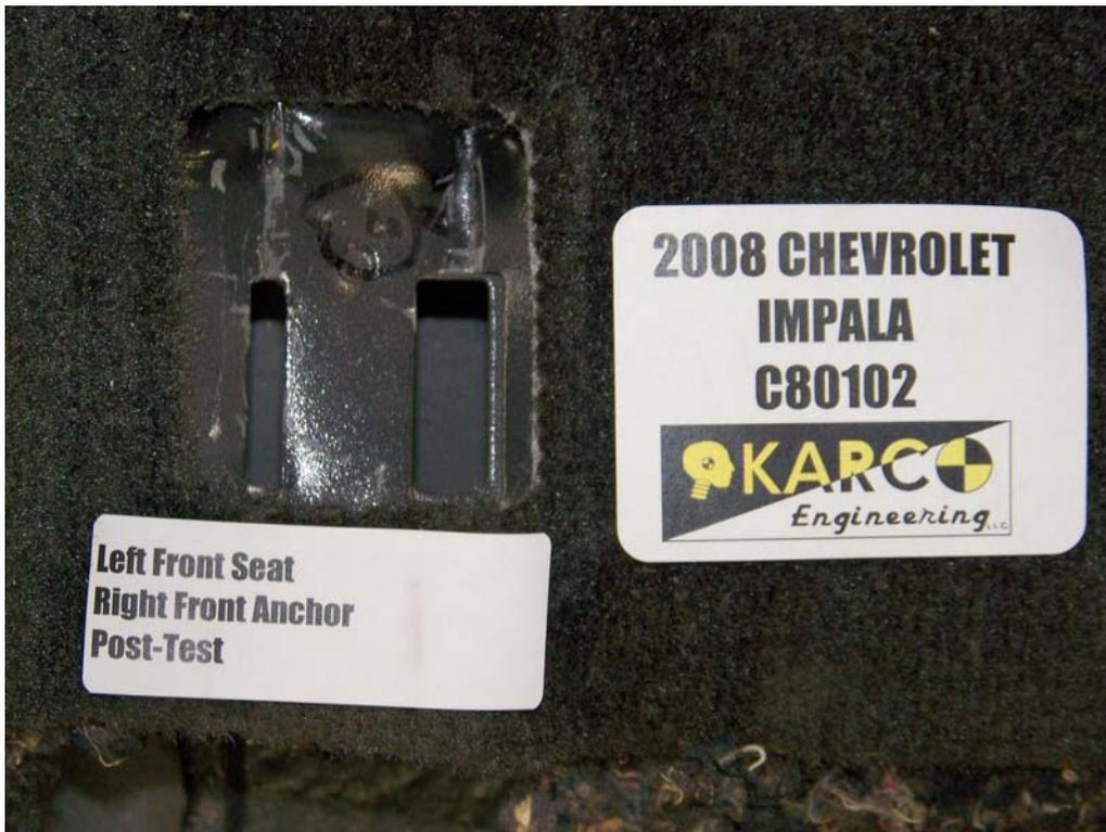
FIGURE 48. Floor Pan Anchor, P1, Post-Test
