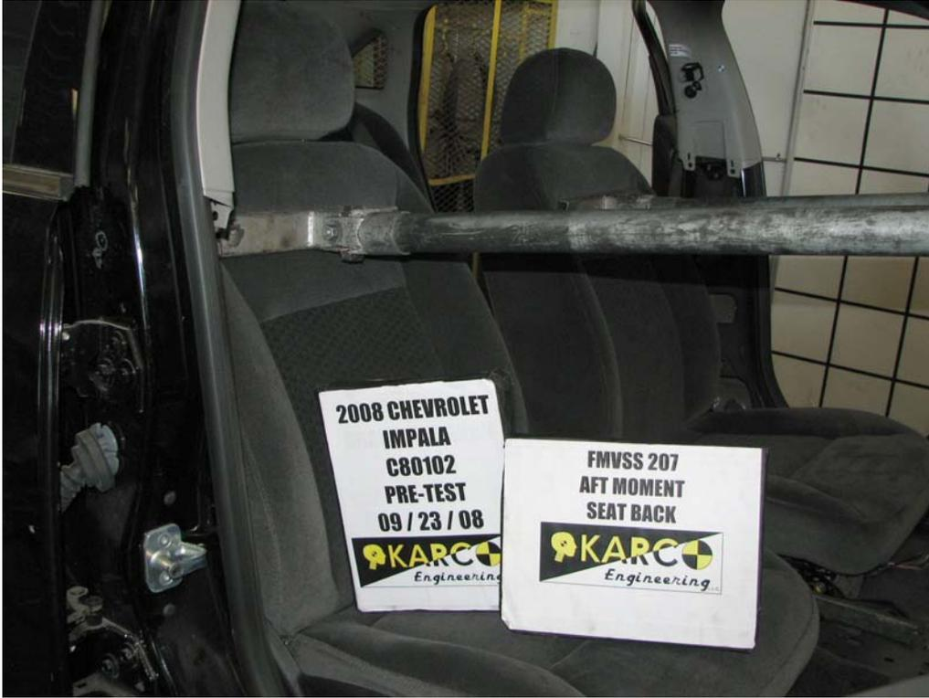
FIGURE 13. Aft Moment on Seat Back, P2, Pre-Test
