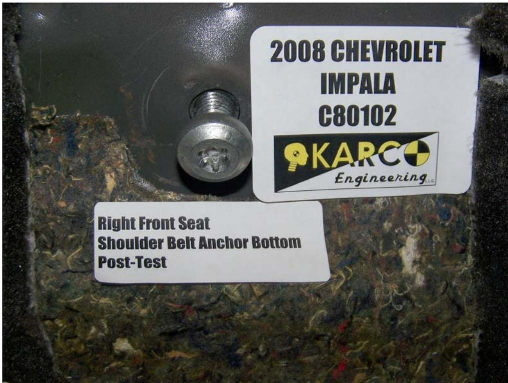
FIGURE 90. Shoulder Belt Anchor, P2, Post-Test
