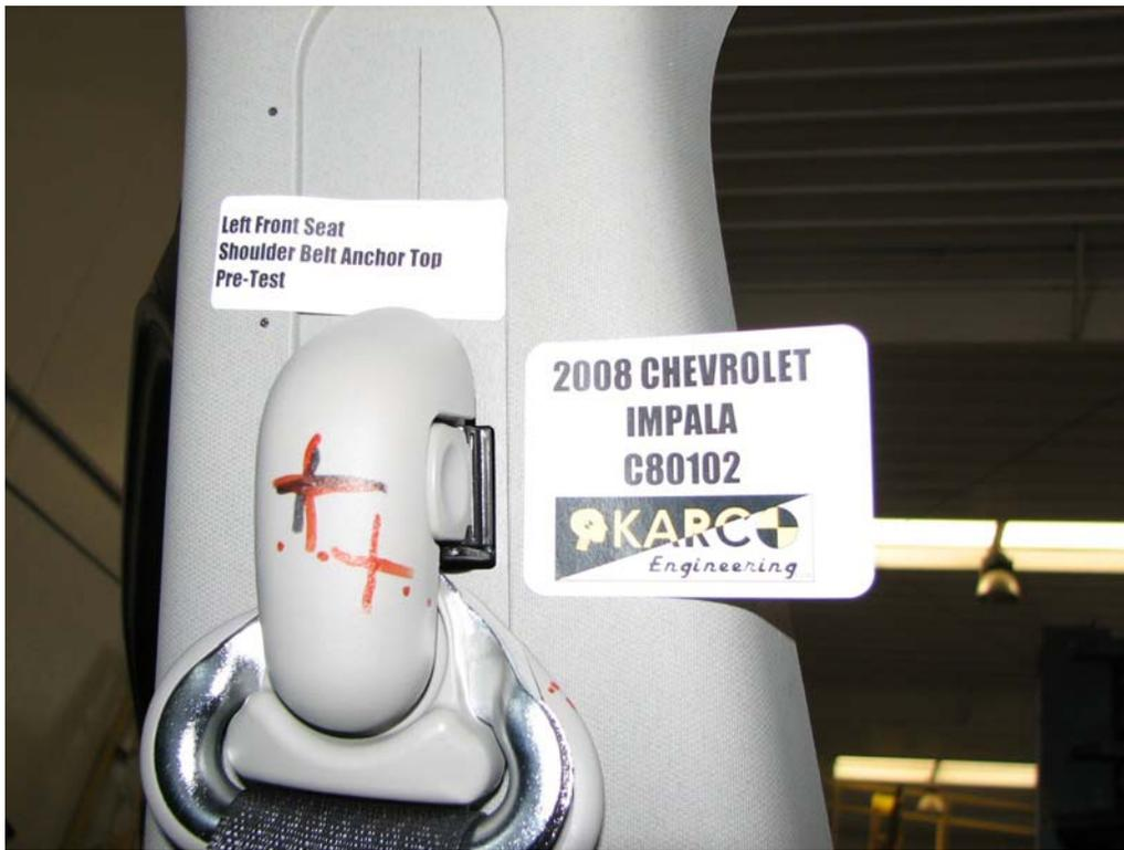
FIGURE 59. Shoulder Belt Anchor, P1, Pre-Test
