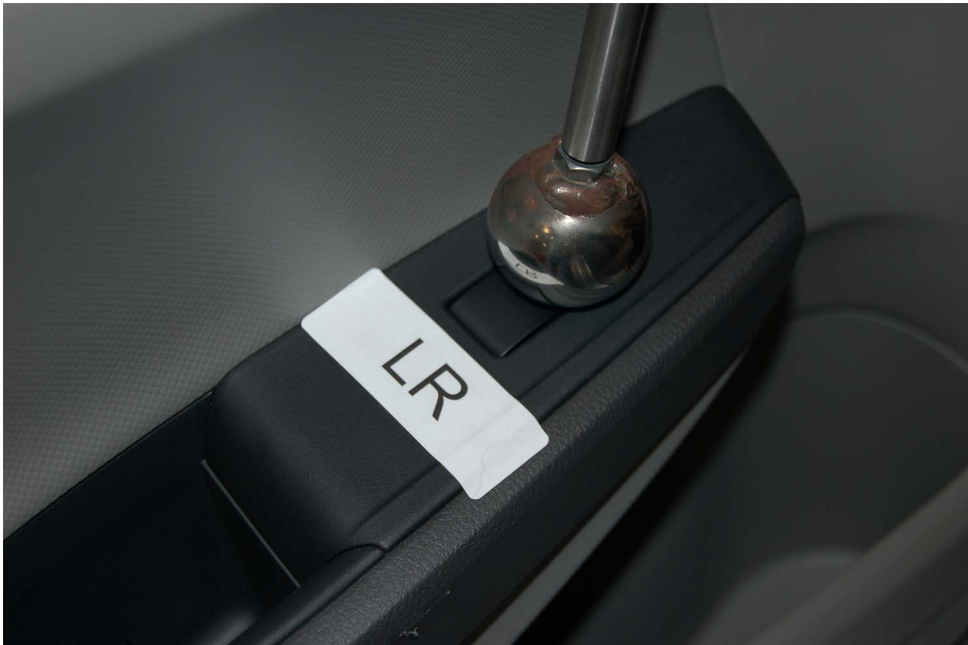
FIGURE 5.11 TYPICAL SWITCH/SPHERE TEST SET-UP
