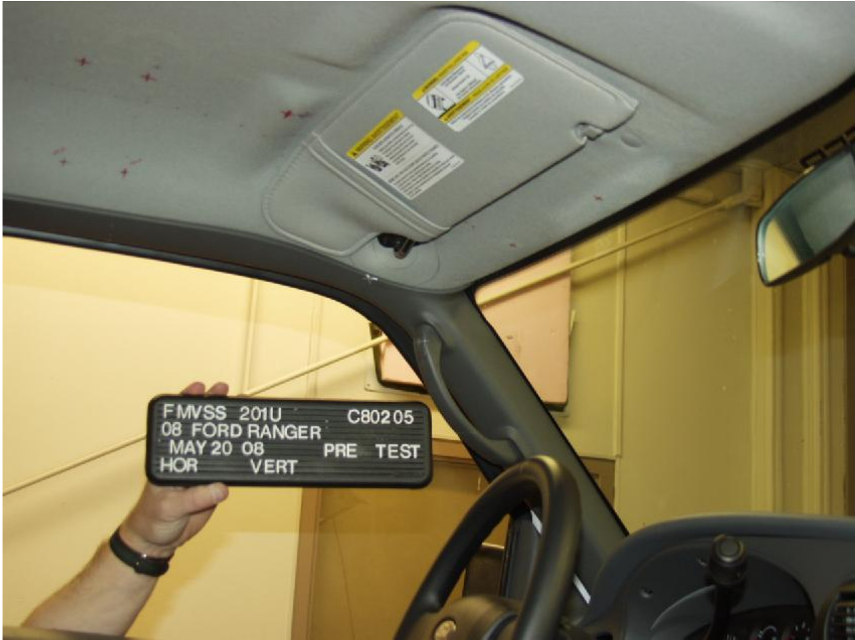
Figure A-7 : PRE-TEST DRIVER SIDE A-PILLAR
