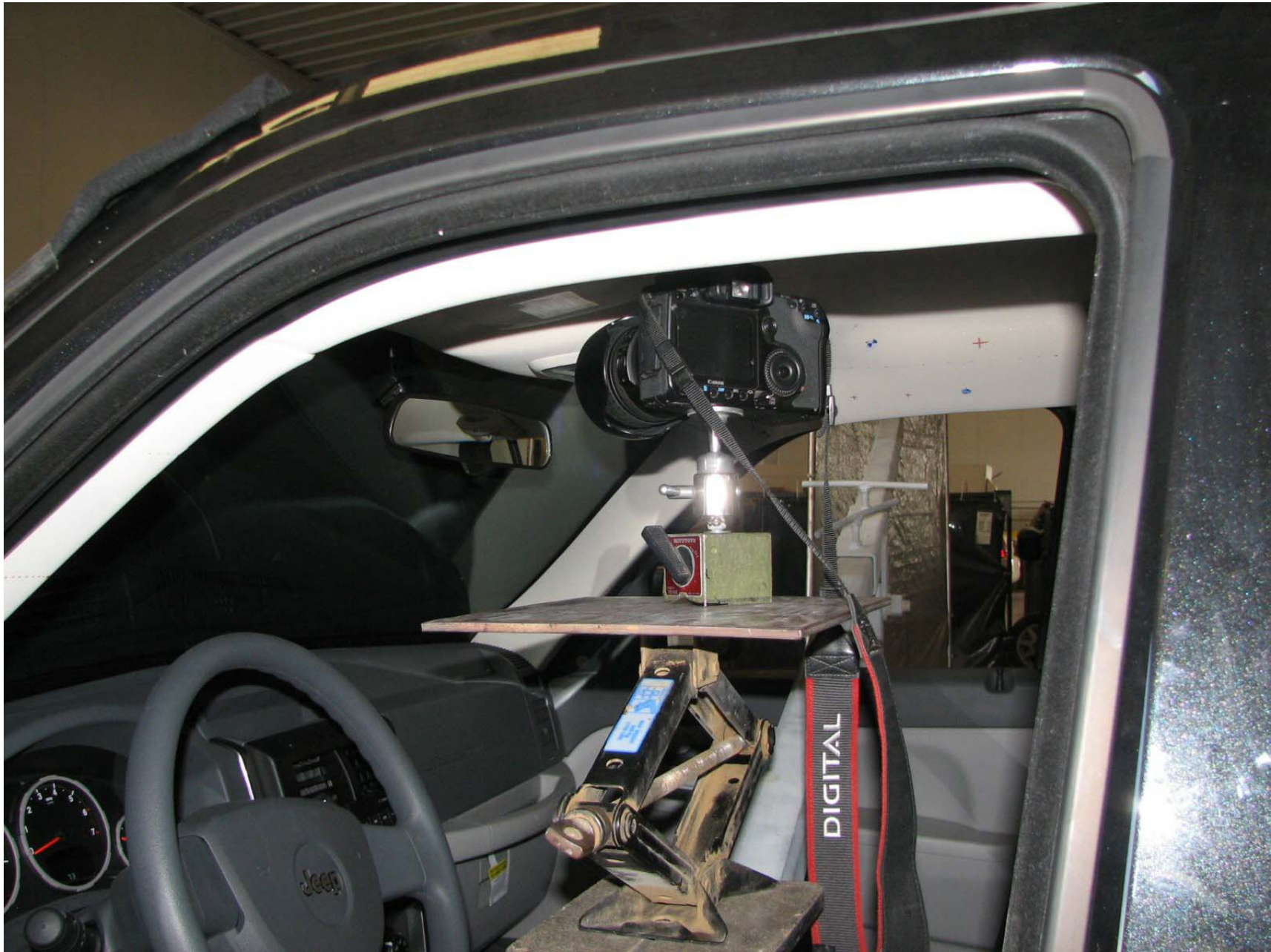
FIGURE 11:CAMERA SET-UP FOR PHOTOGRAPHING REFERENCE BOARD
