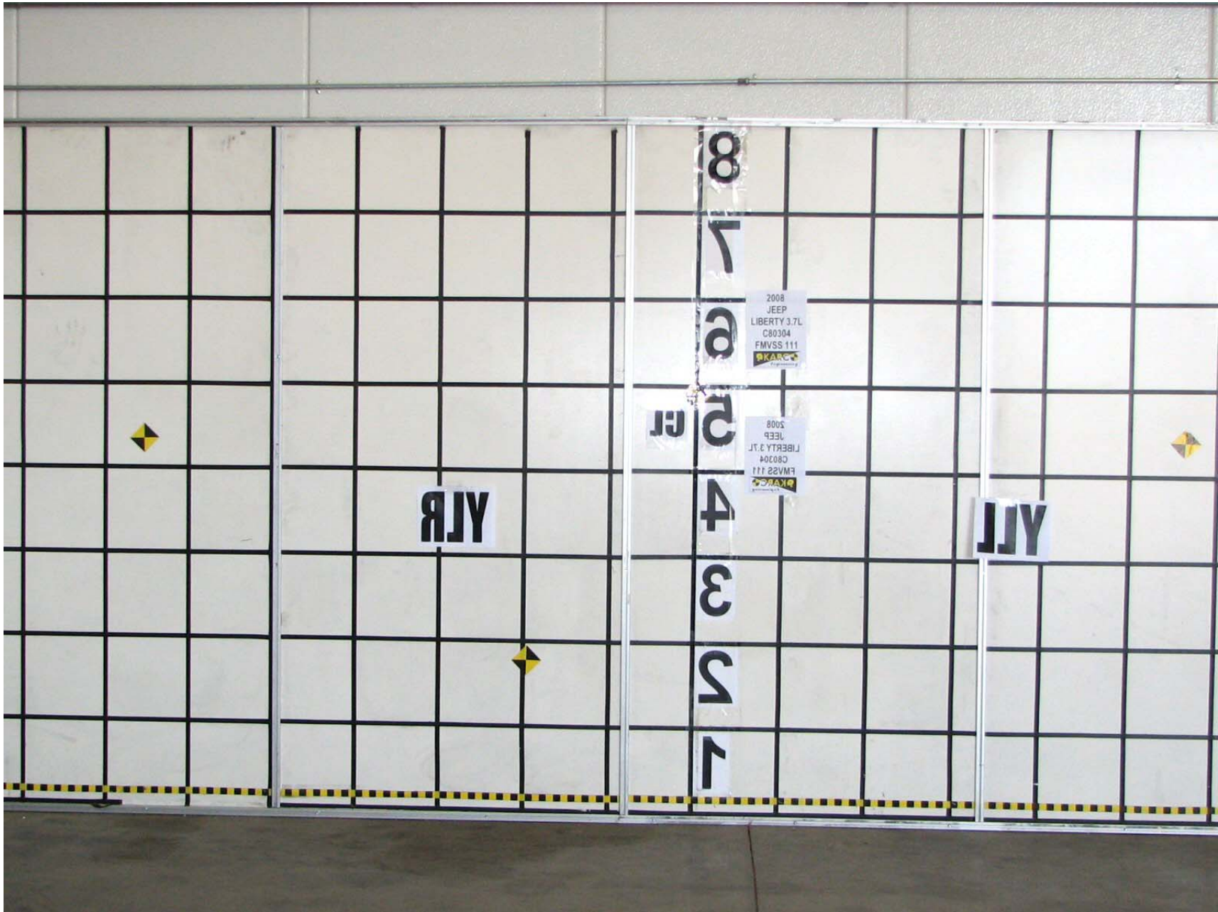
FIGURE 17:REFERENCE BOARD FOR INSIDE MIRROR, LEFT EYE
