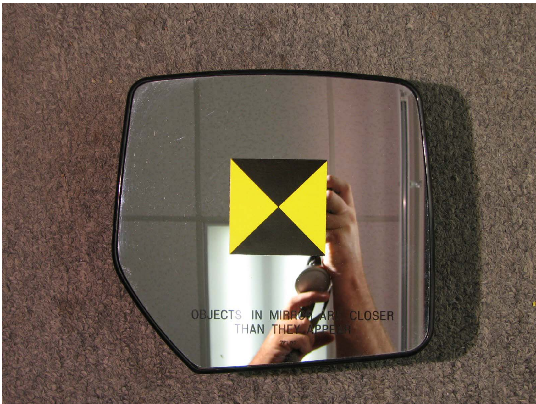
FIGURE 15: MIRROR SET-UP FOR AREA MEASUREMENT
