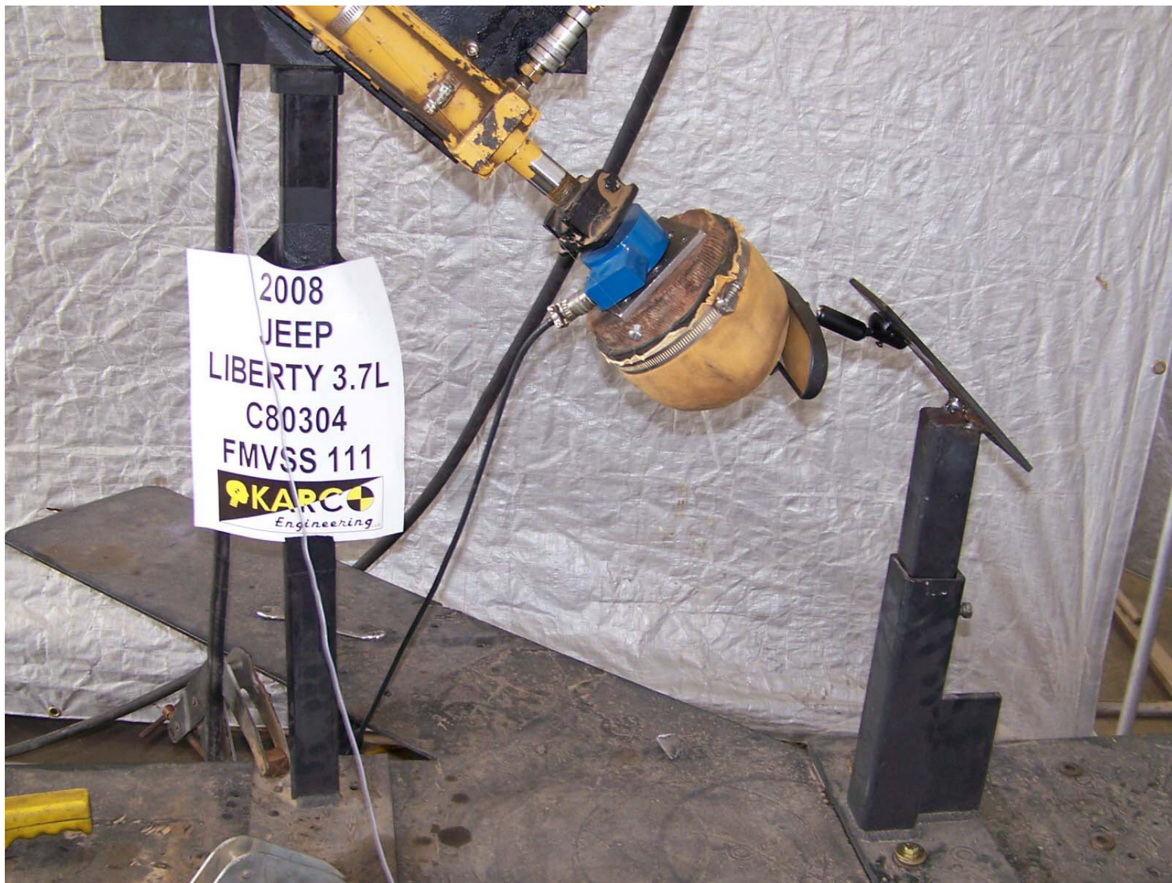
FIGURE 13:CLOSE-UP OF MIRROR BREAK- AWAY TEST
