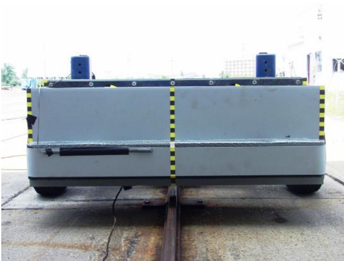
Figure A-19: Pre-Test MDB Front View
