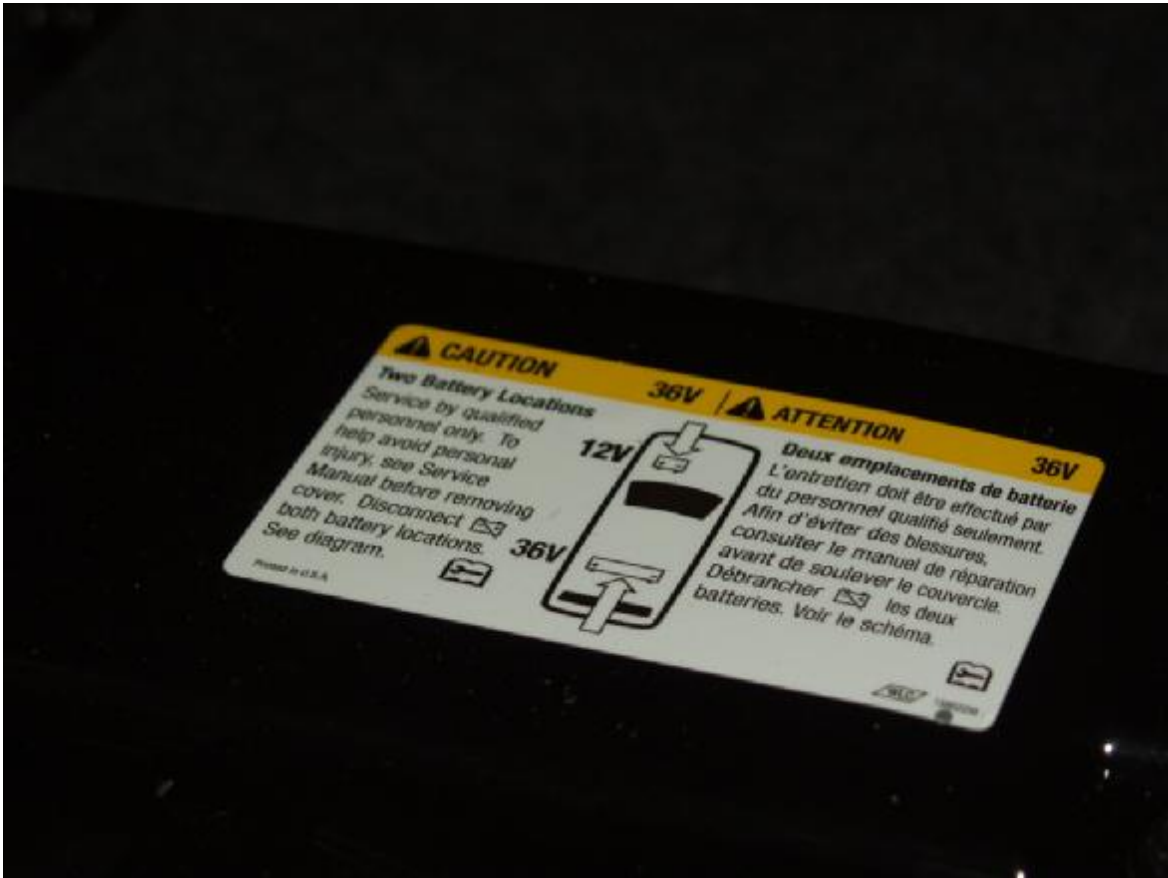
Figure A-3: Vehicle Electric Propulsion System Label
