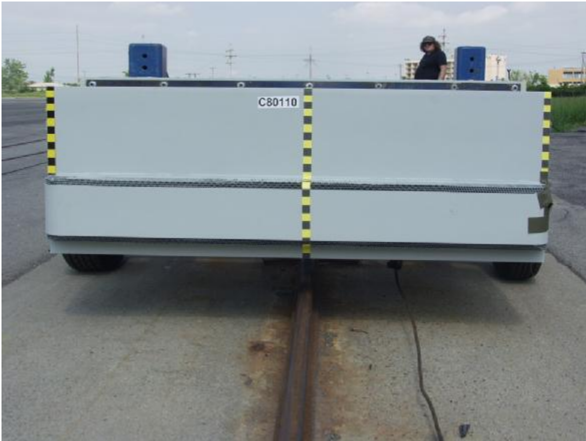
Figure A-23: Pre-Test MDB Front View
