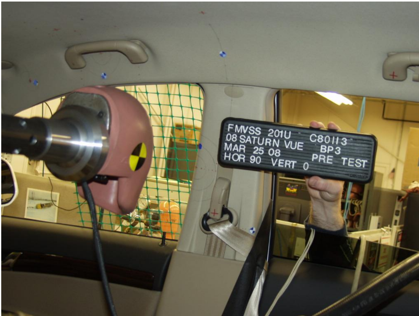
PRE-IMPACT BP3 (TEST PLACARD DATE SHOULD BE MAR. 26, 2008)
