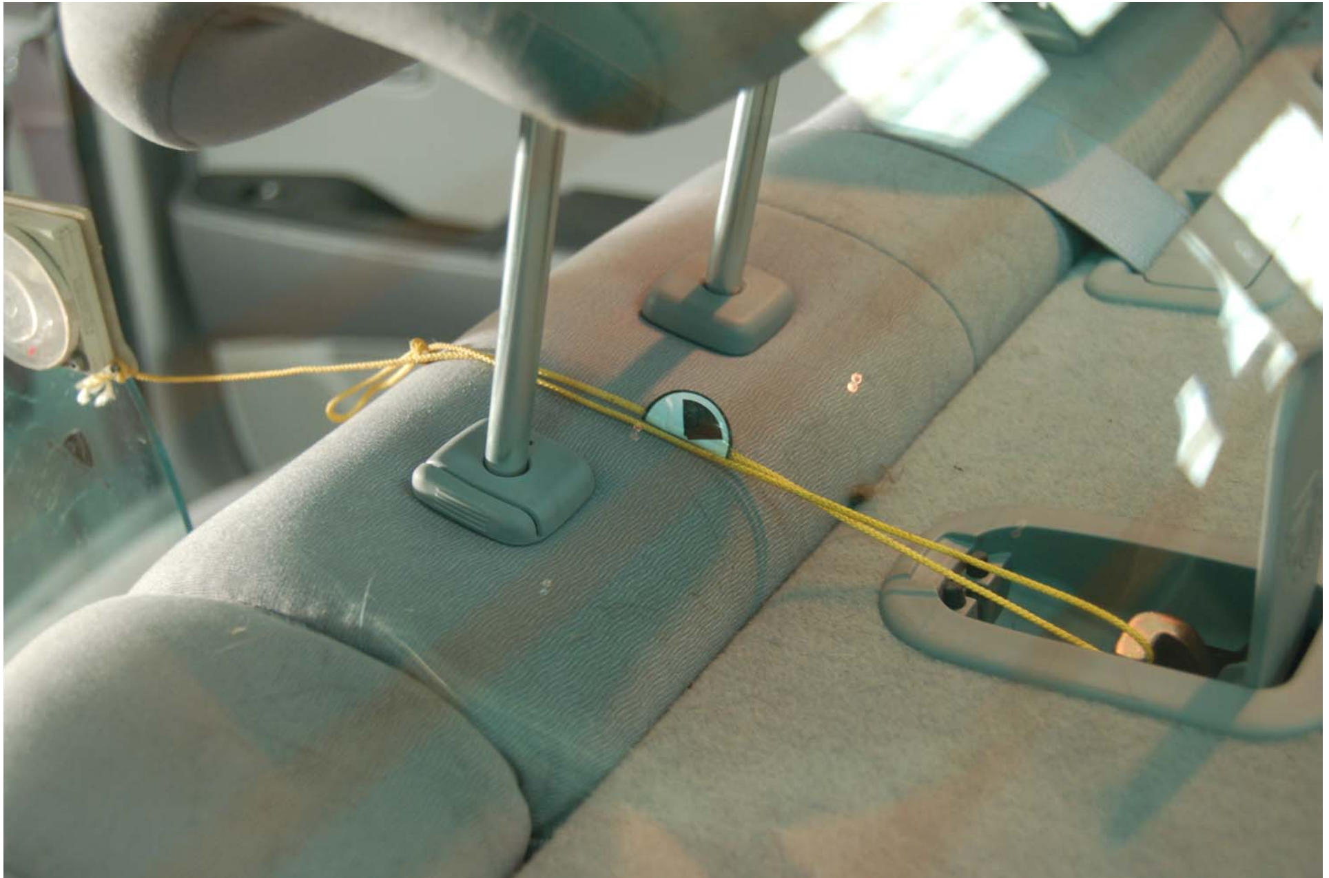
FIGURE 5.24 ROW 2, TOP TETHER ROUTING
