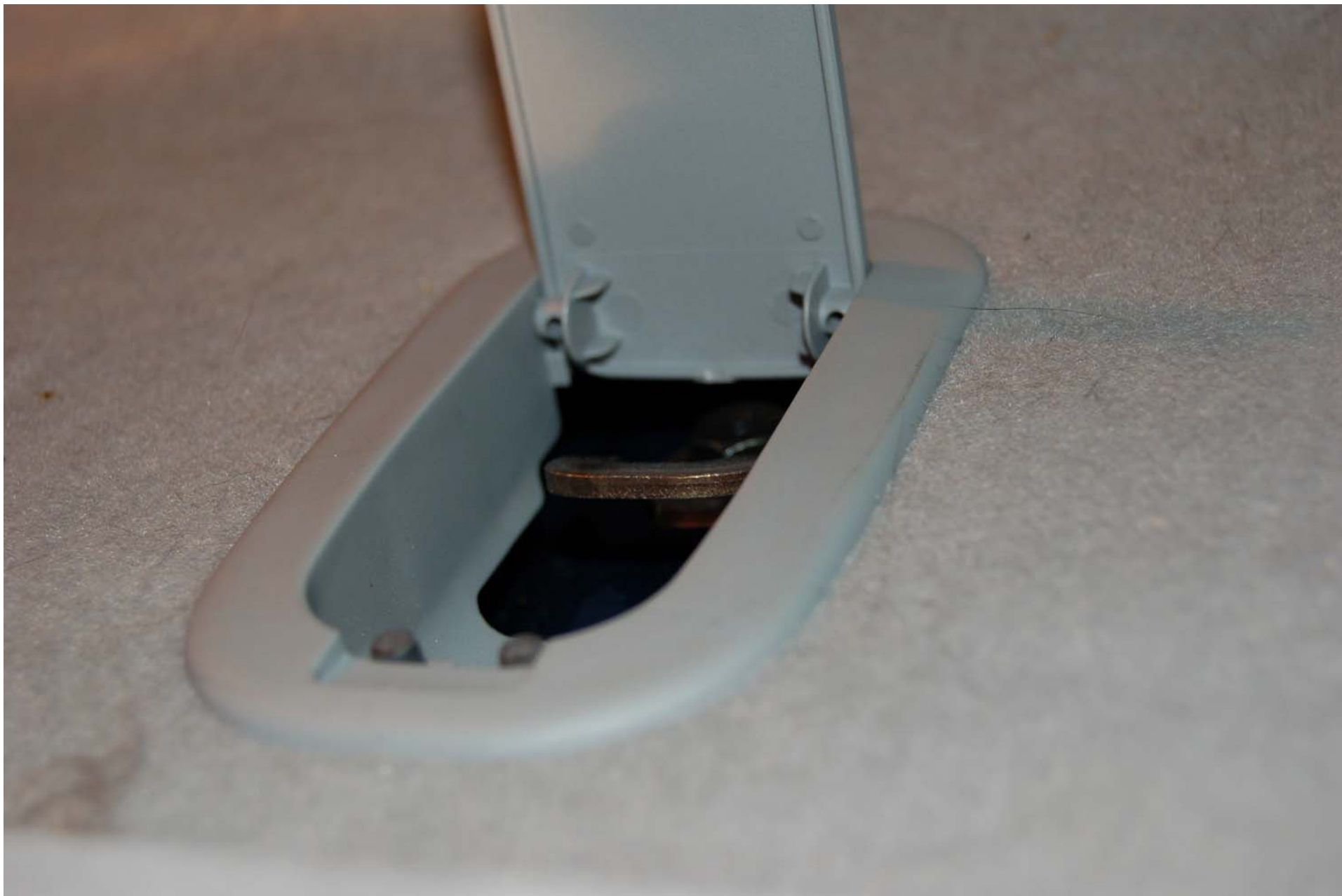
FIGURE 5.9 ROW 2, CENTER, TOP TETHER ANCHOR, PRE-TEST
