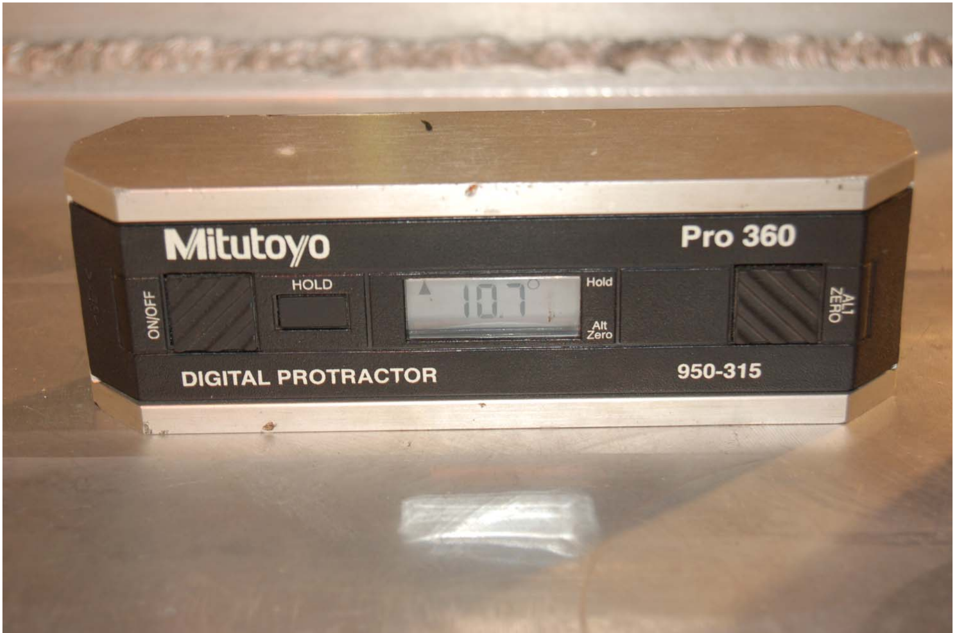
FIGURE 5.31 ROW 2, RIGHT SIDE CRF PITCH MEASUREMENT
