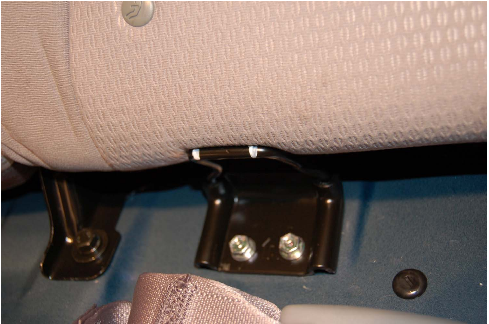
FIGURE 5.7 ROW 2, LEFT SIDE, INBOARD LOWER ANCHOR, PRE-TEST
