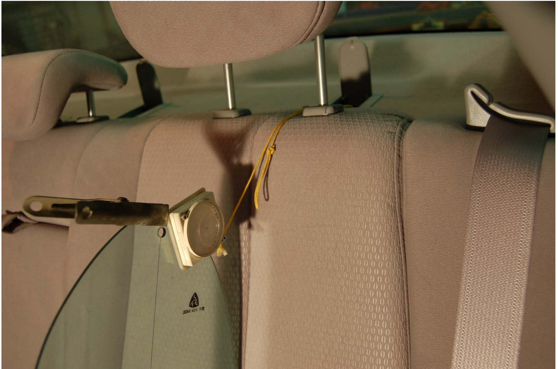
FIGURE 5.16 ROW 2, LEFT SIDE TOP TETHER ROUTING
