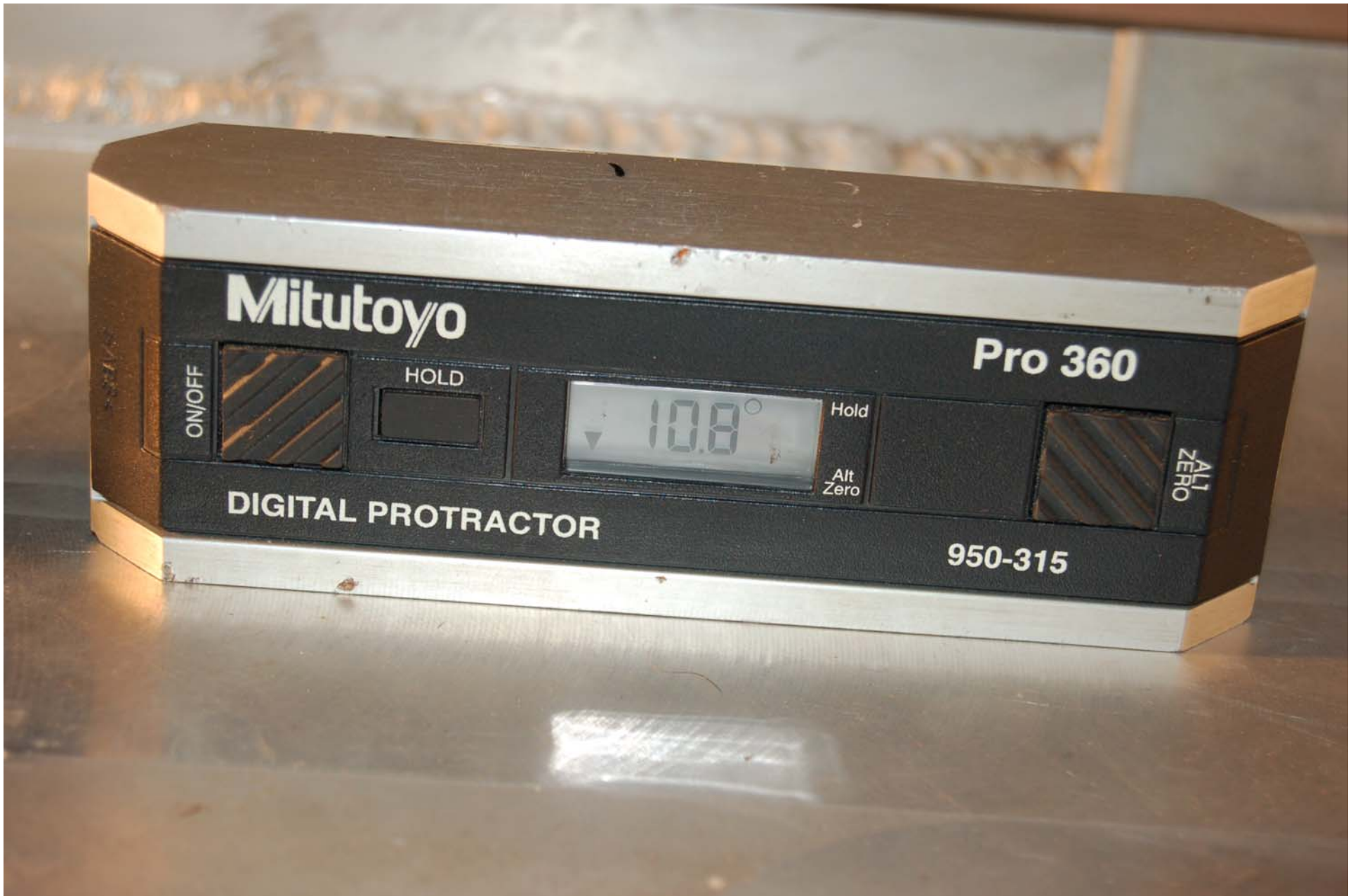
FIGURE 5.30 ROW 2, LEFT SIDE CRF PITCH MEASUREMENT
