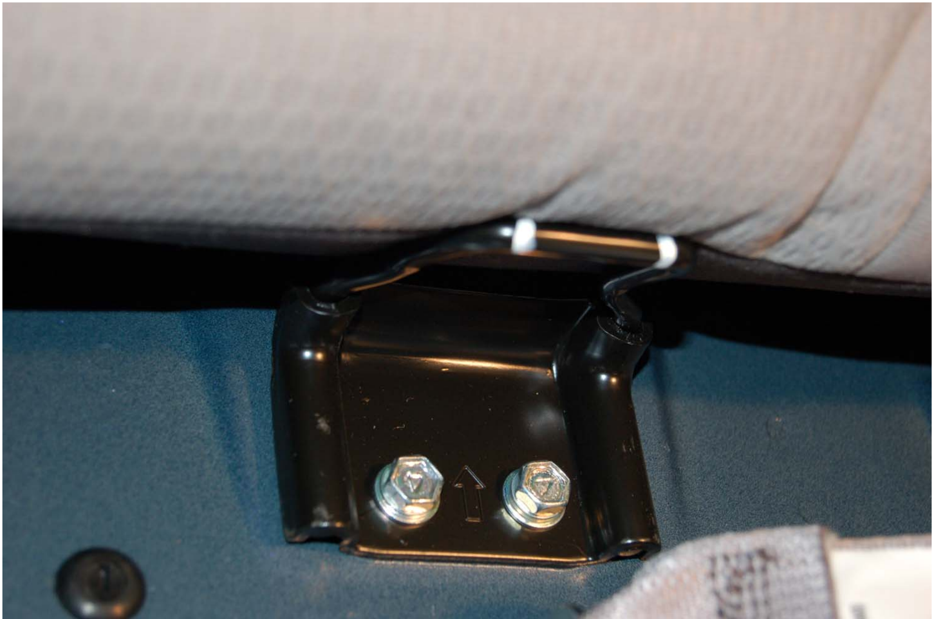
FIGURE 5.10 ROW 2, RIGHT SIDE, INBOARD LOWER ANCHOR , PRE-TEST
