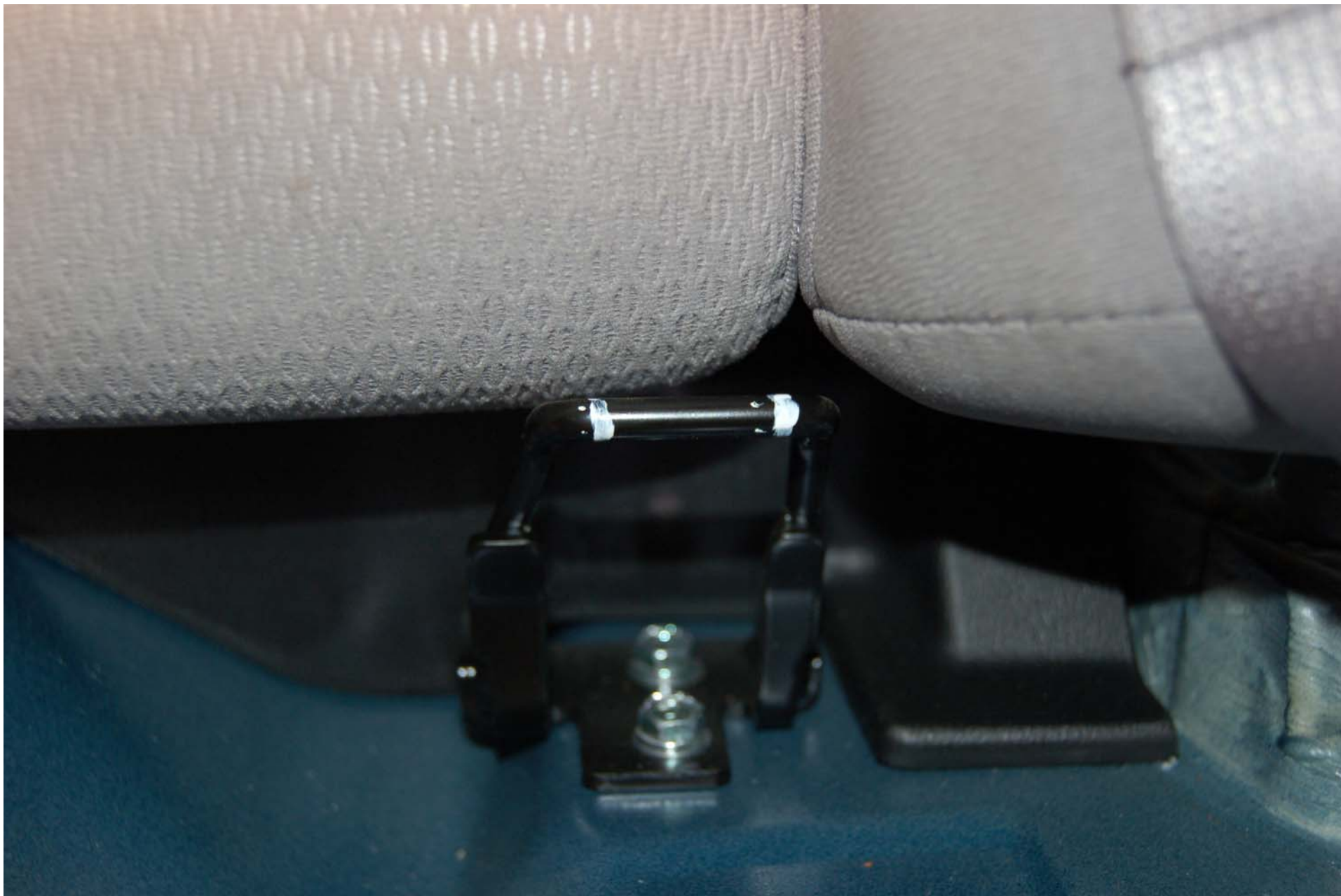
FIGURE 5.6 ROW 2, LEFT SIDE, OUTBOARD LOWER ANCHOR, PRE-TEST
