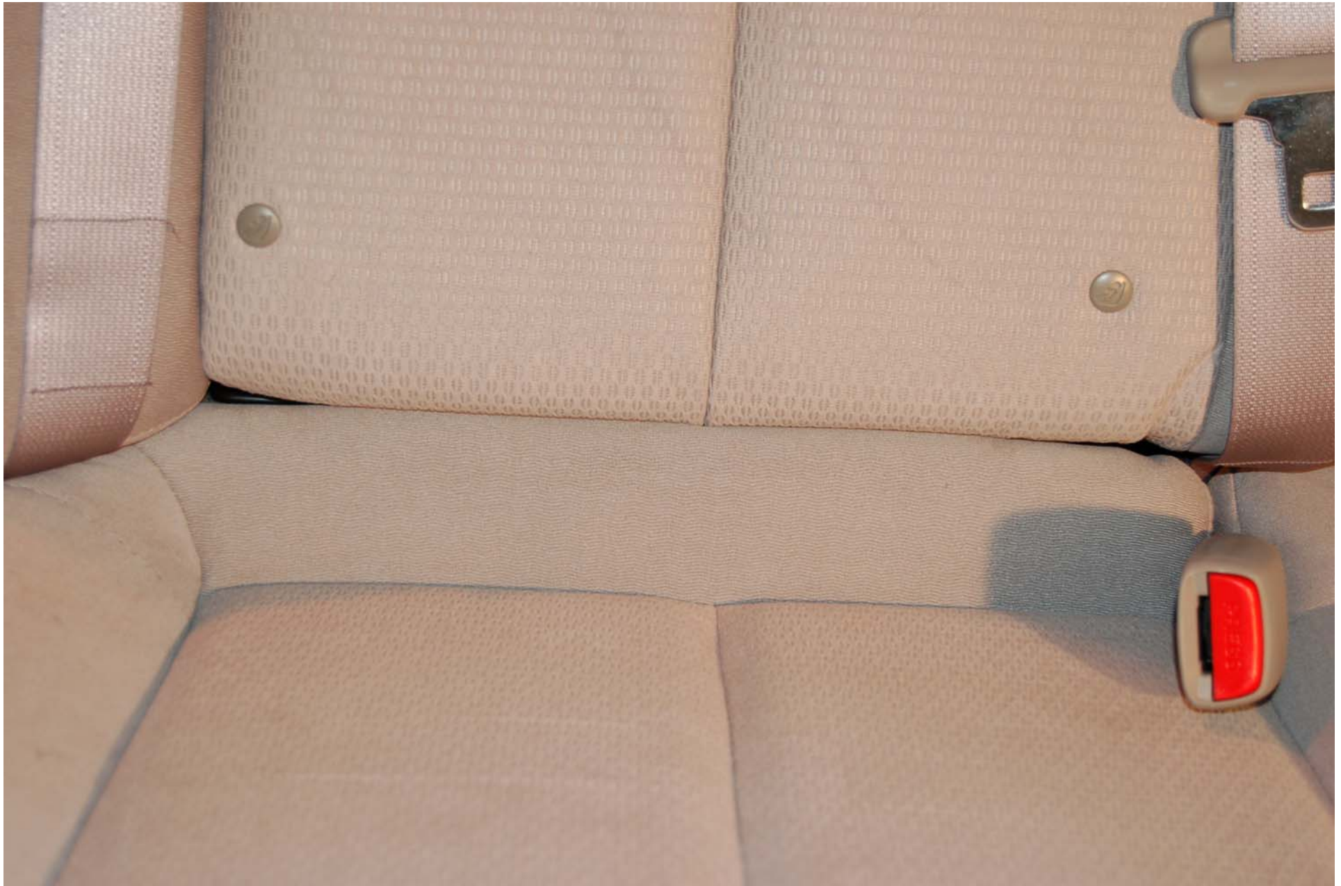
FIGURE 5.5 VISIBILITY OF LOWER ANCHORS
