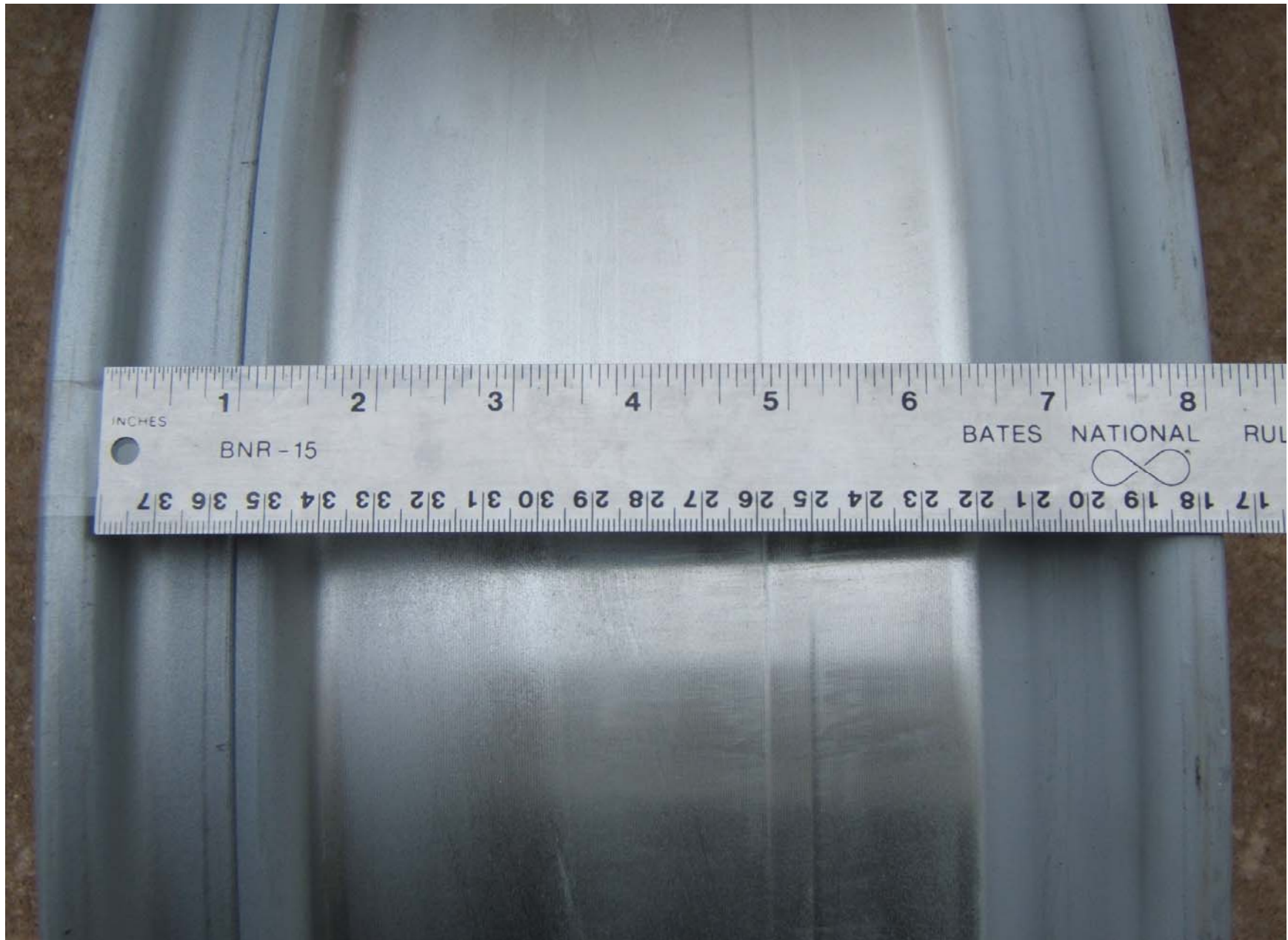
FIGURE 5.11 RIM CONTOUR FOR FULL WIDTH OF CROSS SECTION
