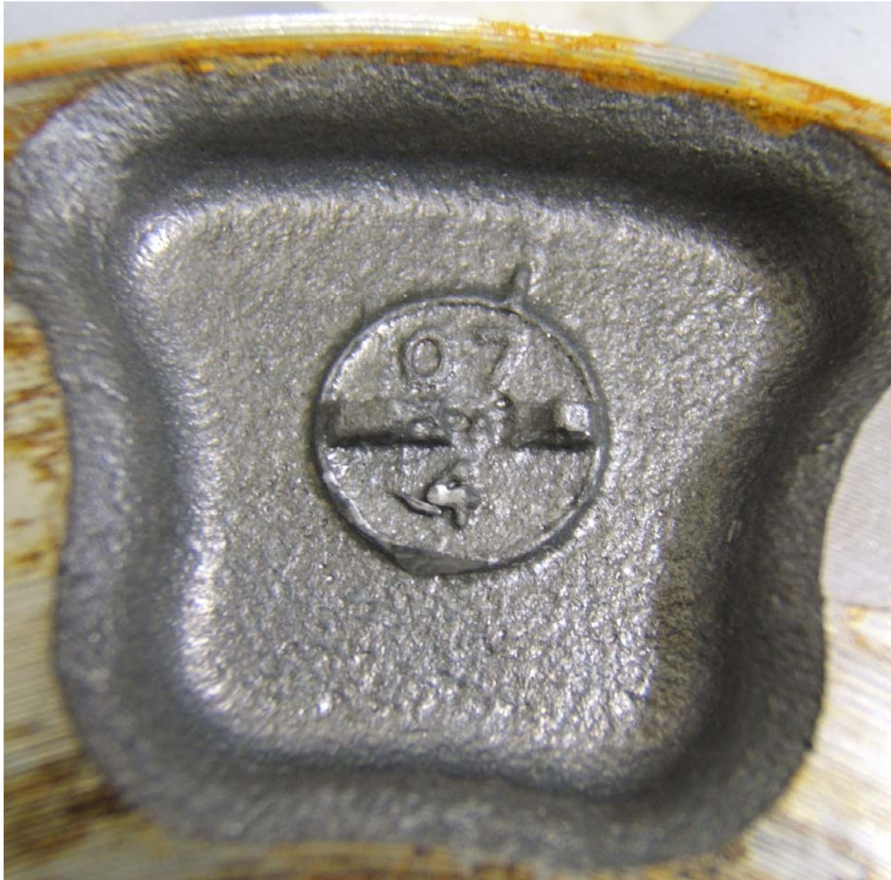
FIGURE 5.13 RIM SHOWING MANUFACTURE DATE
