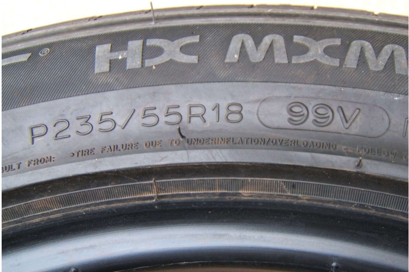
FIGURE 5.7 TIRE SHOWING SIZE, LOAD INDEX, AND SPEED SYMBOL
