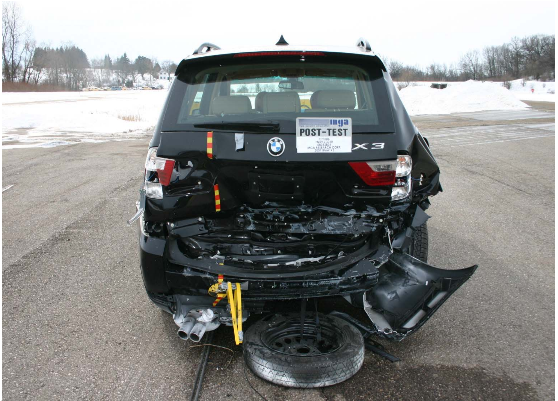
Post-Test Rear View of Vehicle
