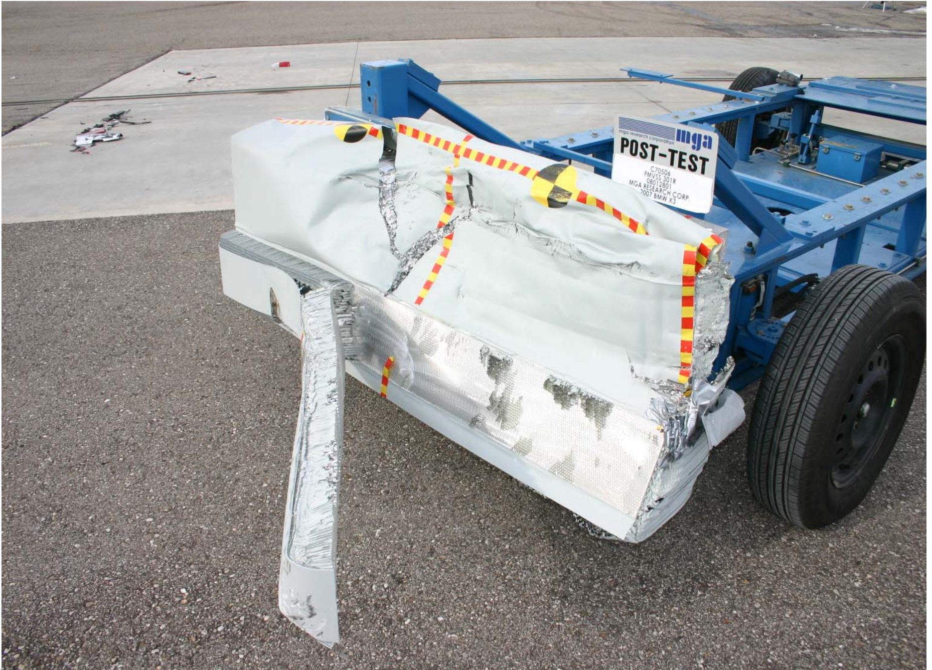
Post-Test \frac{3}{4} Left Side View of MDB
