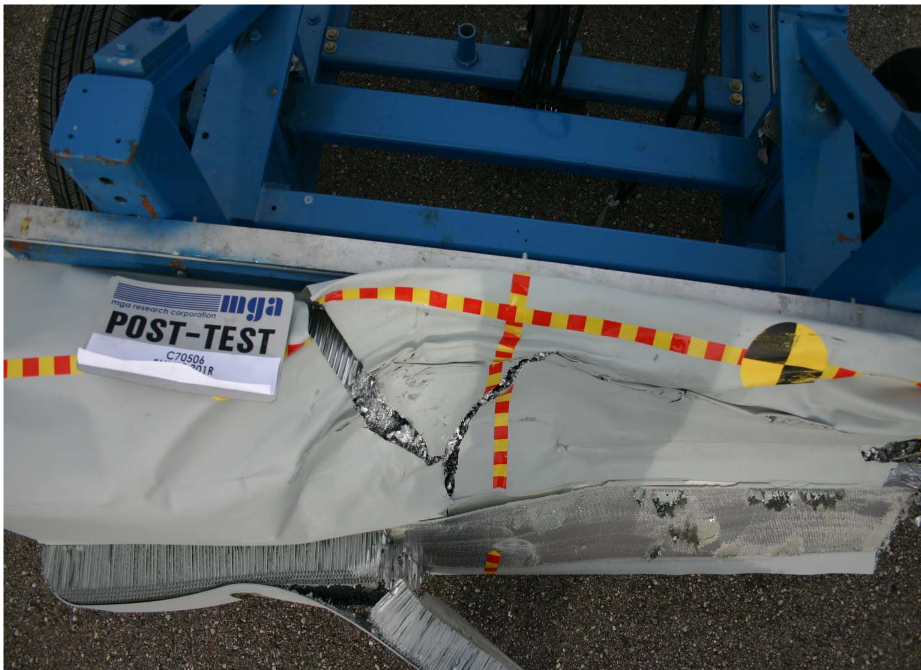
Post-Test Top View of MDB
