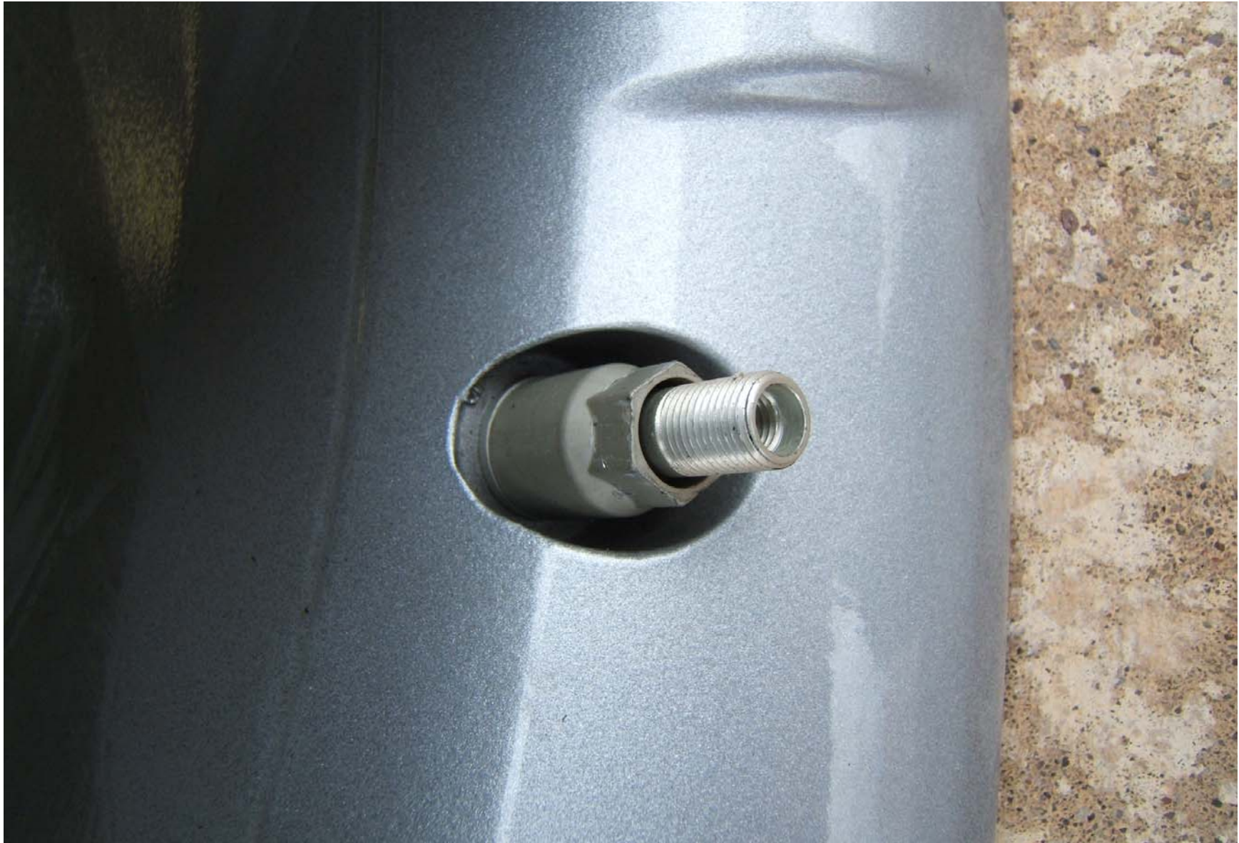
FIGURE 5.10 RIM SHOWING VALVE STEM
