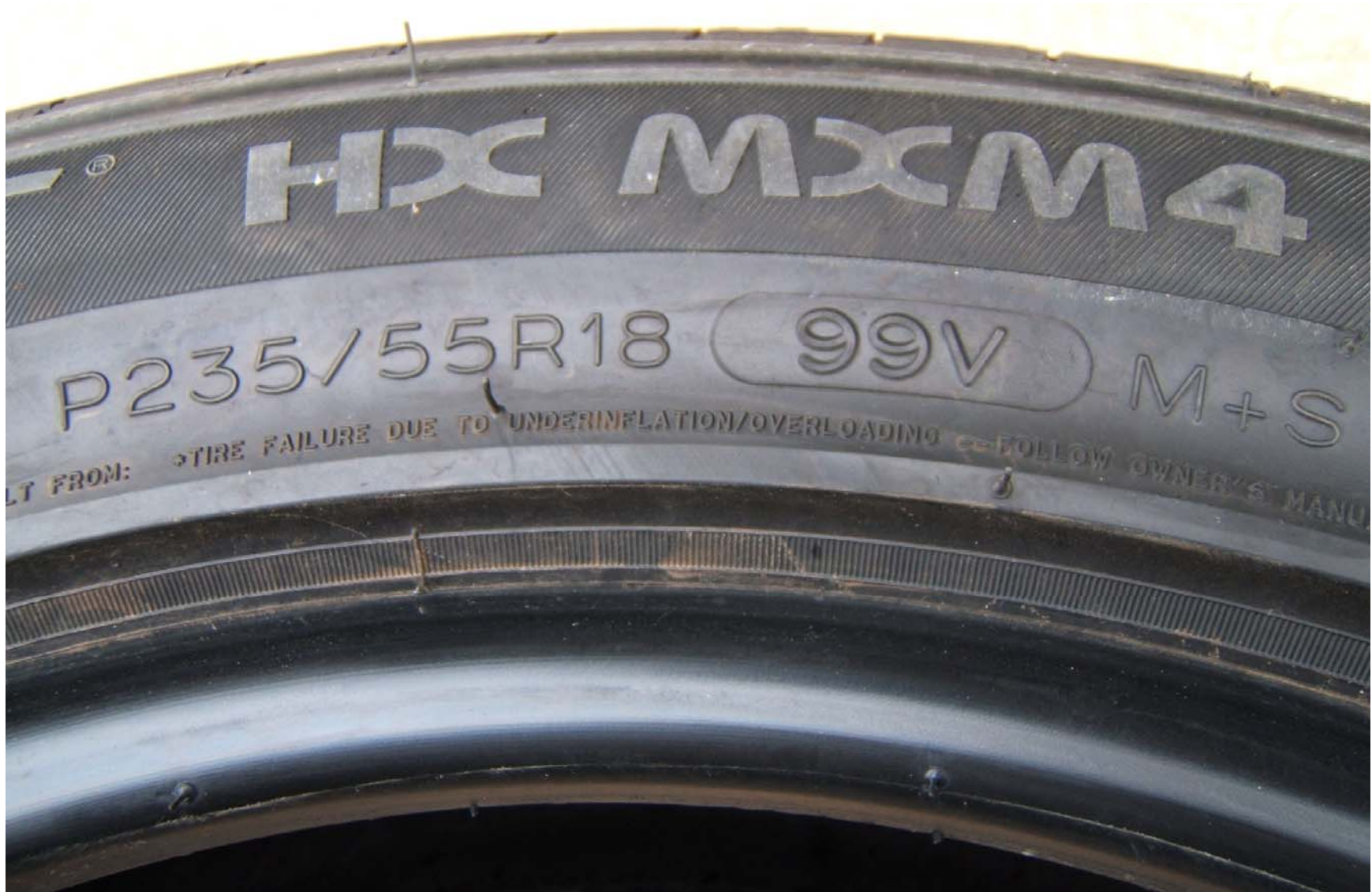
FIGURE 5.6 TIRE SHOWING SIZE, LOAD INDEX, AND SPEED RATING
