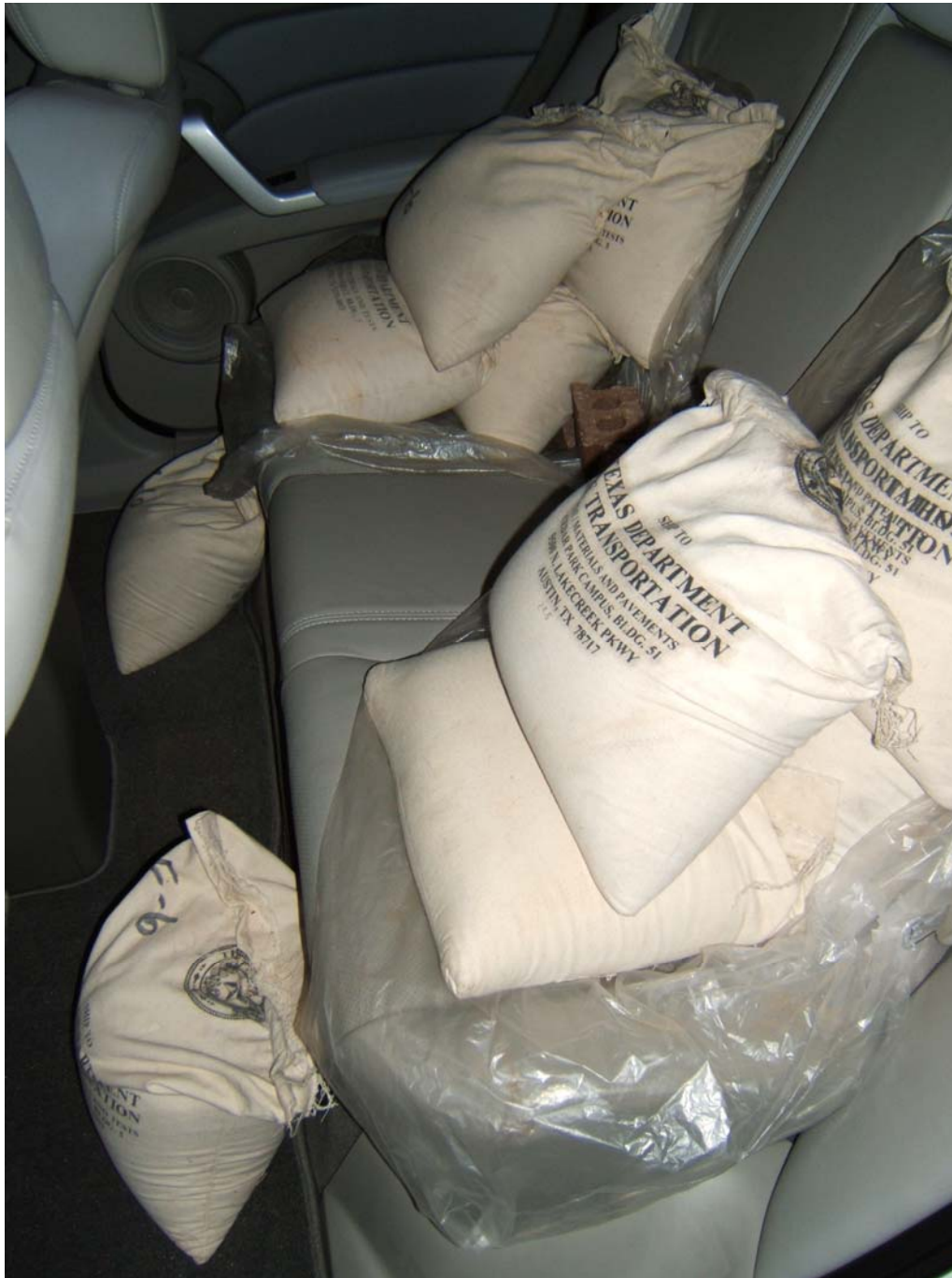
FIGURE 5.14 VEHICLE REAR SEAT BALLAST FOR GVWR LOAD
