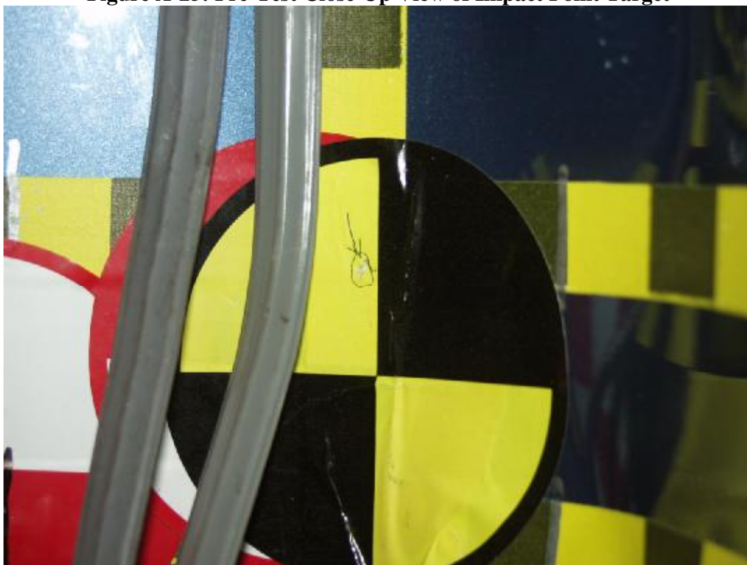
Figure A-26: Post-Test Close-Up View of Impact Point Target (Note: The impact point was moved approximately 22 mm rearward of initial pre-test Target location)
