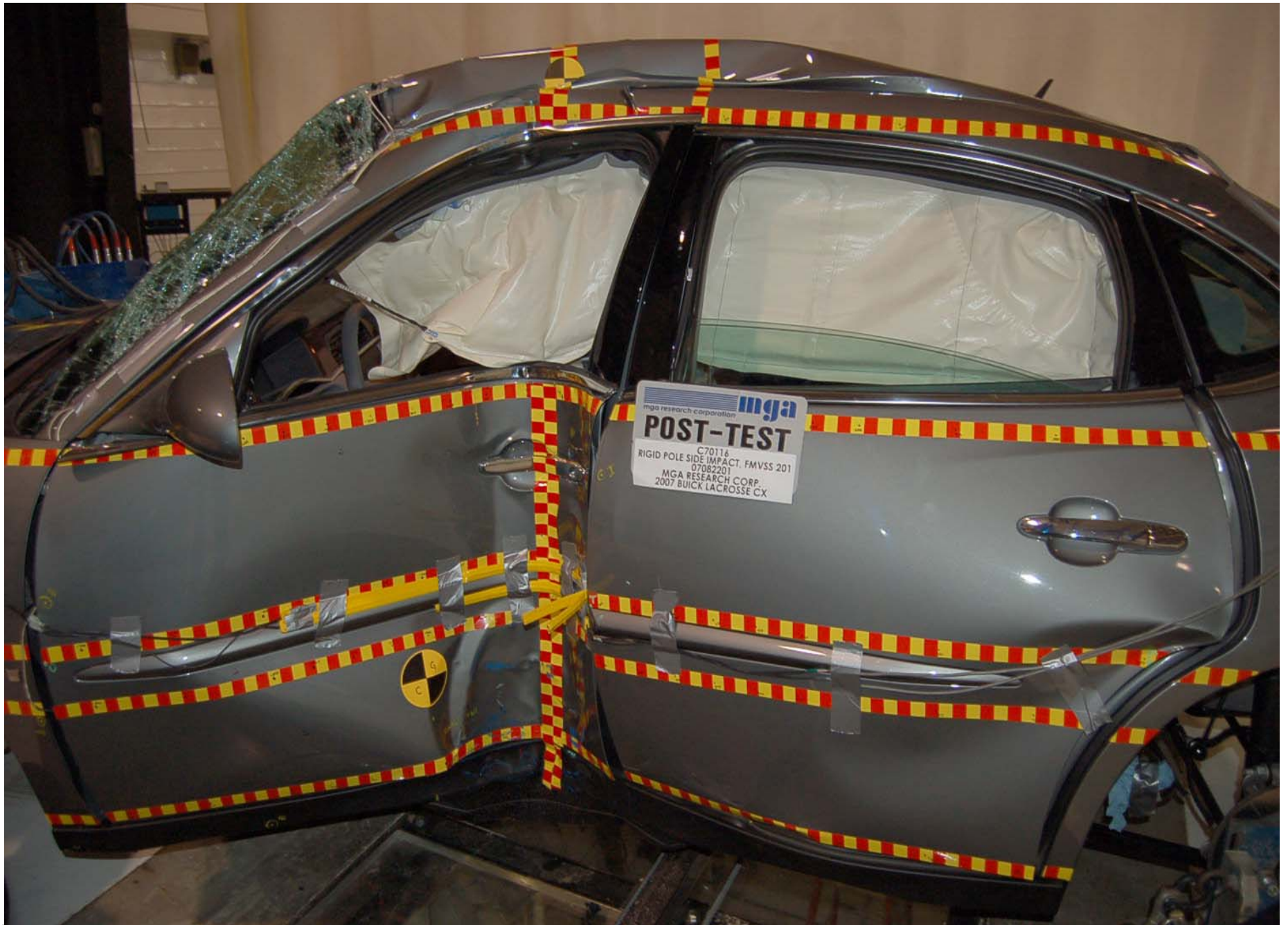
Post-Test Impact Zone Close-up View
