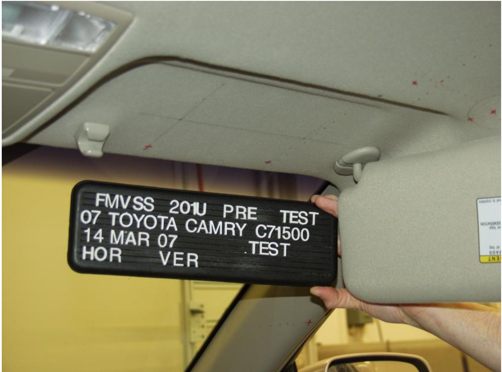
Figure A-13 : PRE-TEST PASSENGER SIDE FRONT HEADER
