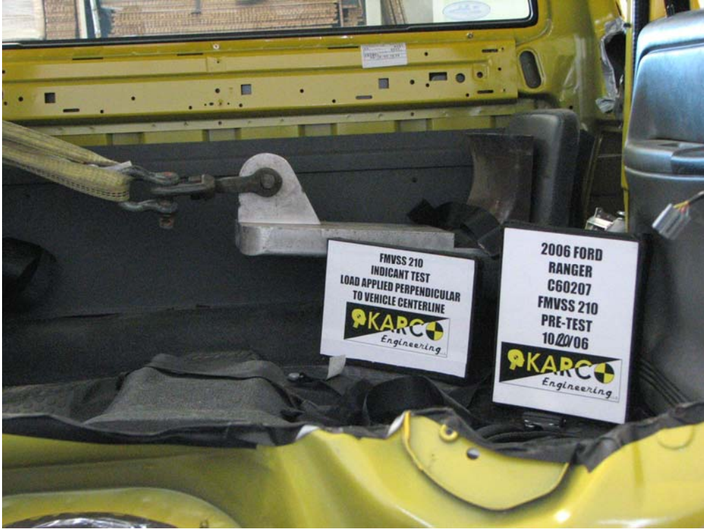
FIGURE 13. Load Applied Perpendicular, P4, Pre-Test
