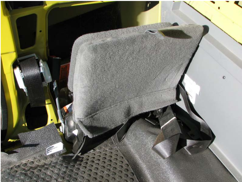
FIGURE 16. Floor Pan Anchors, P3 Overall, Post-Test
