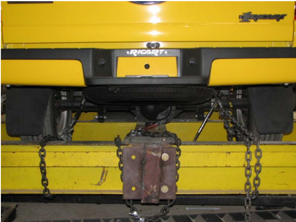
FIGURE 10. Vehicle Mounted in Test Fixture
