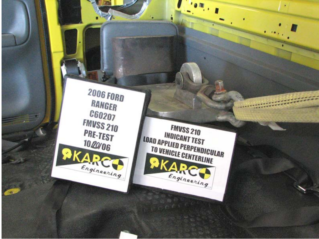
FIGURE 11. Load Applied Perpendicular, P3, Pre-Test
