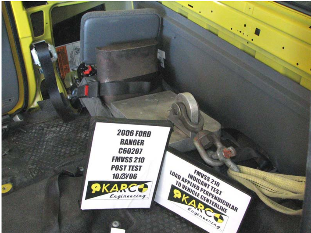
FIGURE 12. Load Applied Perpendicular, P3, Post-Test
