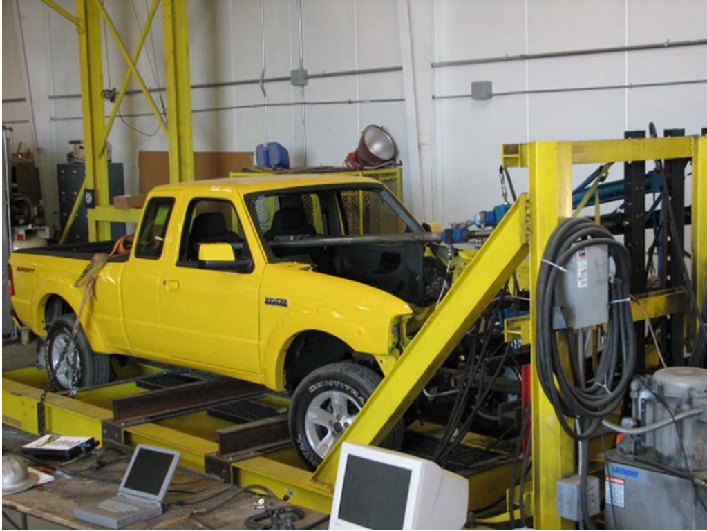
FIGURE 7. Vehicle Mounted in Test Fixture
