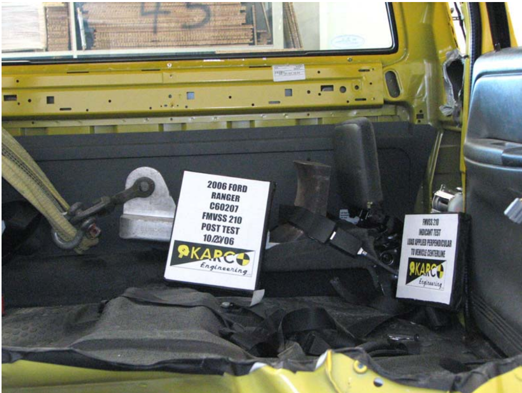
FIGURE 14. Load Applied Perpendicular, P4, Post-Test
