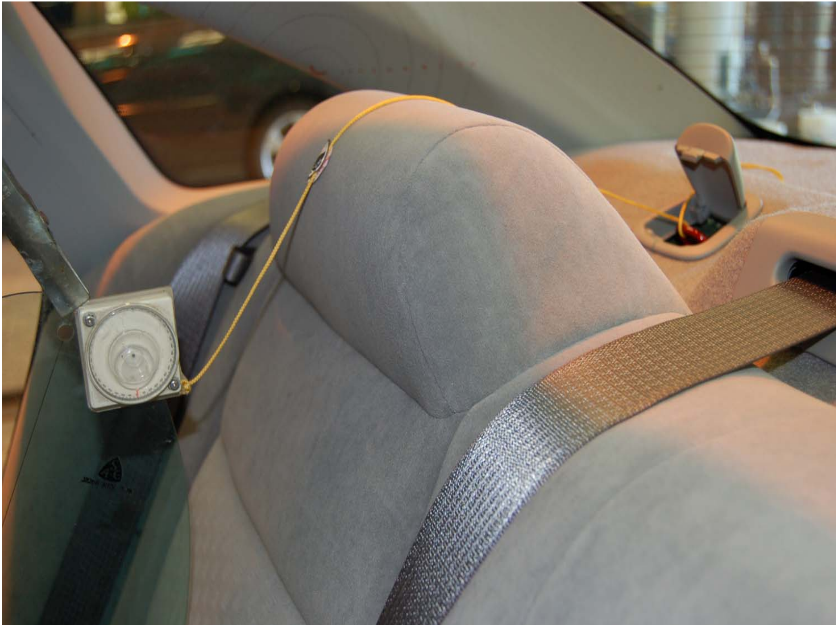
FIGURE 5.18 ROW 2, RIGHT SIDE TOP TETHER ROUTING
