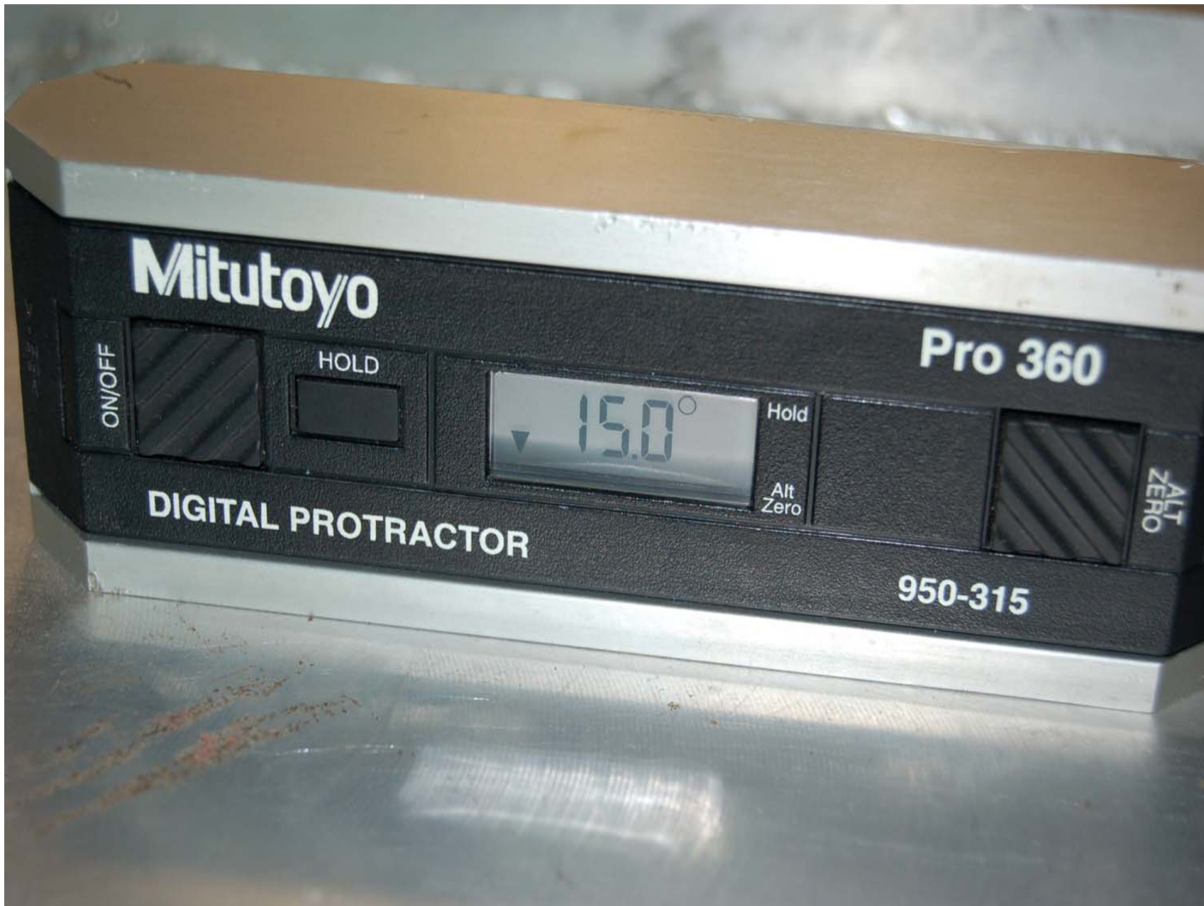
FIGURE 5.31 ROW 2, CENTER CRF PITCH MEASUREMENT
