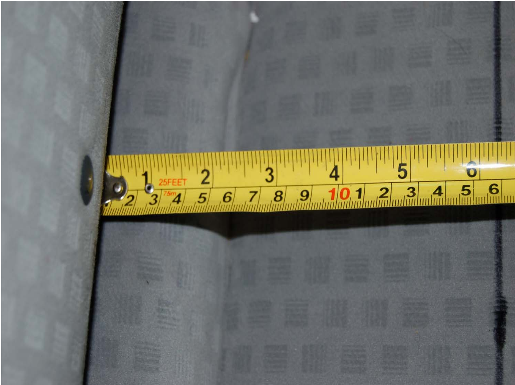
FIGURE 5.32 ROW 2, LEFT SIDE OUTBOARD SRP MEASUREMENT
