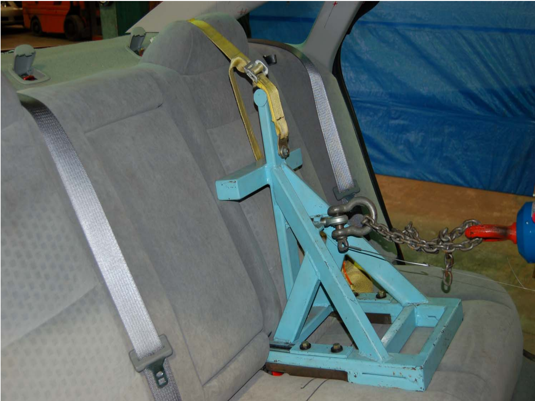
FIGURE 5.41 POST TEST ROW 2, LEFT SIDE WITH SFAD 2
