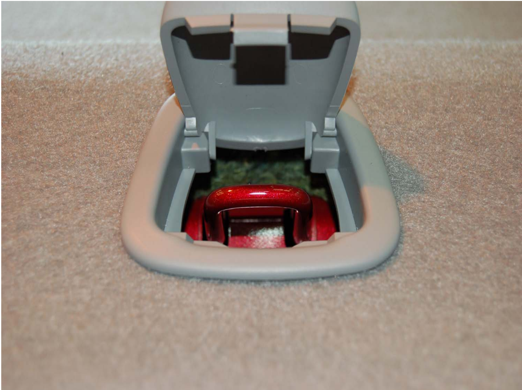
FIGURE 5.8 ROW 2, LEFT SIDE, TOP TETHER ANCHOR, PRE-TEST
