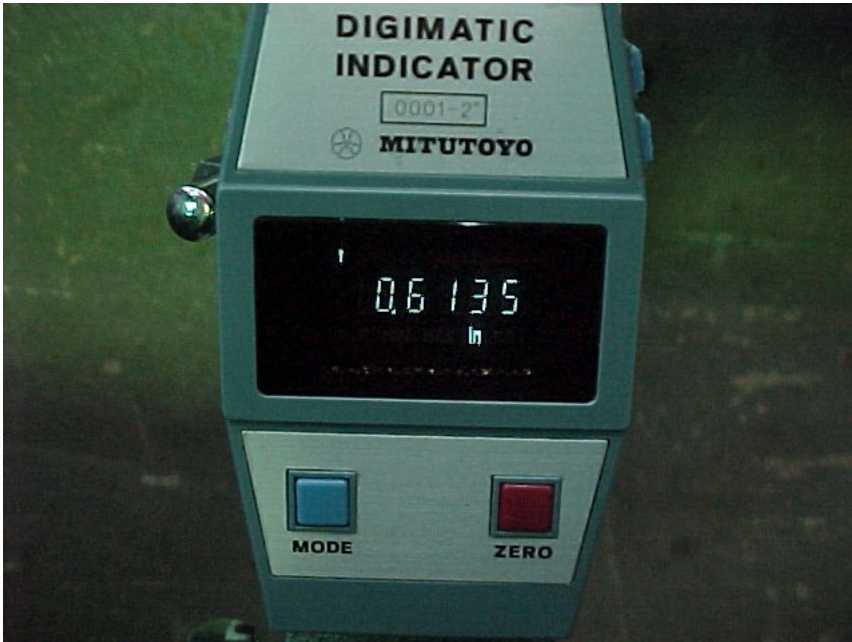
FIGURE 5.15 DIAL INDICATOR AT MAX LOAD – TEST 1
