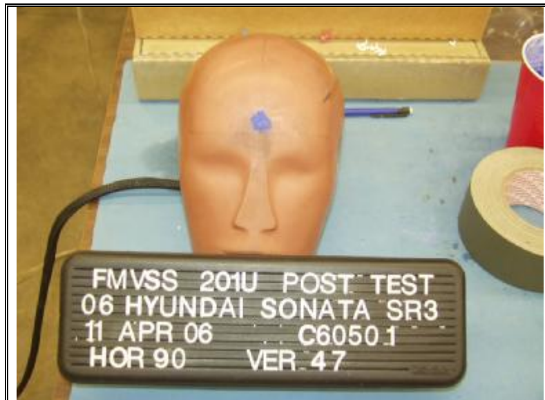
POST-IMPACT SR3F HEADFORM (Placard Date Mislabeled – 10 Apr 06)
