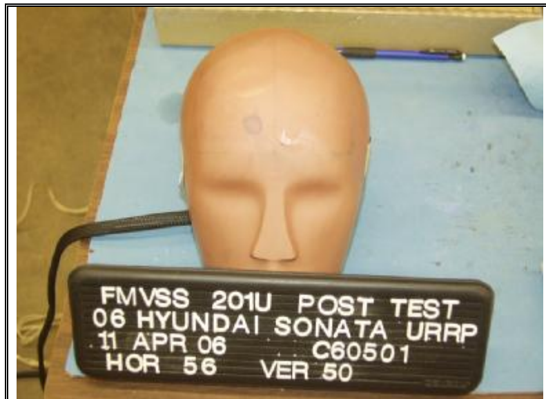
POST-IMPACT URRP HEADFORM (Placard Date Mislabeled – 10 Apr 06)
