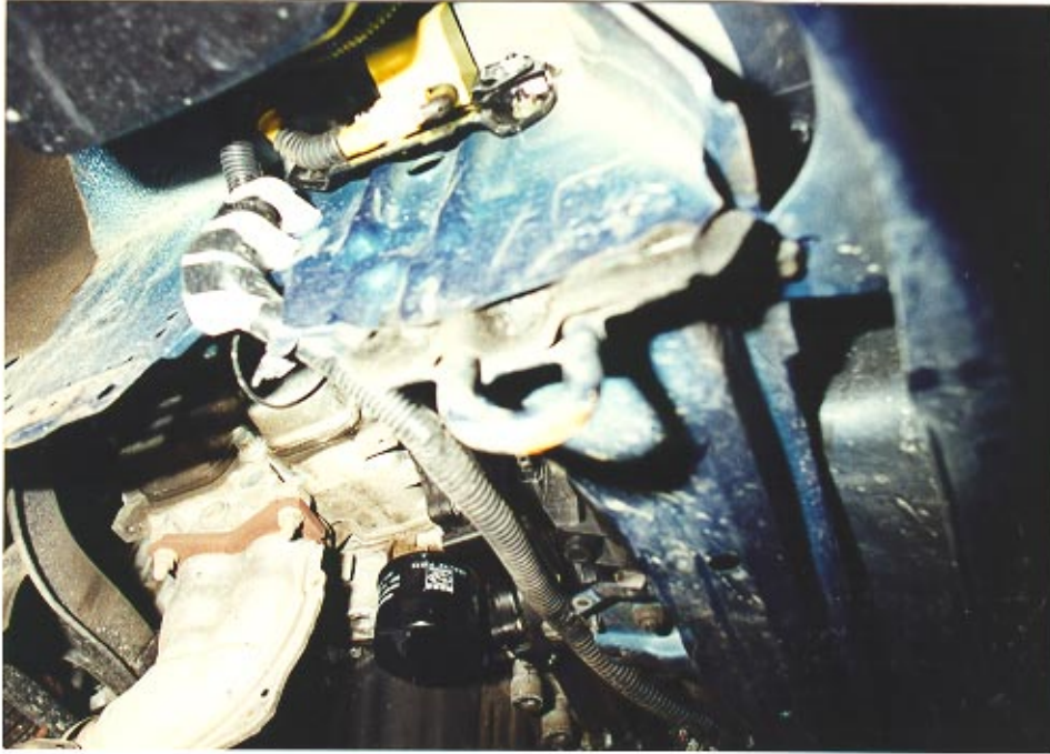
13. Vehicle structure above the tie-down; no residual deformation.
