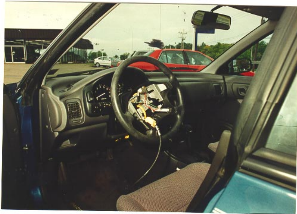
30. Overall view of the steering assembly with the air bag module removed.
