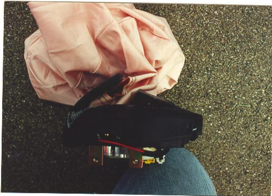
34. Profile view of the symmetrical module cover flaps.
