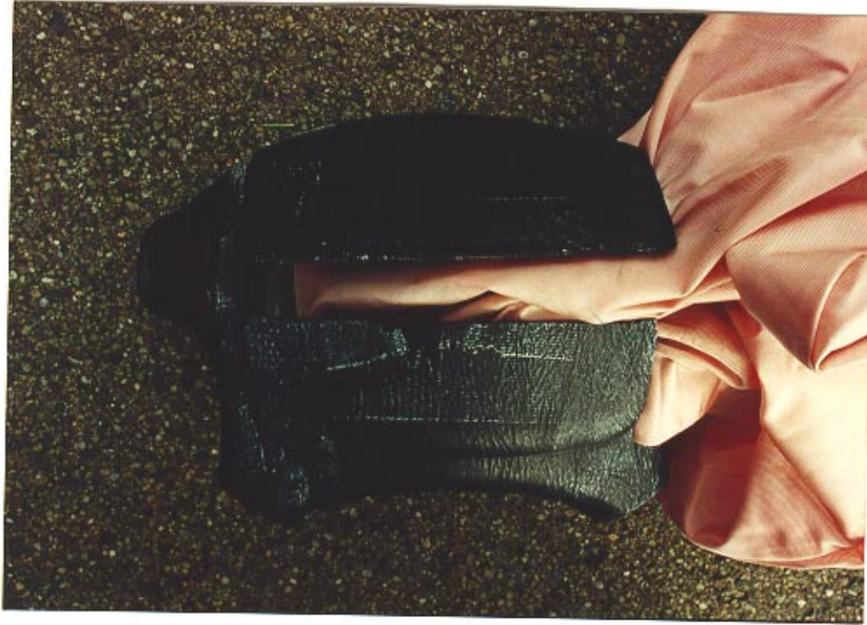
33. Driver's side air bag module cover flaps.
