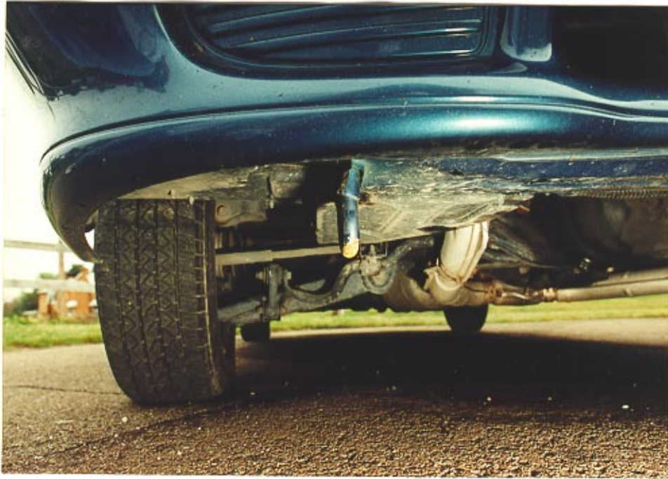
9. Contact damage to the right tie-down bracket.
