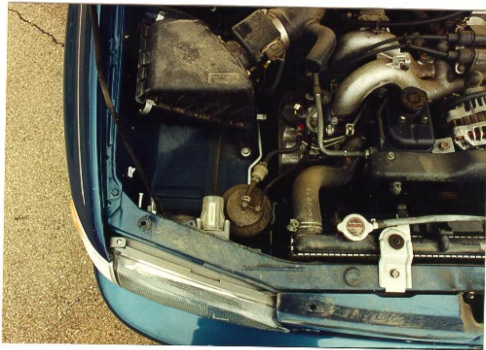
21. & 22. Undeformed areas of the front mounted crash sensors.
