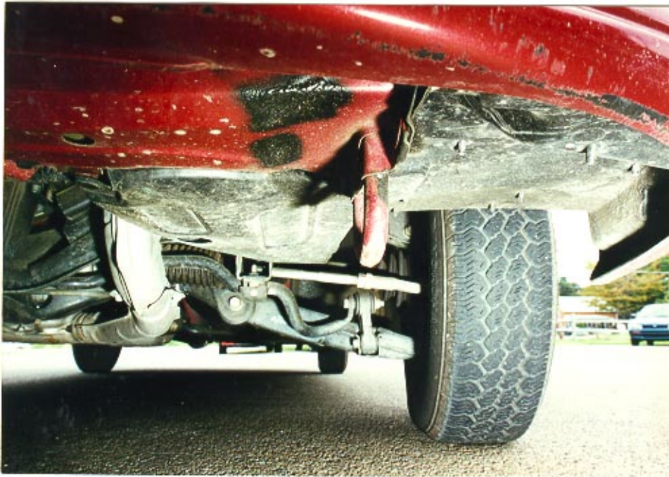
24. Similar contact to the left tie-down bracket of the exemplar vehicle. This contact did not result in air bag deployment.
