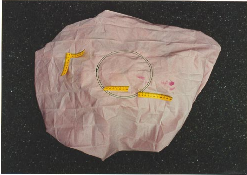
29. Driver's lipstick and makeup transfer on air bag.
