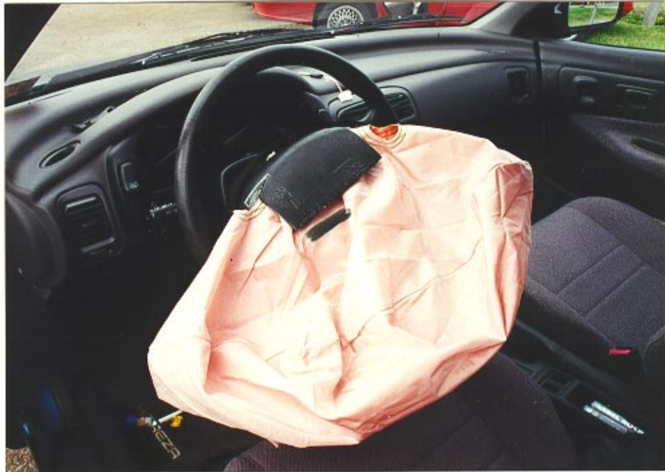
25. Overall view of the deployed driver's side air bag.
