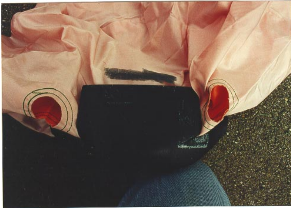
37. Identification labels affixed to the backside of the gas generator.
