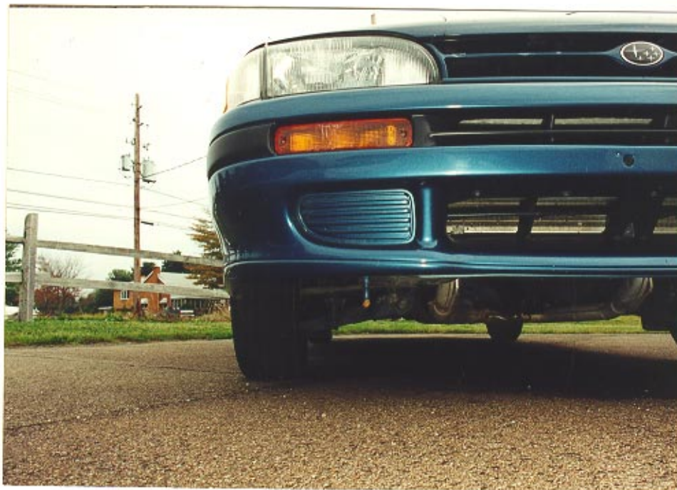
8. Location and exposure of the right tie-down bracket.
