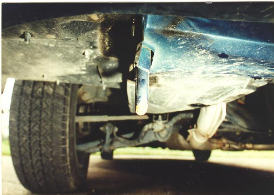
10. Close-up view of the contact damage.
