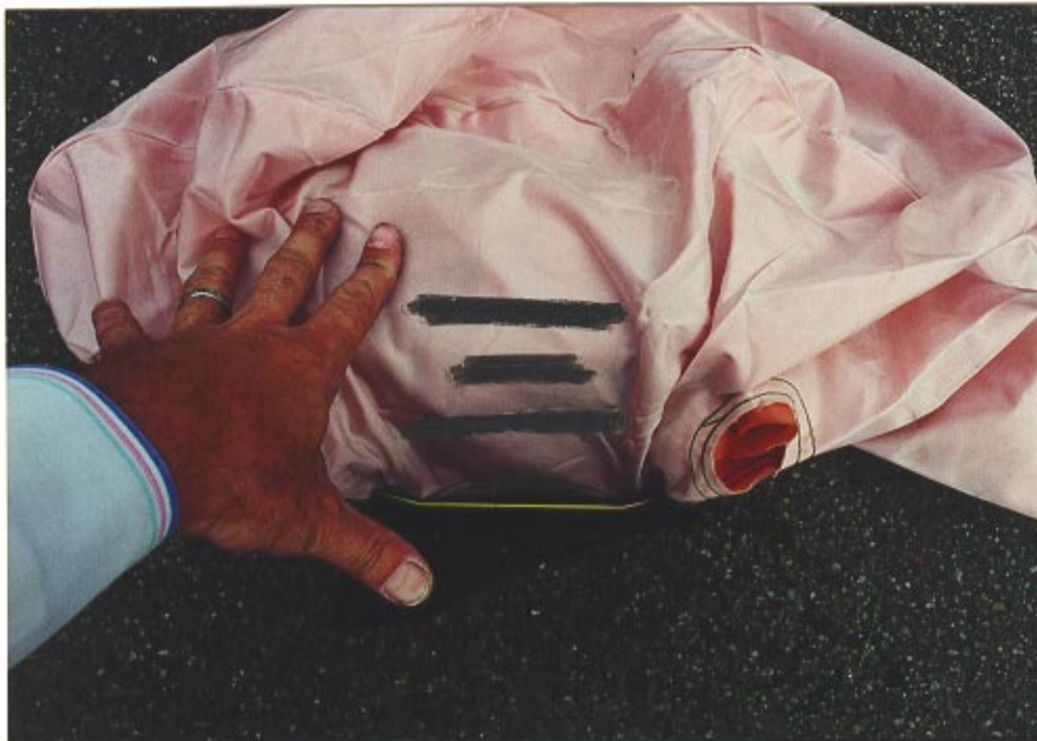
35. Air bag identification numbers stamped onto bag between vent ports.
