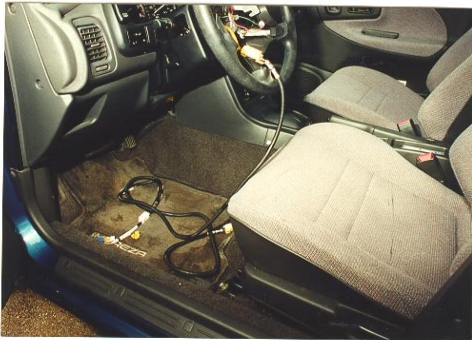
32. Test Harness C used for testing of on board diagnostics of air bag system.
