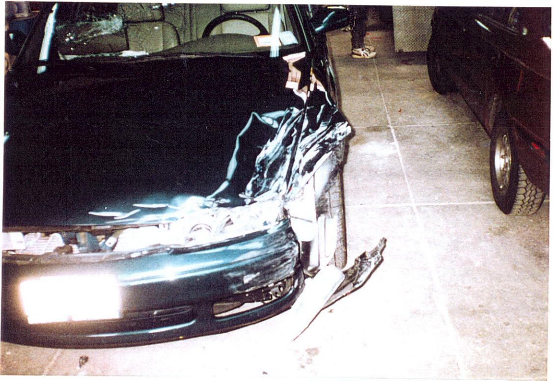
1. Damage to the front and left side plane of the 1994 Mazda 626 (Vehicle #1).
