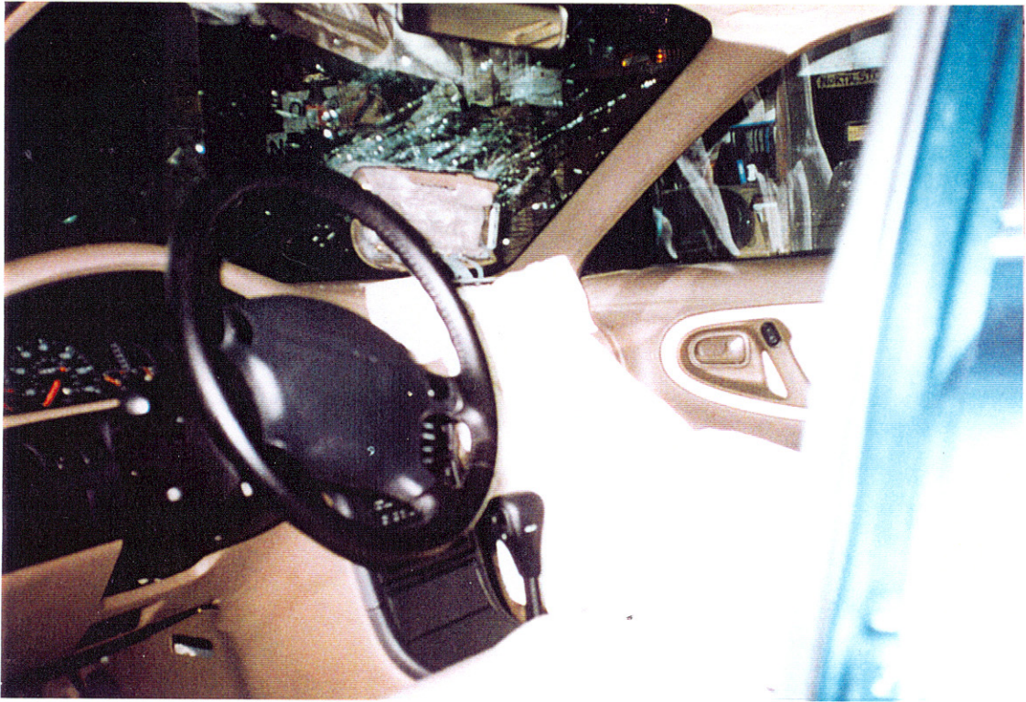
3. Lateral view of the undeployed driver's side air bag and the deployed passenger side air bag.
